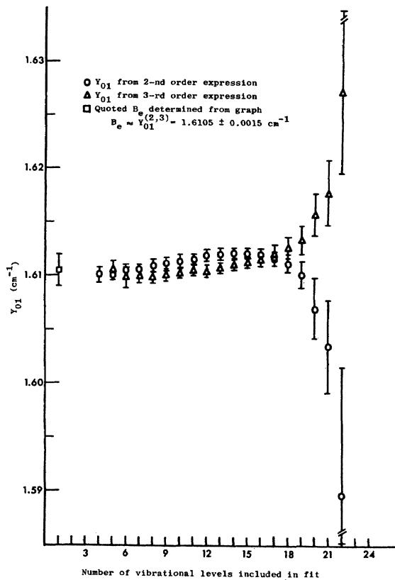
FIGURE 1. Graphical display of  $\gamma_{01}$ -values for the  $A^1\Pi$  state from least squares fits of the  $B_v$ -values to 2d and 3d order expressions as a function of the number of  $B_v$ -values included in the fit.
