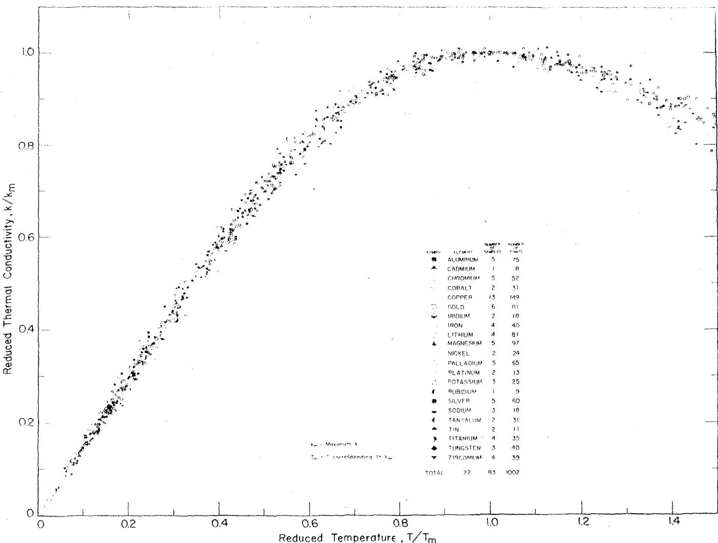
FIGURE 1. REDUCED THERMAL CONDUCTIVITY AS A FUNCTION OF REDUCED TEMPERATURE FOR TWENTY-TWO METALS AT CRYOGENIC TEMPERATURES
