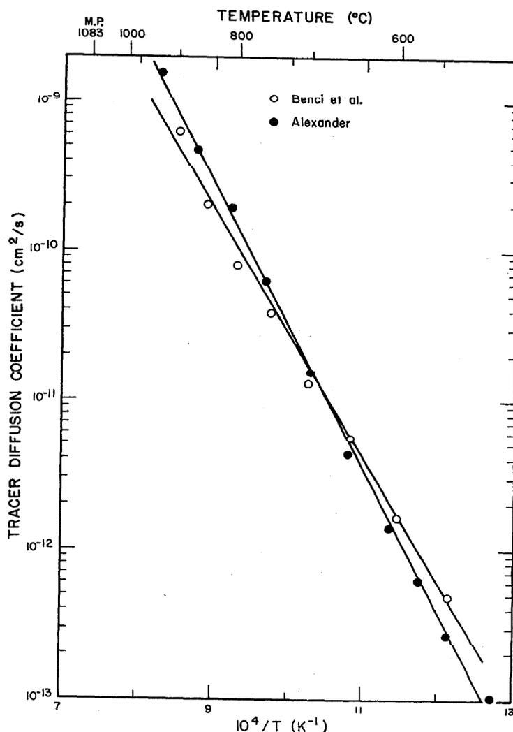
FIGURE 34. The tracer diffusion coefficient of Au-195 in the disordered alloy Cu<sub>3</sub>Au as a function of reciprocal absolute temperature.
