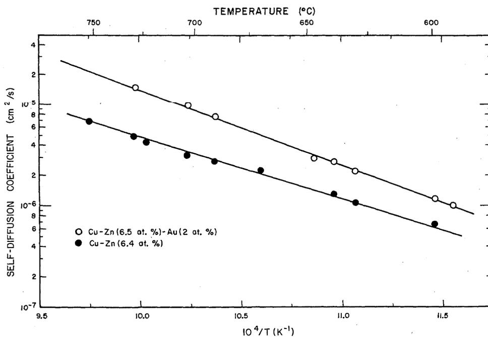
FIGURE 47. The apparent self-diffusion coefficient of zinc in a copper-zinc (6.5 at. %) - gold (2 at. %) alloy as a function of reciprocal absolute temperature.
