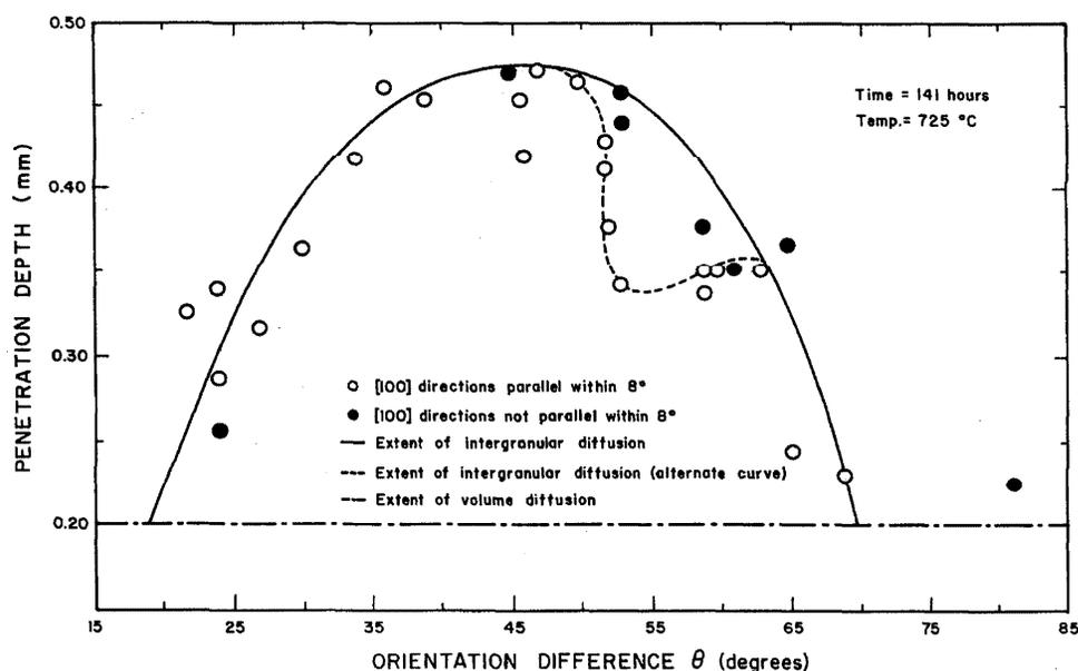
FIGURE 21. Grain boundary penetration of silver as a function of orientation difference ( $\theta$ ) of two columnar grains of copper after 141 hours of diffusion annealing at 725 °C.
