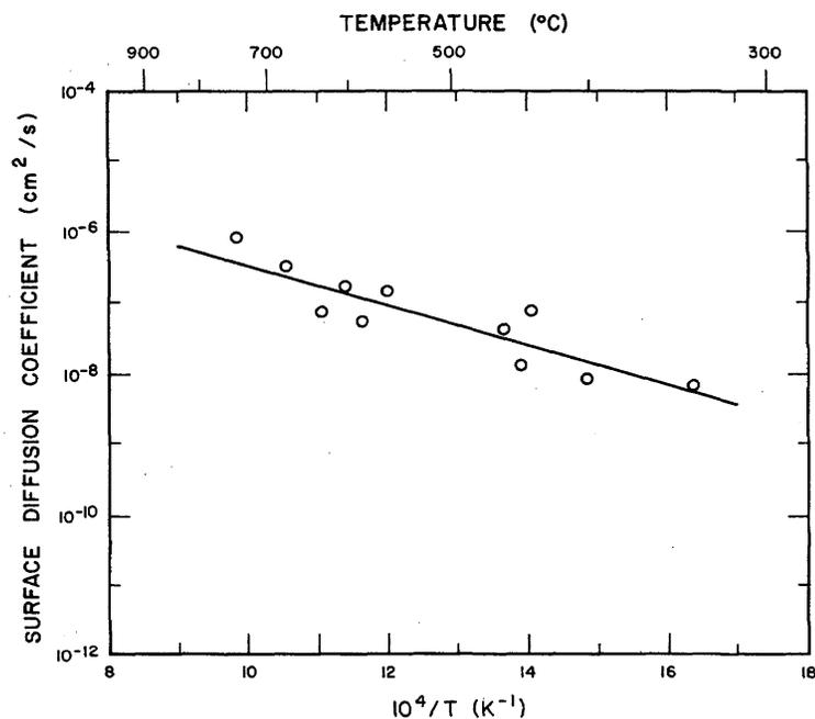
FIGURE 29. The "apparent surface diffusion coefficients" of copper on a silver surface as a function of reciprocal absolute temperature.
