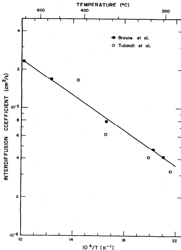
FIGURE 16. Average interdiffusion coefficients for the interdiffusion of copper in silver sulfide (Ag<sub>2</sub>S) as a function of reciprocal absolute temperature.
