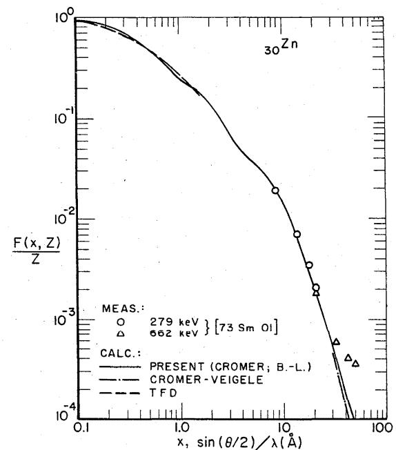
FIGURE 21. Comparison of Thomas-Fermi-Dirac (TFD) (from ref. [6], table 3.3.1B) and present (Cromer [10], [20] for  $x \leq 10 \text{ \AA}^{-1}$ , Bethe-Levinger for  $x > 10 \text{ \AA}^{-1}$ ) tabulated  $F(x, Z)$  values for Zn, also the high- $x$  Cromer-Veigle [12], [20] values, with available measurements.
