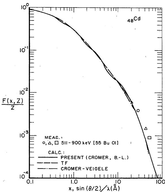
FIGURE 28. Comparison of Thomas-Fermi (TF) and present (Cromer [10], [20] for  $x \leq 10 \text{ \AA}^{-1}$ , Bethe-Levinger [29] for  $x > 10 \text{ \AA}^{-1}$ ) tabulated  $F(x, Z)$  values for Cd, also the high- $x$  Cromer-Veigle [12], [20] values, with available measurements.
