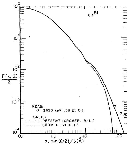
FIGURE 40. Comparison of present (Cromer [10], [20] for  $x \leq 10 \text{ \AA}^{-1}$ , Bethe-Levinger for  $x > 10 \text{ \AA}^{-1}$ ) tabulated  $F(x, Z)$  values for Bi, also the high- $x$  Cromer-Veigle [12], [20] values, with available measurements.
