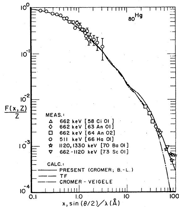
FIGURE 38. Comparison of Thomas-Fermi (TF) and present (Cromer [10], [20] for  $x \leq 10 \text{ \AA}^{-1}$ , Bethe-Levinger [29] for  $x > 10 \text{ \AA}^{-1}$ ) tabulated  $F(x, Z)$  values for Hg, also the high- $x$  Cromer-Veigele [12], [20] values, with available measurements.
