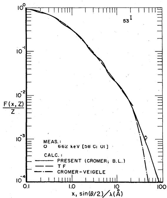
FIGURE 31. Comparison of Thomas-Fermi (TF) and present (Cromer [10], [20] for  $x \leq 10 \text{ \AA}^{-1}$ , Bethe-Levinger [29] for  $x > 10 \text{ \AA}^{-1}$ ) tabulated  $F(x, Z)$  values for I, also the high- $x$  Cromer-Veigle [12], [20] values, with available measurements.
