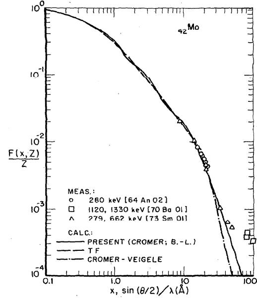
FIGURE 25. Comparison of Thomas-Fermi (TF) and present (Cromer [10], [20] for  $x \leq 10 \text{ \AA}^{-1}$ , Bethe-Levinger [29] for  $x > 10 \text{ \AA}^{-1}$ ) tabulated  $F(x, Z)$  values for Mo, also the high- $x$  Cromer-Veigle [12], [20] values, with available measurements.
