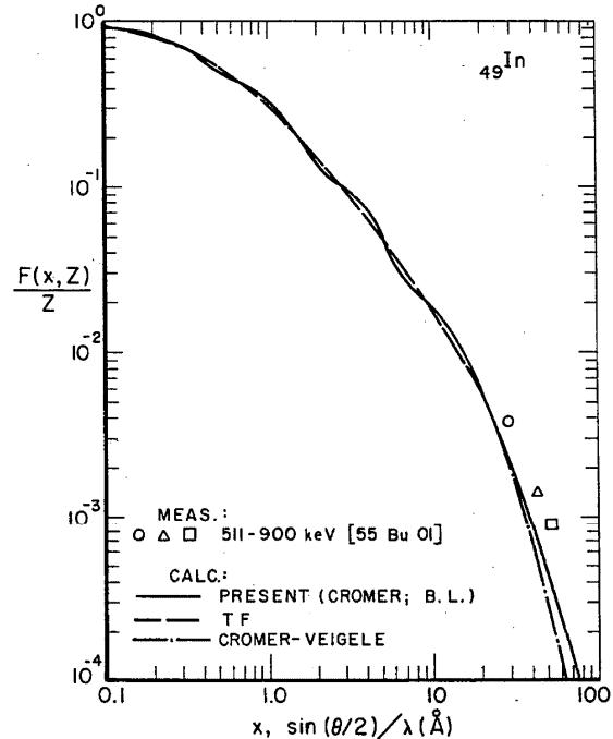
FIGURE 29. Comparison of Thomas-Fermi (TF) and present (Cromer [10], [20] for  $x \leq 10 \text{ \AA}^{-1}$ , Bethe-Levinger [29] for  $x > 10 \text{ \AA}^{-1}$ ) tabulated  $F(x, Z)$  values for In, also the high- $x$  Cromer-Veigle [12], [20] values, with available measurements.
