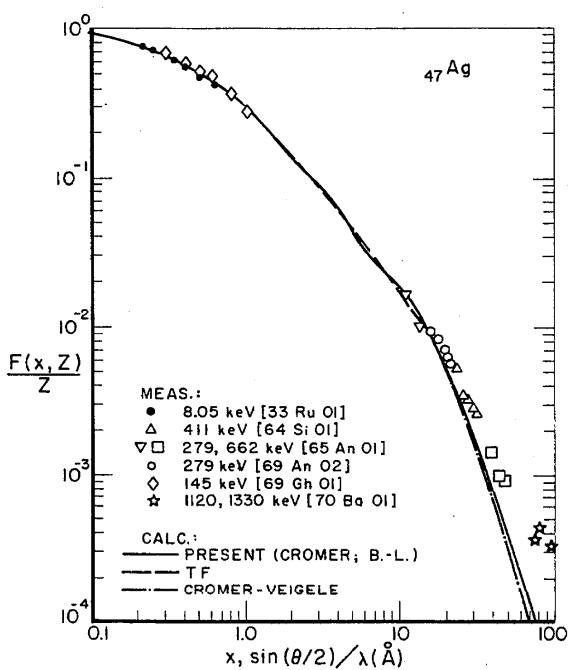
FIGURE 27. Comparison of Thomas-Fermi (TF) and present (Cromer [10], [20] for  $x \leq 10 \text{ \AA}^{-1}$ , Bethe-Levinger [29] for  $x > 10 \text{ \AA}^{-1}$ ) tabulated  $F(x, Z)$  values for Ag, also the high- $x$  Cromer-Veigle [12], [20] values, with available measurements.
