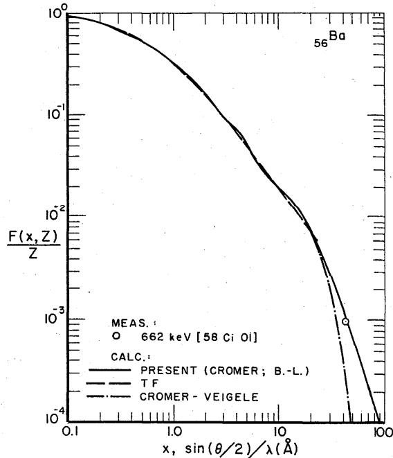
FIGURE 32. Comparison of Thomas-Fermi (TF) and present (Cromer [10], [20] for  $x \leq 10 \text{ \AA}^{-1}$ , Bethe-Levinger [29] for  $x > 10 \text{ \AA}^{-1}$ ) tabulated  $F(x, Z)$  values for Ba, also the high- $x$  Cromer-Veigle [12], [20] values, with available measurements.
