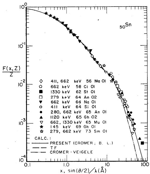
FIGURE 30. Comparison of Thomas-Fermi (TF) and present (Cromer [10], [20] for  $x \leq 10 \text{ \AA}^{-1}$ , Bethe-Levinger [29] for  $x > 10 \text{ \AA}^{-1}$ ) tabulated  $F(x, Z)$  values for Sn, also the high- $x$  Cromer-Veigle [12], [20] values, with available measurements.
