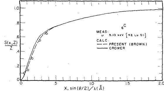
FIGURE 43. Comparison of the Cromer [18], [20] non-relativistic Hartree-Fock and the Brown [56] configuration interaction (present tabulation) calculated  $S(x, Z)$  values for C with the measurement by Laval [42 La 01].
