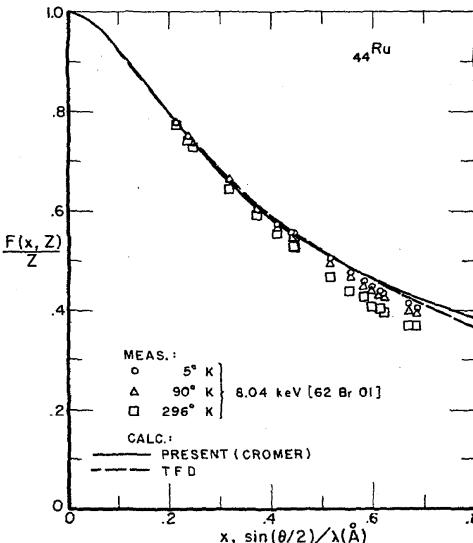
FIGURE 26. Comparison of Thomas-Fermi-Dirac (TFD) and present (Cromer [10], [20] in this  $x$ -range) tabulated  $F(x, Z)$  values for Ru with the Brill and Chopra [62Br 01] measurements of Ru powder showing the effect of thermal motion on the scattering centers.
