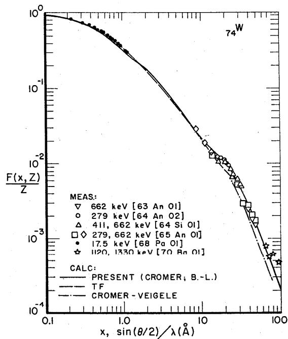
FIGURE 35. Comparison of Thomas-Fermi (TF) and present (Cromer [10], [20] for  $x \leq 10 \text{ \AA}^{-1}$ , Bethe-Levinger [29] for  $x > 10 \text{ \AA}^{-1}$ ) tabulated  $F(x, Z)$  values for W, also the high- $x$  Cromer-Veigele [12], [20] values, with available measurements.
