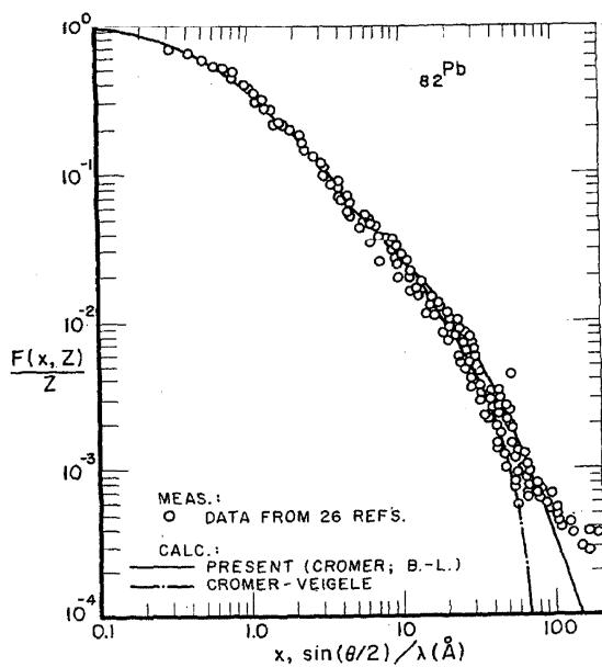
FIGURE 39. Comparison of present (Cromer [10], [20] for  $x \leq 10 \text{ \AA}^{-1}$ , Bethe-Levinger for  $x > 10 \text{ \AA}^{-1}$ ) tabulated  $F(x, Z)$  values for Pb, also the high- $x$  Cromer-Veigle [12], [20] values, with available measurements.
