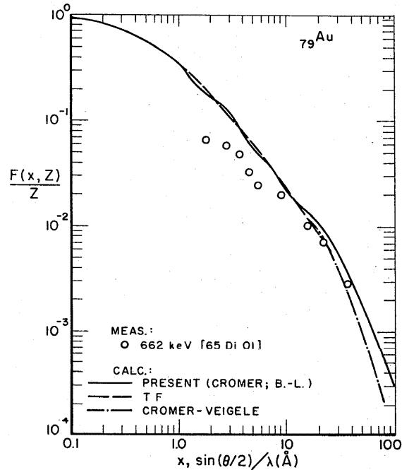
FIGURE 37. Comparison of Thomas-Fermi (TF) and present (Cromer [10], [20] for  $x \leq 10 \text{ \AA}^{-1}$ , Bethe-Levinger [29] for  $x > 10 \text{ \AA}^{-1}$ ) tabulated  $F(x, Z)$  values for Au, also the high- $x$  Cromer-Veigele [12], [20] values, with available measurements.
