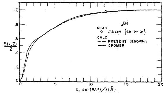
FIGURE 42. Comparison of the Cromer-Mann [17], [20] non-relativistic Hartree-Fock and the Brown [56] configuration-interaction (present tabulation) calculated  $S(x, Z)$  values for Be with the measurement by Phillips and Weiss [68 Ph 01].
