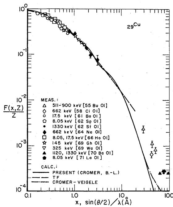
FIGURE 20. Comparison of Thomas-Fermi (TF) and present (Cromer [10], [20] for  $x \leq 10 \text{ \AA}^{-1}$ , Bethe-Levinger [29] for  $x > 10 \text{ \AA}^{-1}$ ) tabulated  $F(x, Z)$  values for Cu, also the high- $x$  Cromer-Veigle [12], [20] values, with available measurements.
