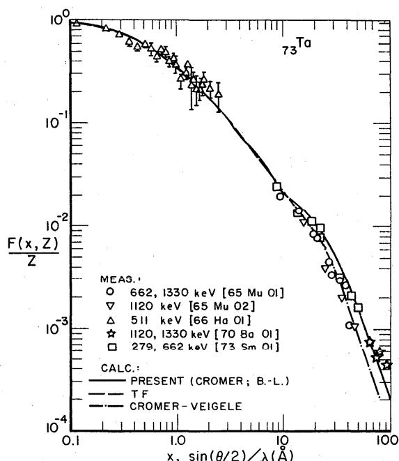
FIGURE 34. Comparison of Thomas-Fermi (TF) and present (Cromer [10], [20] for  $x \leq 10 \text{ \AA}^{-1}$ , Bethe-Levinger [29] for  $x > 10 \text{ \AA}^{-1}$ ) tabulated  $F(x, Z)$  values for Ta, also the high- $x$  Cromer-Veigle [12], [20] values, with available measurements.
