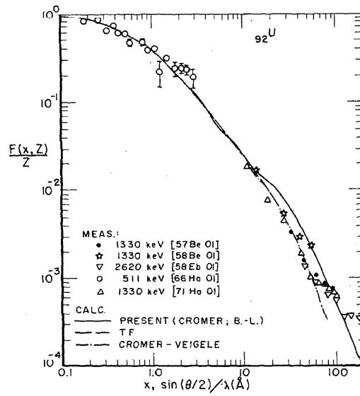
FIGURE 41. Comparison of Thomas-Fermi (TF) and present (Cromer [10], [20] for  $x \leq 10 \text{ \AA}^{-1}$ , Bethe-Levinger [29] for  $x > 10 \text{ \AA}^{-1}$ ) tabulated  $F(x, Z)$  values for U, also the high- $x$  Cromer-Veigle [12], [20] values with available measurements.
