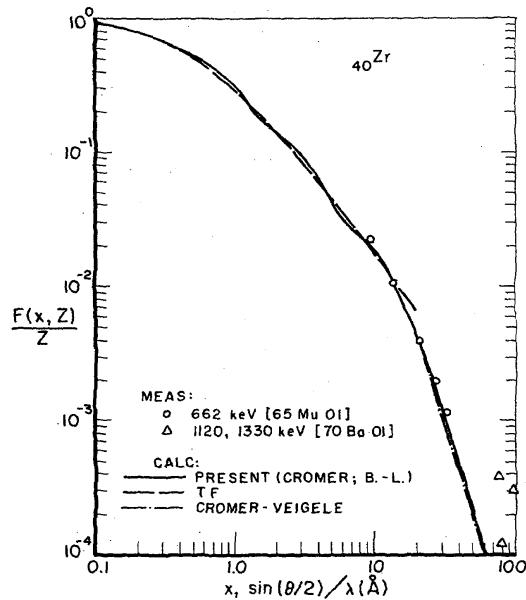
FIGURE 24. Comparison of Thomas-Fermi (TF) and present (Cromer [10], [20] for  $x \leq 10 \text{ \AA}^{-1}$ , Bethe-Levinger [29] for  $x > 10 \text{ \AA}^{-1}$ ) tabulated  $F(x, Z)$  values for Zr, also the high- $x$  Cromer-Veigle [12], [20] values, with available measurements.
