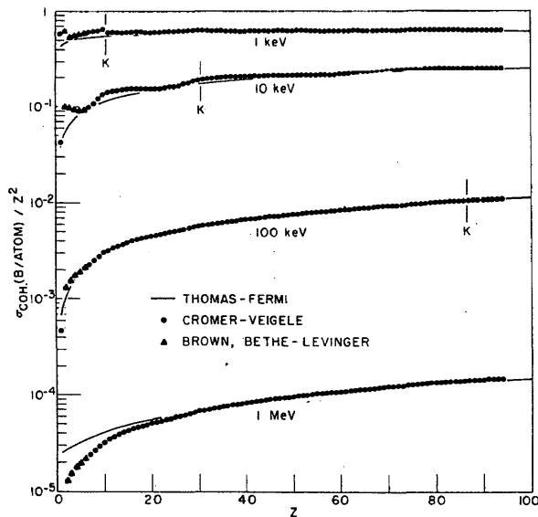
FIGURE 48. Comparison of integrated coherent (Rayleigh) scattering cross sections using  $F(x, Z)$  values from (a) the Thomas-Fermi model (solid curves), (b) the Cromer-Veigle [12], [20] tables (circles) and (c) the configuration-interaction results of Brown [56], [94] (triangles) as a function of  $Z$  for photon energies of 1, 10, 100, and 1000 keV.
