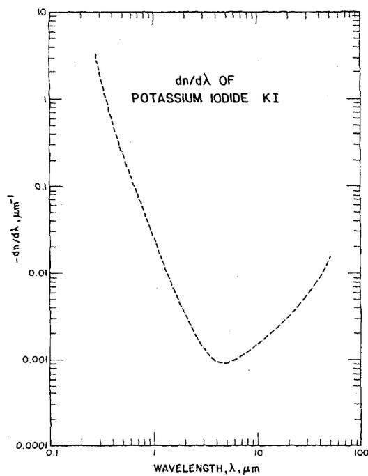
FIGURE 42.  $dn/d\lambda$  of KI
