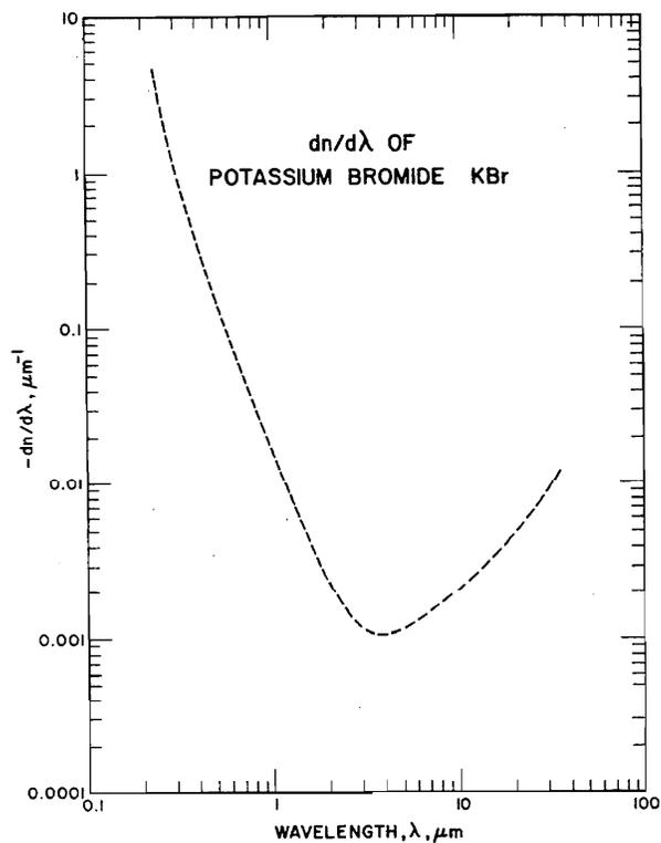
FIGURE 39.  $dn/d\lambda$  of KBr
