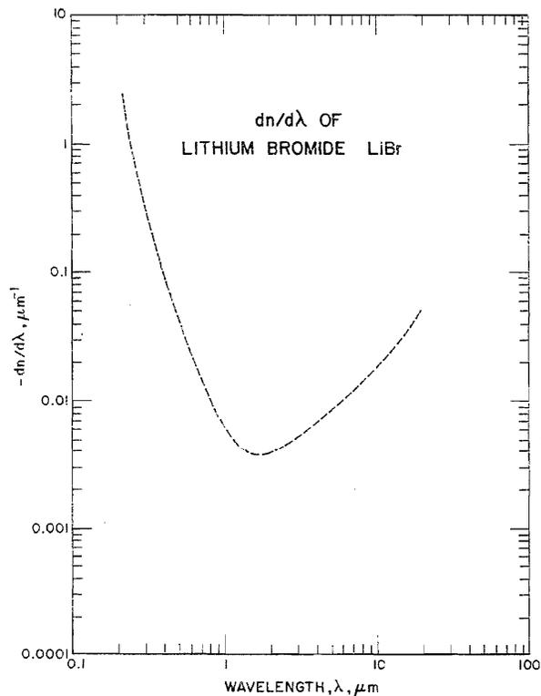
FIGURE 12.  $dn/d\lambda$  of LiBr
