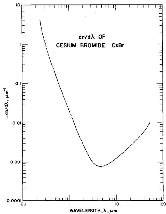
FIGURE 63.  $dn/d\lambda$  of CsBr
