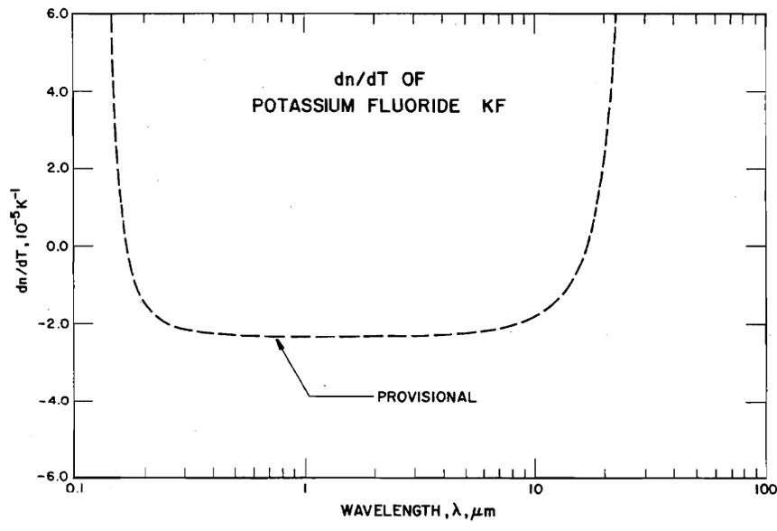
FIGURE 32.  $dn/dT$  of KF
