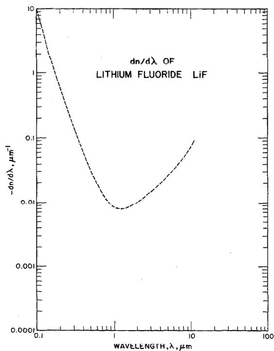
FIGURE 6.  $dn/d\lambda$  of LiF
