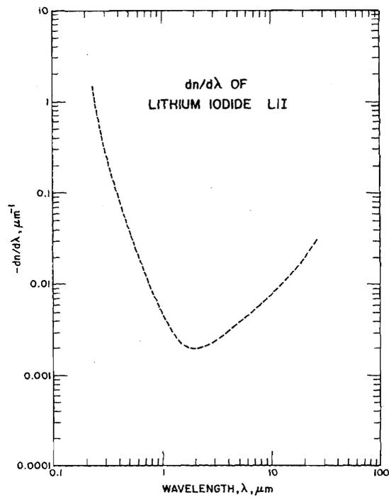
FIGURE 15.  $dn/d\lambda$  of LiI
