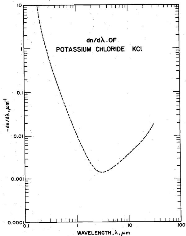
FIGURE 35.  $dn/d\lambda$  of KCl
