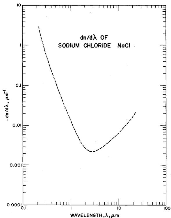
FIGURE 22.  $dn/d\lambda$  of NaCl
