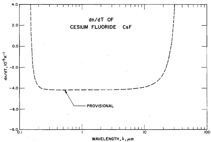
FIGURE 58.  $dn/dT$  of  $\text{CsF}$
