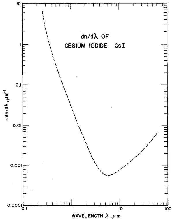
FIGURE 66.  $dn/d\lambda$  of CsI
