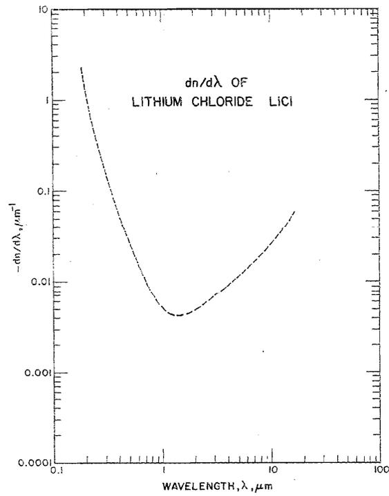
FIGURE 9.  $dn/d\lambda$  of LiCl
