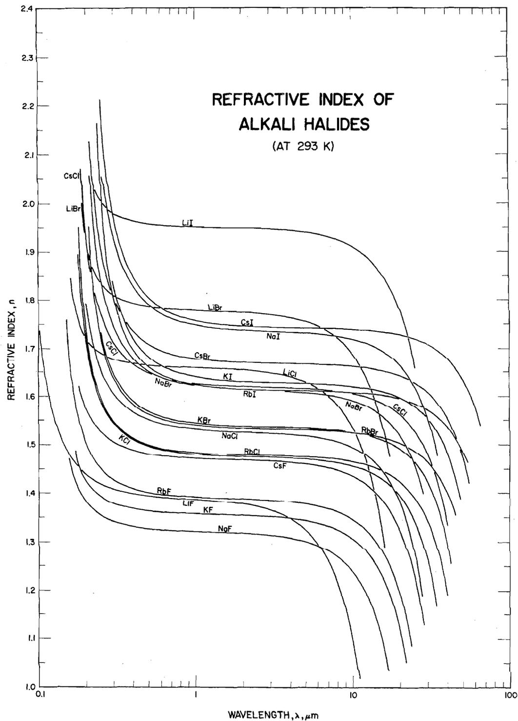
FIGURE 68. Refractive Index of Alkali Halides at 293 K
