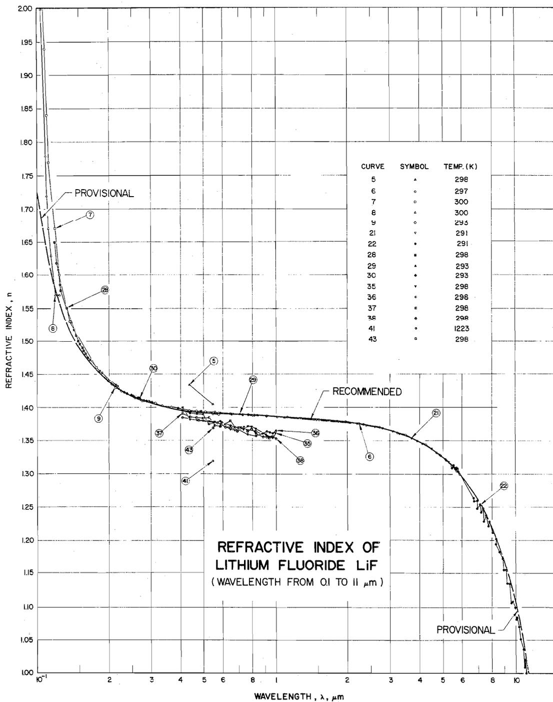
FIGURE 4. Refractive Index of LiF (transparent region)
