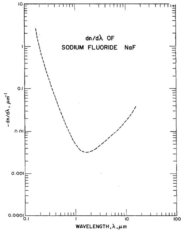
FIGURE 18.  $dn/d\lambda$  of NaF
