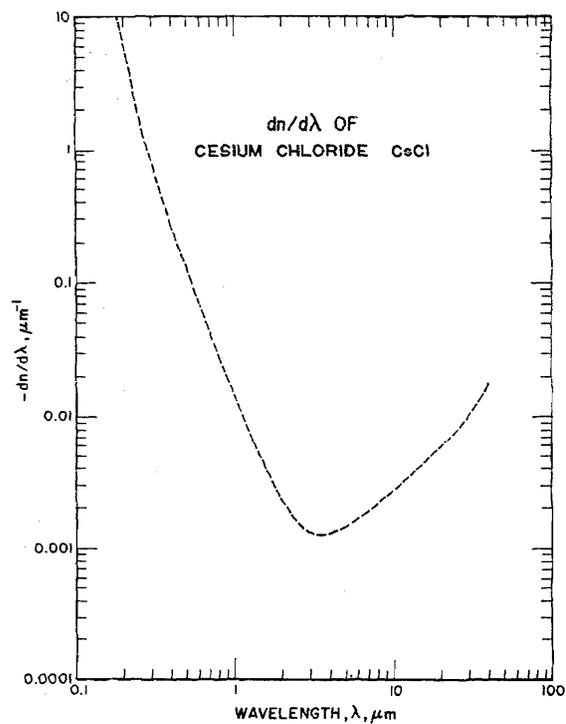
FIGURE 60.  $dn/d\lambda$  of CsCl
