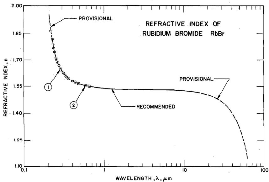
FIGURE 50. Refractive Index of RbBr
