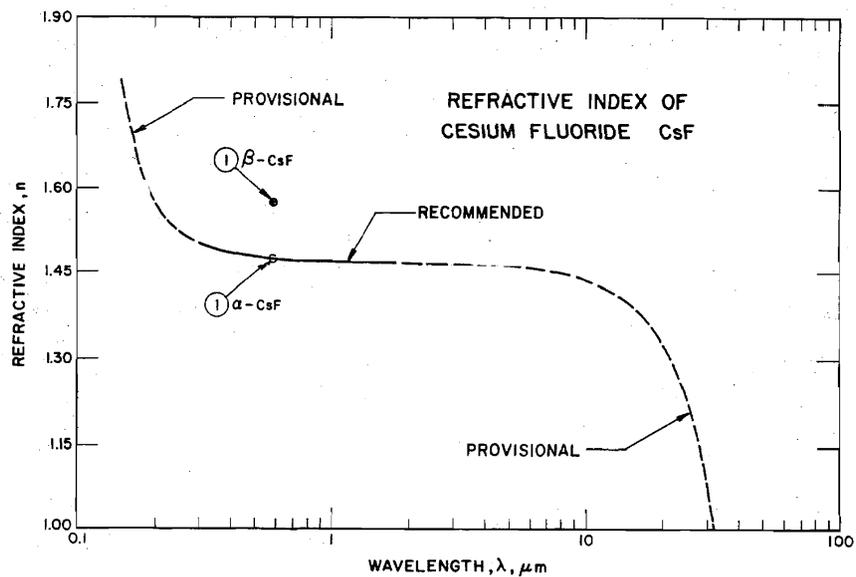
FIGURE 56. Refractive Index of CsF
