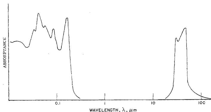
FIGURE 1. Absorption Spectrum of a Typical Alkali-Halide Crystal
