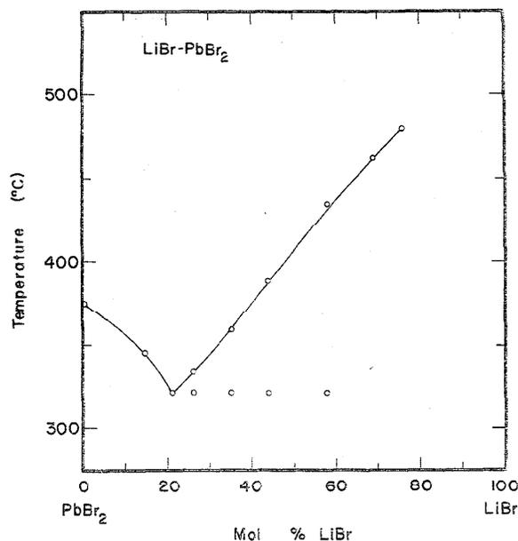
FIGURE 35. Temperature-composition phase diagram for LiBr-PbBr<sub>2</sub>.
