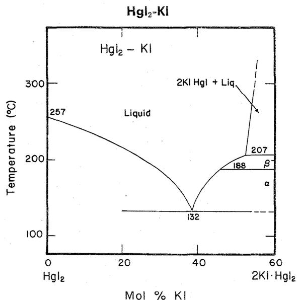
FIGURE 56. Temperature-composition phase diagram for  $\text{HgI}_2$ -KI.
