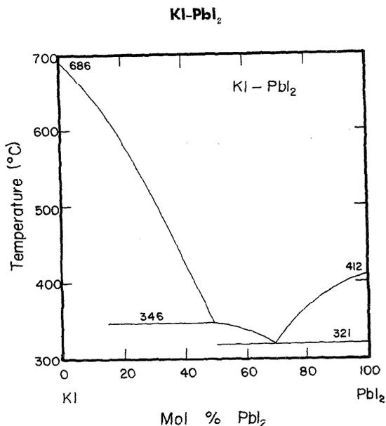
FIGURE 62. Temperature-composition phase diagram for KI-PbI<sub>2</sub>.
