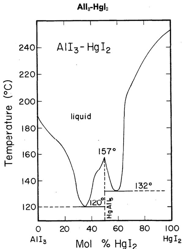
FIGURE 42. Temperature-composition phase diagram for All<sub>3</sub>-HgI<sub>2</sub>.
