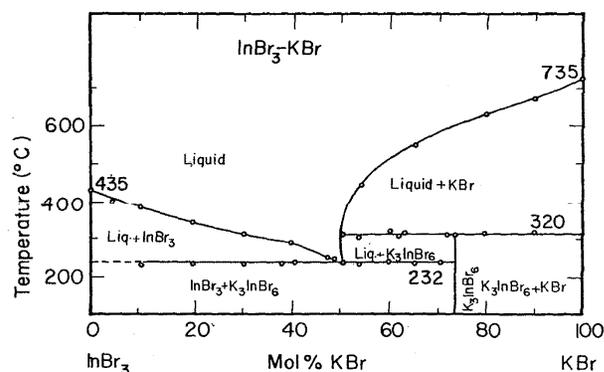
FIGURE 26. Temperature-composition phase diagram for InBr<sub>3</sub>-KBr.
