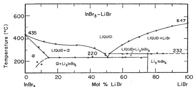
FIGURE 27. Temperature-composition phase diagram for InBr<sub>3</sub>-LiBr.
