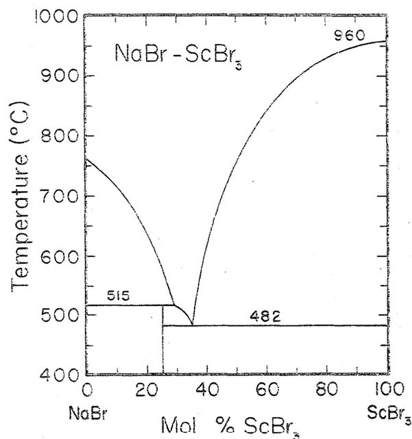
FIGURE 39. Temperature-composition phase diagram for NaBr-ScBr<sub>3</sub>.
