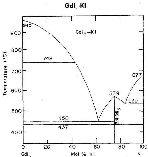
FIGURE 53. Temperature-composition phase diagram for  $GdI_3$ -KI.
