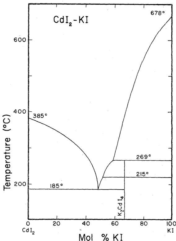
FIGURE 45. Temperature-composition phase diagram for CdI<sub>2</sub>-KI.
