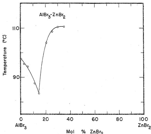
FIGURE 12. Temperature-composition phase diagram for  $\text{AlBr}_3\text{-ZnBr}_2$ .
