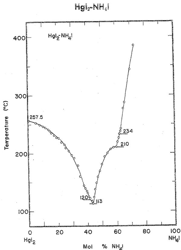
FIGURE 57. Temperature-composition phase diagram for  $\text{HgI}_2\text{-NH}_4\text{I}$ .
