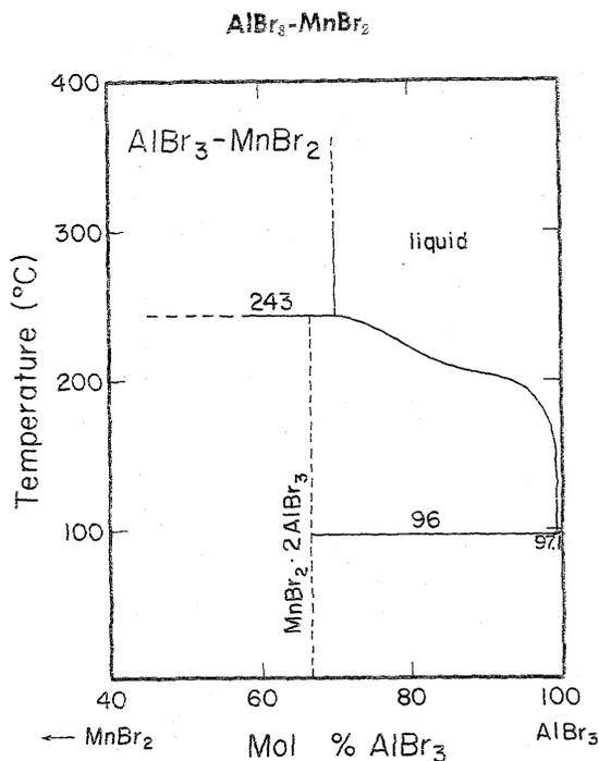
FIGURE 8. Temperature-composition phase diagram for  $\text{AlBr}_3\text{-MnBr}_2$ .
