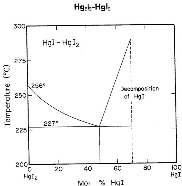
FIGURE 55. Temperature-composition phase diagram for  $Hg_2I_2$ -HgI<sub>2</sub>.
