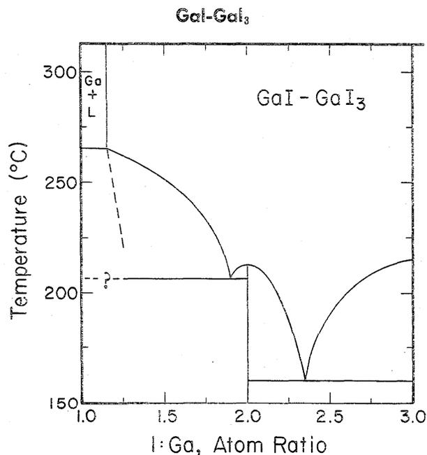
FIGURE 52. Temperature-composition phase diagram for  $\text{GaI-GaI}_3$ .
