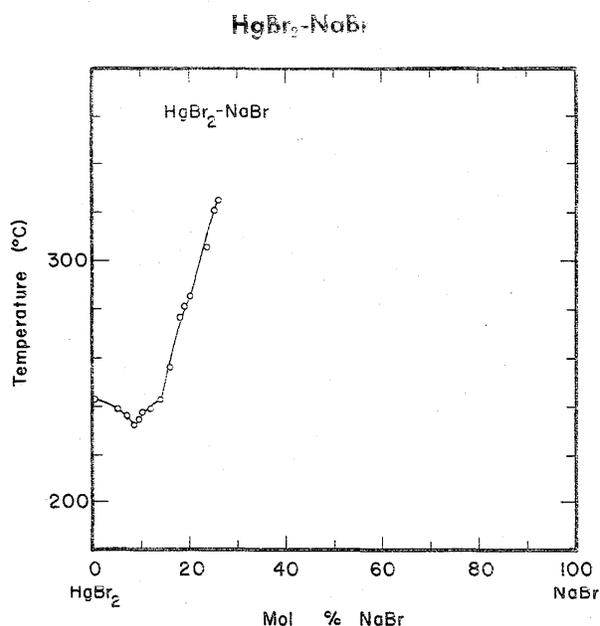
FIGURE 23. Temperature-composition phase diagram for HgBr<sub>2</sub>-NaBr.
