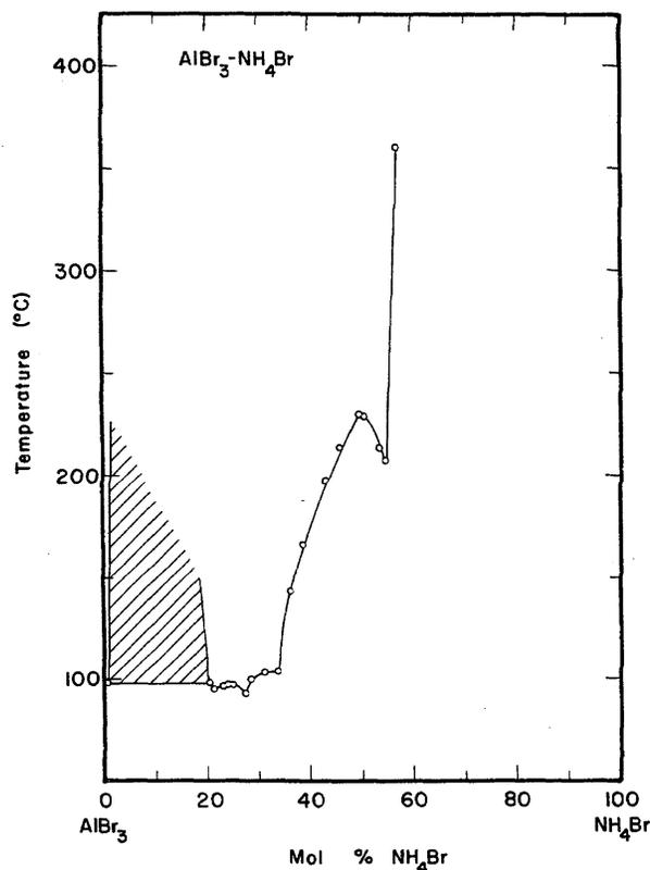
FIGURE 10. Temperature-composition phase diagram for  $\text{AlBr}_3\text{-NH}_4\text{Br}$ .
