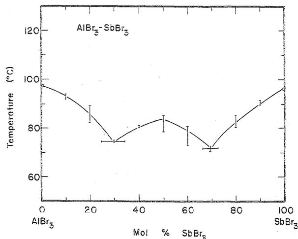
FIGURE 11. Temperature-composition phase diagram for  $\text{AlBr}_3\text{-SbBr}_3$ .
