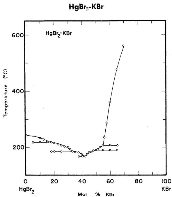
FIGURE 22. Temperature-composition phase diagram for HgBr<sub>2</sub>-KBr.
