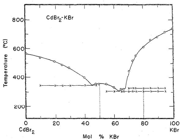
FIGURE 15. Temperature-composition phase diagram for CdBr<sub>2</sub>-KBr.
