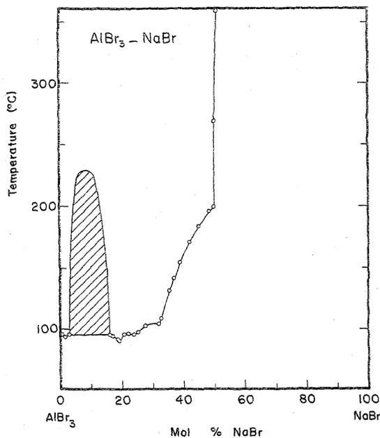
FIGURE 9. Temperature-composition phase diagram for  $\text{AlBr}_3\text{-NaBr}$ .
