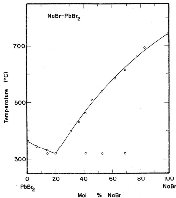
FIGURE 37. Temperature-composition phase diagram for NaBr-PbBr<sub>2</sub>.
