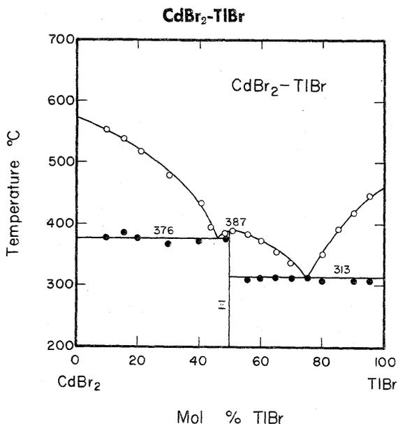
FIGURE 17. Temperature-composition phase diagram for CdBr<sub>2</sub>-TlBr.
