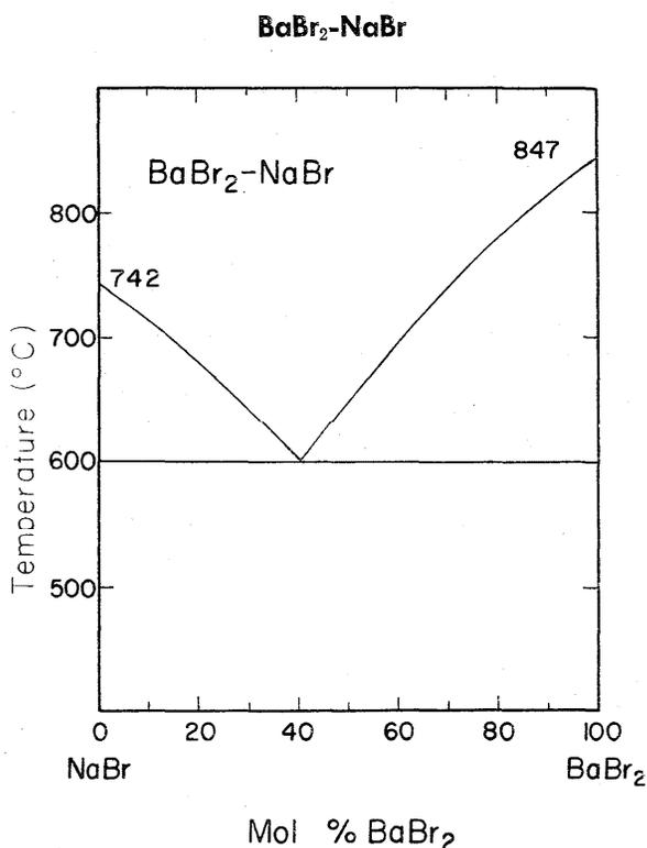
FIGURE 14. Temperature-composition phase diagram for BaBr<sub>2</sub>-NaBr.
