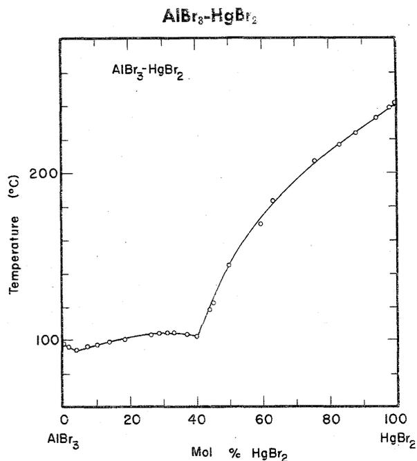
FIGURE 6. Temperature-composition phase diagram for  $\text{AlBr}_3$ - $\text{HgBr}_2$ .
