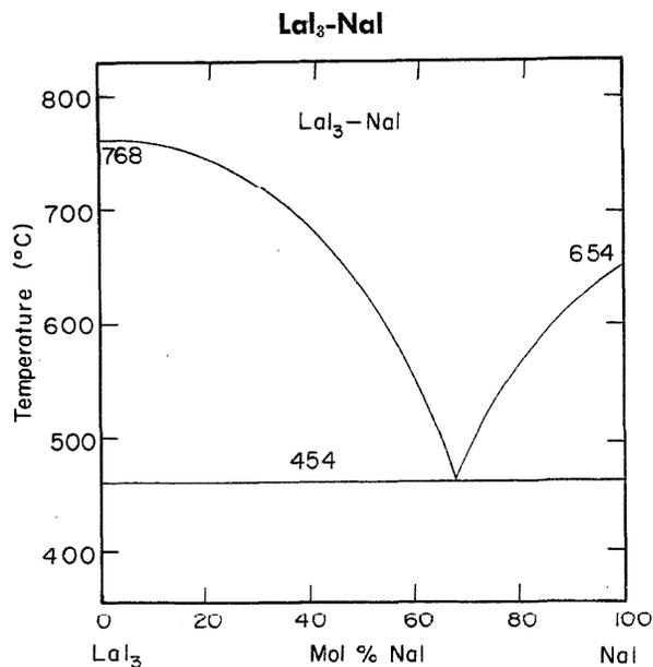
FIGURE 65. Temperature-composition phase diagram for LaI<sub>3</sub>-NaI.
