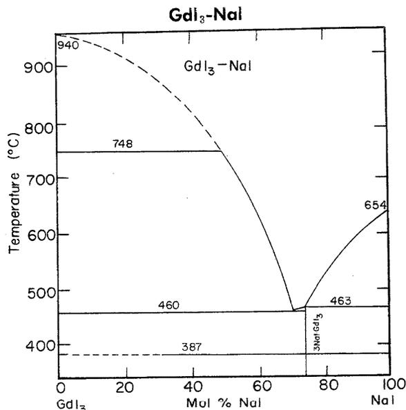
FIGURE 54. Temperature-composition phase diagram for  $GdI_3$ -NaI.
