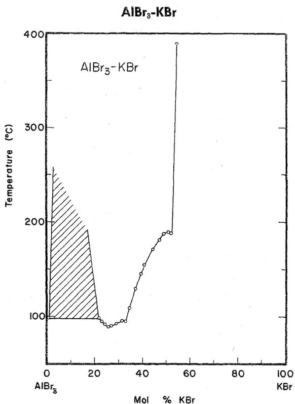
FIGURE 7. Temperature-composition phase diagram for  $\text{AlBr}_3\text{-KBr}$ .
