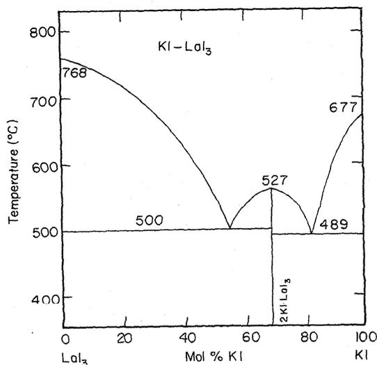
FIGURE 58. Temperature-composition phase diagram for KI-LaI<sub>3</sub>.
