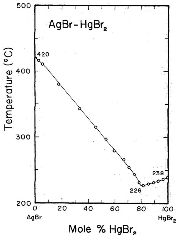
FIGURE 1. Temperature-composition phase diagram for AgBr-HgBr<sub>2</sub>.
