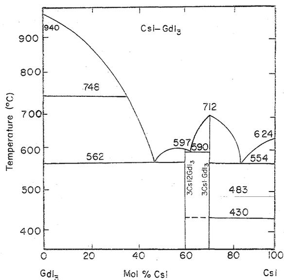
FIGURE 48. Temperature-composition phase diagram for CsI-GdI<sub>3</sub>.
