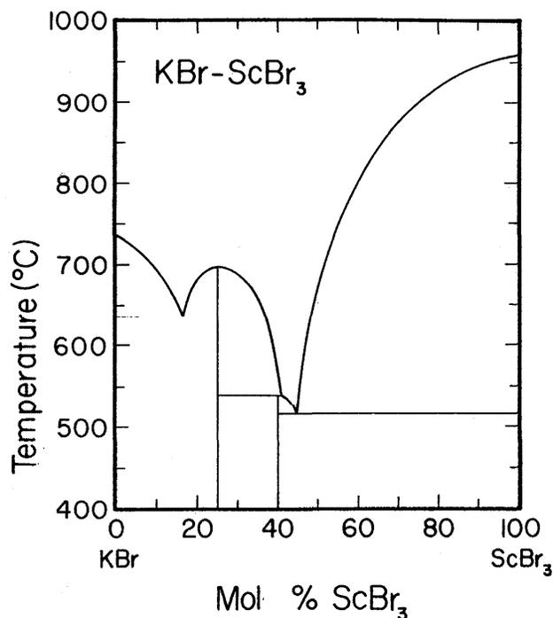
FIGURE 32. Temperature-composition phase diagram for KBr-ScBr<sub>3</sub>.
