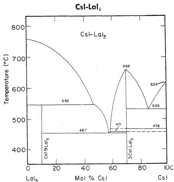
FIGURE 40. Temperature-composition phase diagram for CsI-LaI<sub>3</sub>.
