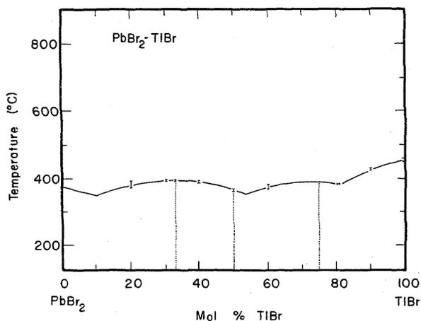
FIGURE 40. Temperature-composition phase diagram for PbBr<sub>2</sub>-TlBr.
