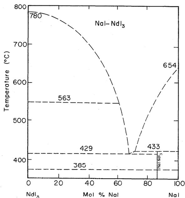
FIGURE 66. Temperature-composition phase diagram for NaI-NdI<sub>3</sub>.
