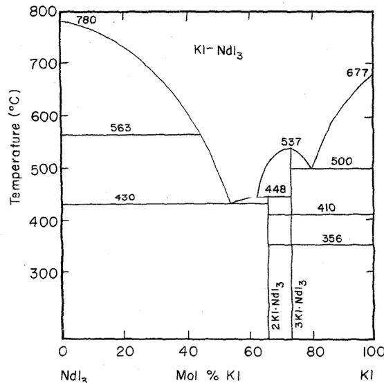
FIGURE 61. Temperature-composition phase diagram for KI-NdI<sub>3</sub>.
