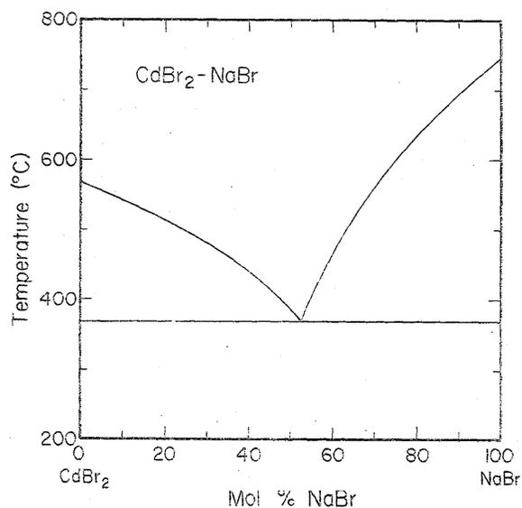
FIGURE 16. Temperature-composition phase diagram for CdBr<sub>2</sub>-NaBr.
