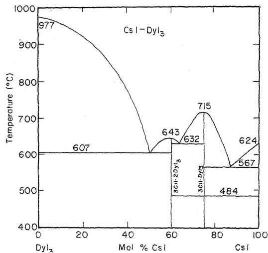
FIGURE 47. Temperature-composition phase diagram for CsI-DyI<sub>3</sub>.
