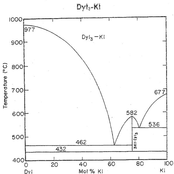
FIGURE 51. Temperature-composition phase diagram for  $\text{DyI}_3\text{-KI}$ .
