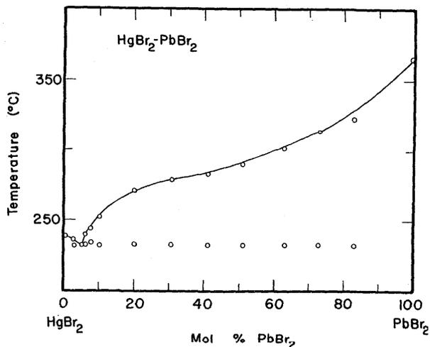
FIGURE 25. Temperature-composition phase diagram for HgBr<sub>2</sub>-PbBr<sub>2</sub>.
