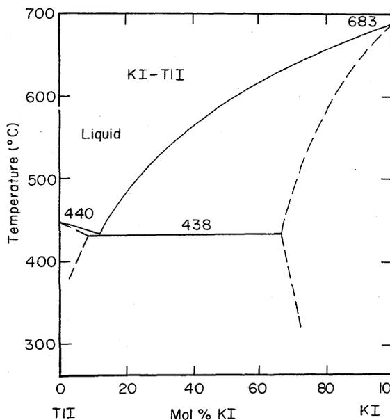
FIGURE 64. Temperature-composition phase diagram for KI-TII.
