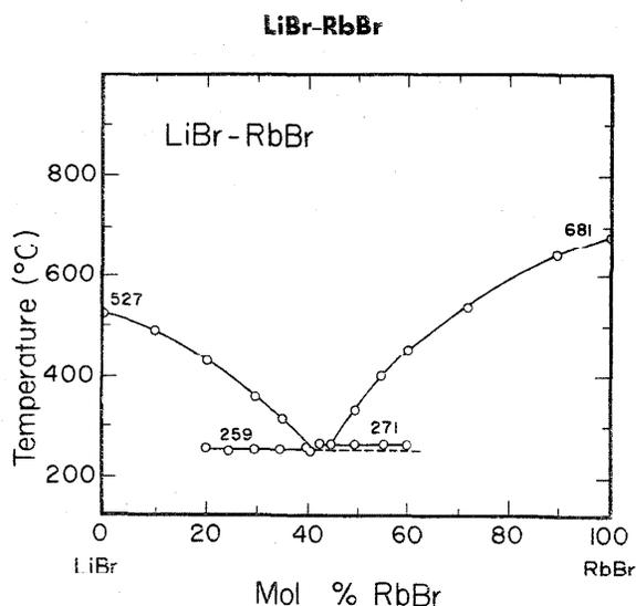
FIGURE 36. Temperature-composition phase diagram for LiBr-RbBr.
