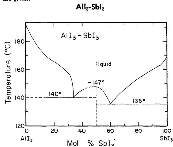
FIGURE 44. Temperature-composition phase diagram for  $\text{AlI}_3\text{-SbI}_3$ .
