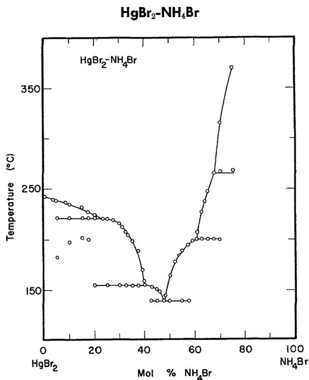
FIGURE 24. Temperature-composition phase diagram for HgBr<sub>2</sub>-NH<sub>4</sub>Br.
