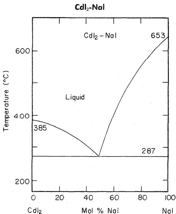
FIGURE 46. Temperature-composition phase diagram for CdI<sub>2</sub>-NaI.
