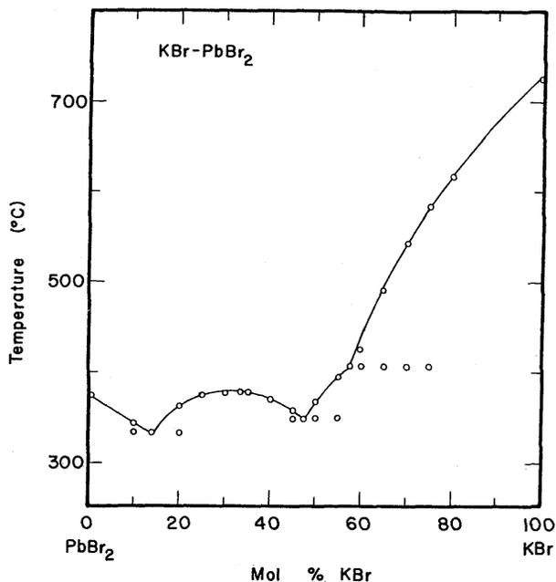
FIGURE 30. Temperature-composition phase diagram for KBr-PbBr<sub>2</sub>.
