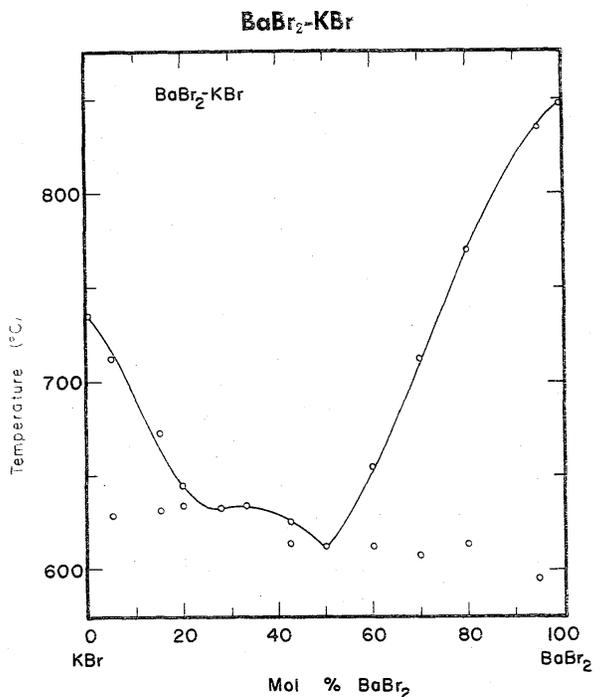
FIGURE 13. Temperature-composition phase diagram for BaBr<sub>2</sub>-KBr.
