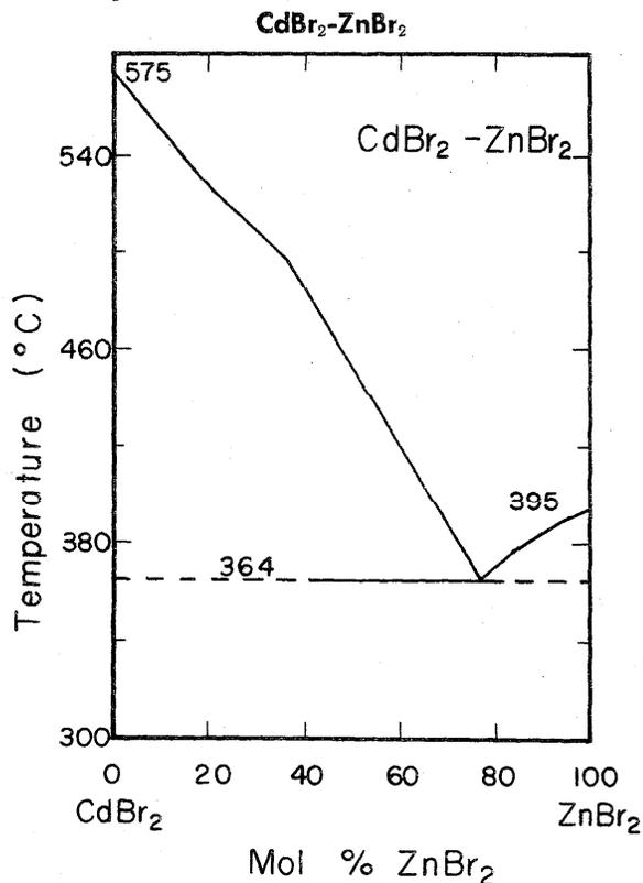
FIGURE 18. Temperature-composition phase diagram for CdBr<sub>2</sub>-ZnBr<sub>2</sub>.
