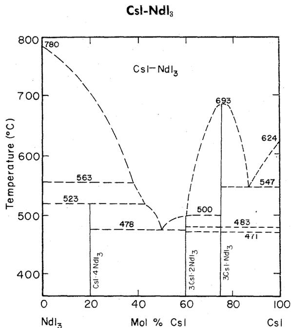
FIGURE 50. Temperature-composition phase diagram for CsI-NdI<sub>3</sub>.
