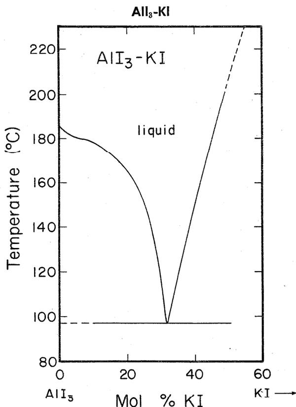
FIGURE 43. Temperature-composition phase diagram for  $\text{AlI}_3\text{-KI}$ .
