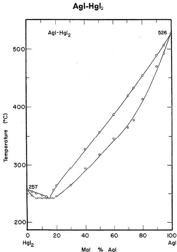
FIGURE 41. Temperature-composition phase diagram for AgI-HgI<sub>2</sub>.
