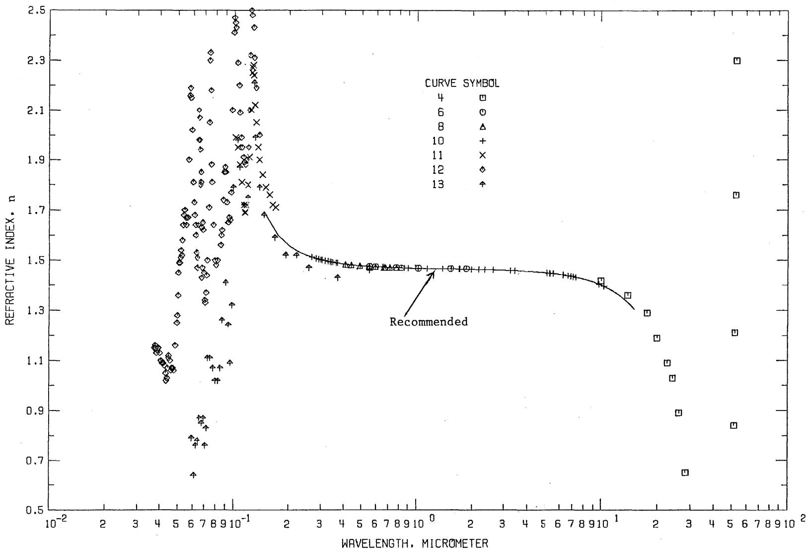
FIGURE 16. REFRACTIVE INDEX OF BARIUM FLUORIDE (WAVELENGTH DEPENDENCE).
