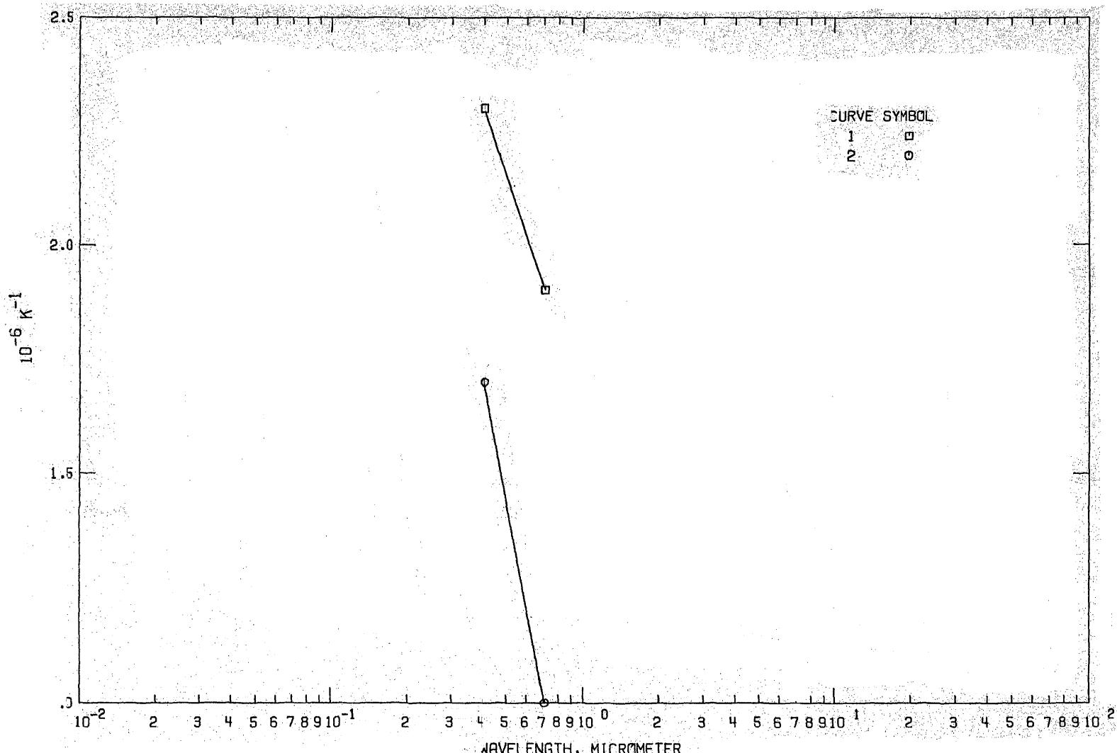
FIGURE 24. TEMPERATURE DERIVATIVE OF REFRACTIVE INDEX OF MAGNESIUM FLUORIDE (WAVELENGTH DEPENDENCE)
