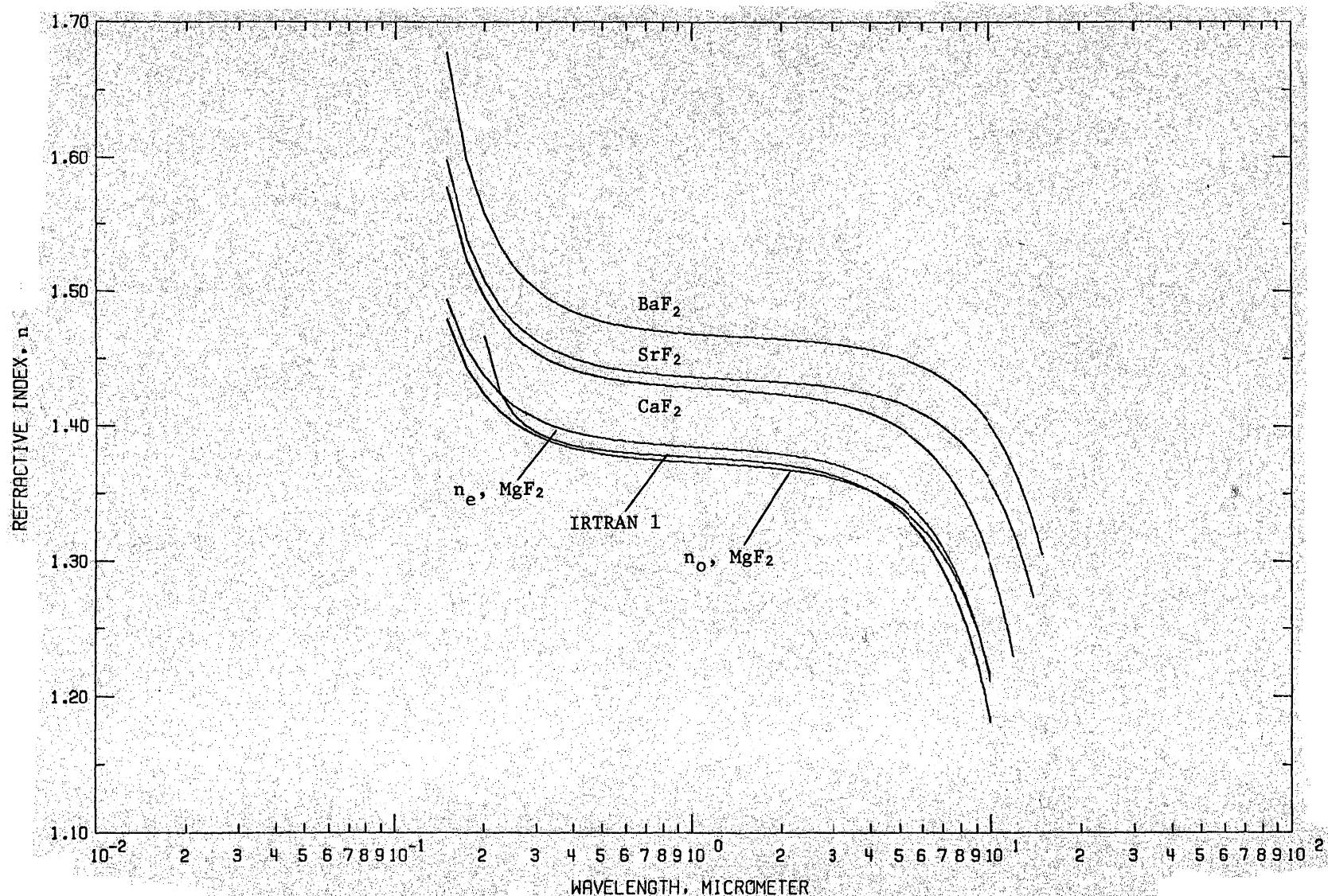
FIGURE 29. REFRACTIVE INDEX OF ALKALINE EARTH HALIDES (WAVELENGTH DEPENDENCE).
