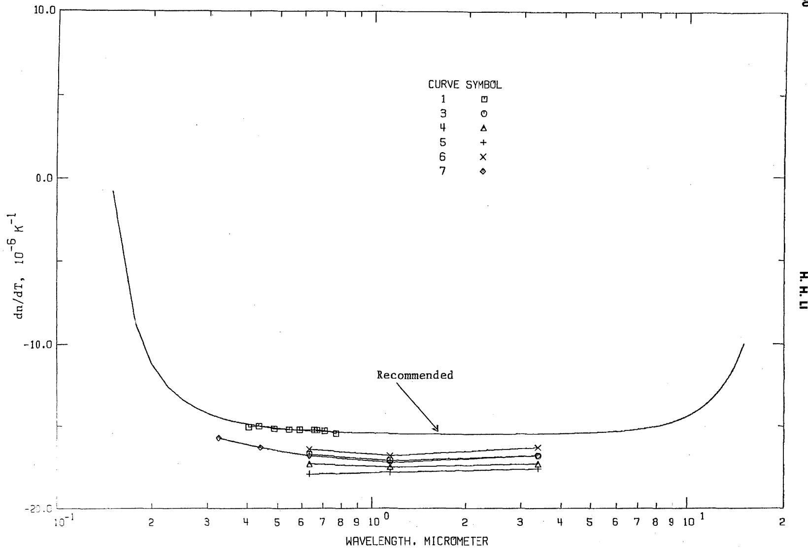
FIGURE 19. TEMPERATURE DERIVATIVE OF REFRACTIVE INDEX OF BARIUM FLUORIDE (WAVELENGTH DEPENDENCE).
