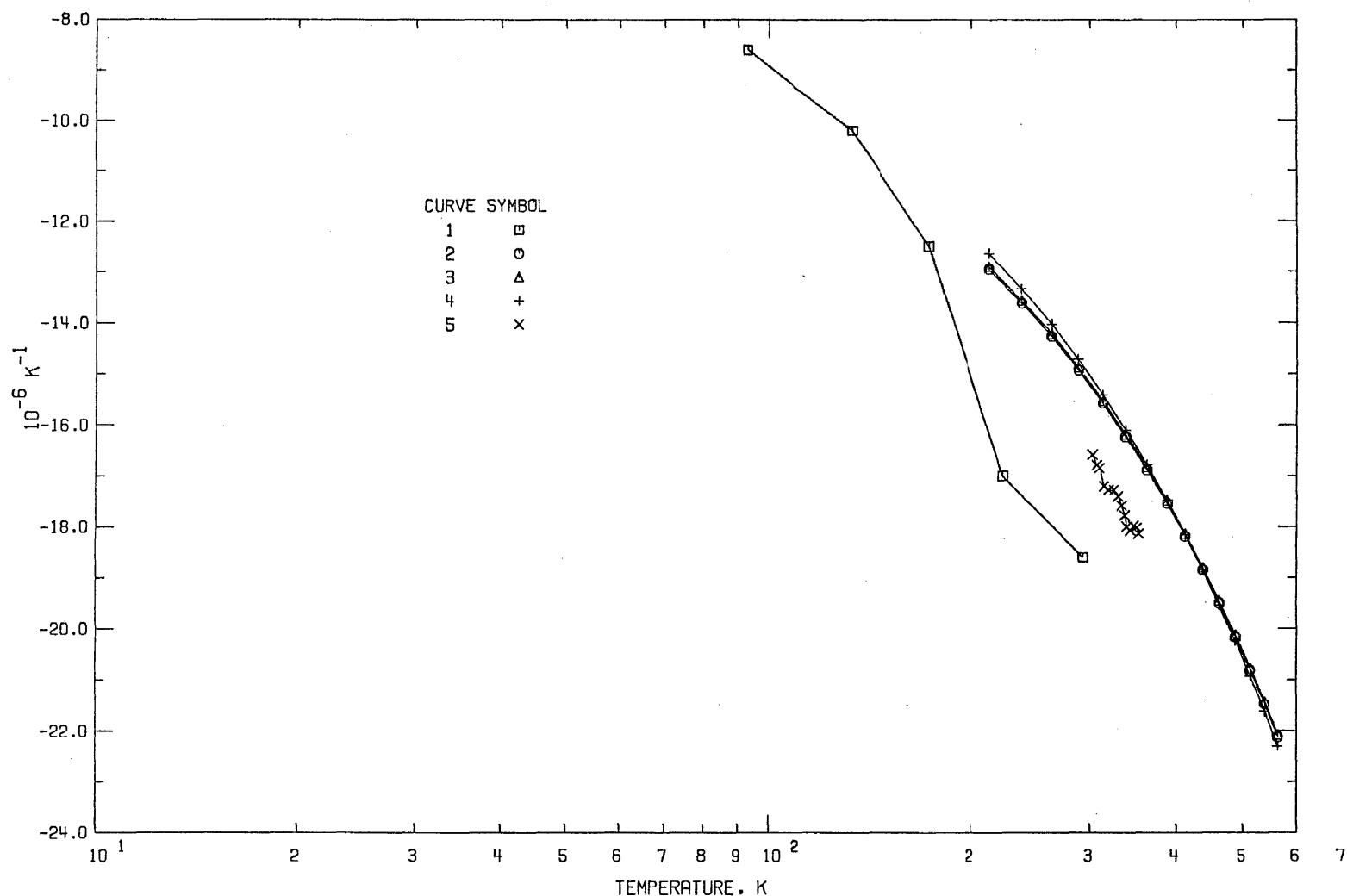
FIGURE 20. TEMPERATURE DERIVATIVE OF REFRACTIVE INDEX OF BARIUM FLUORIDE (TEMPERATURE DEPENDENCE).
