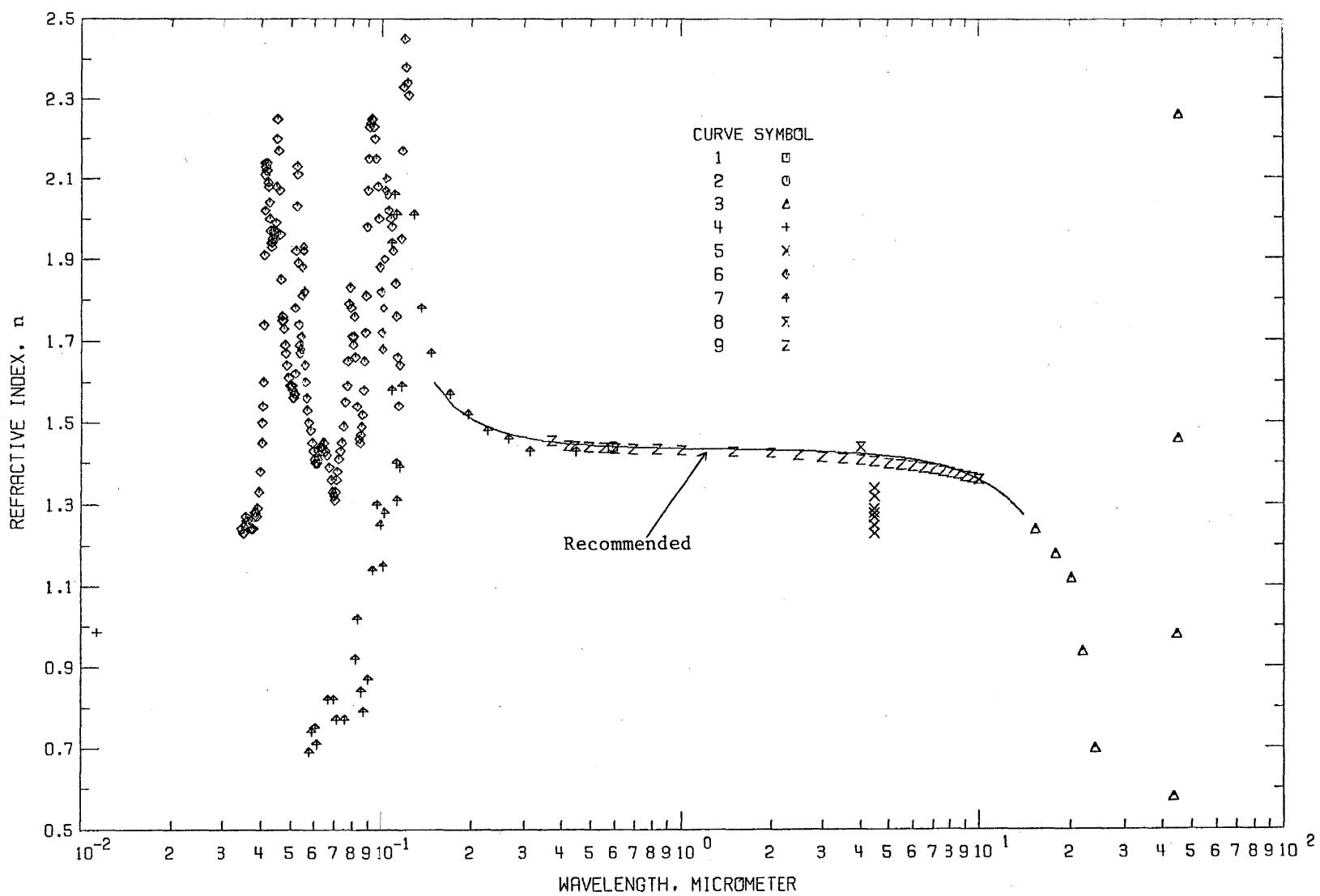
FIGURE 12. REFRACTIVE INDEX OF STRONTIUM FLUORIDE (WAVELENGTH DEPENDENCE).
