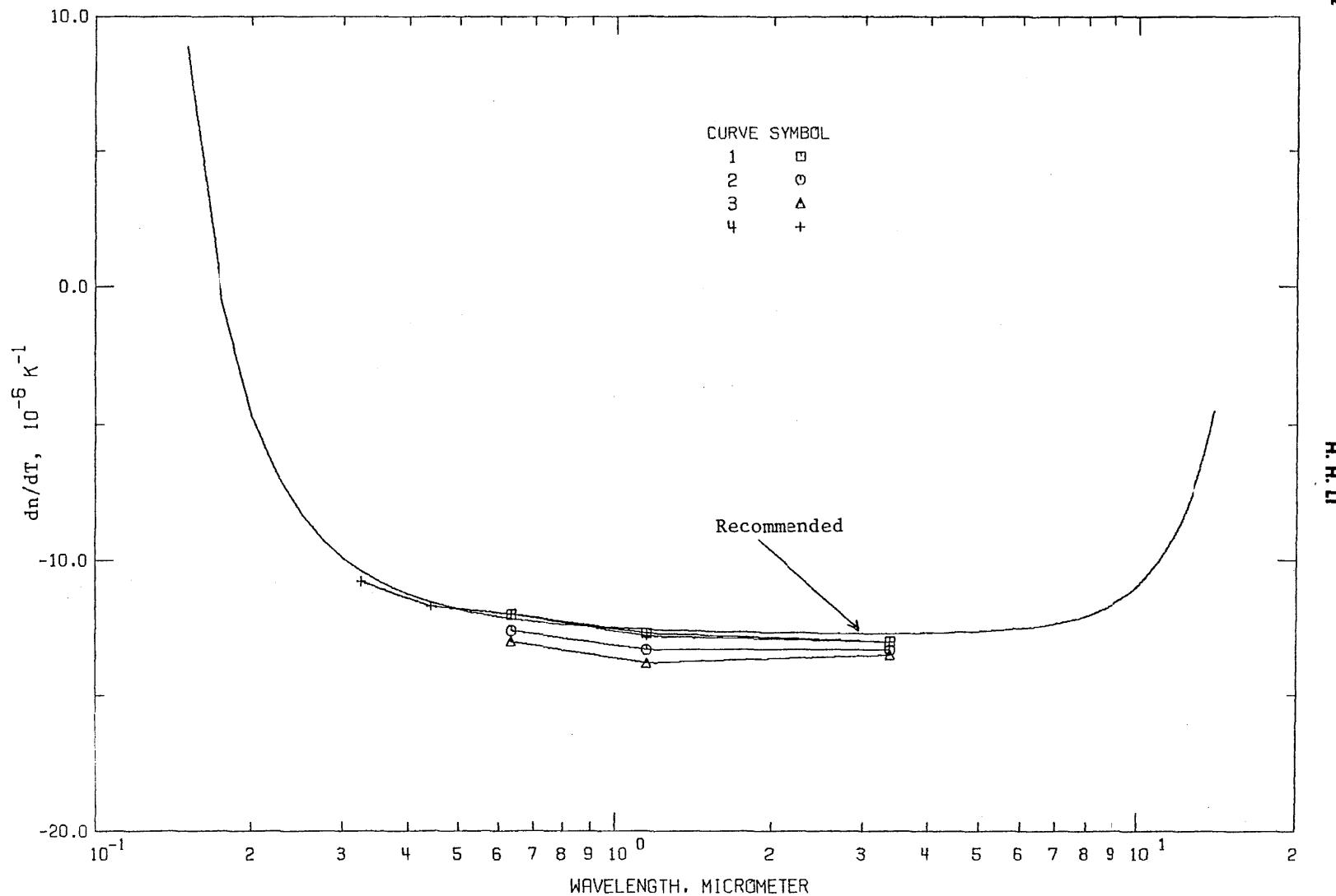
FIGURE 15. TEMPERATURE DERIVATIVE OF REFRACTIVE INDEX OF STRONTIUM FLUORIDE (WAVELENGTH DEPENDENCE)
