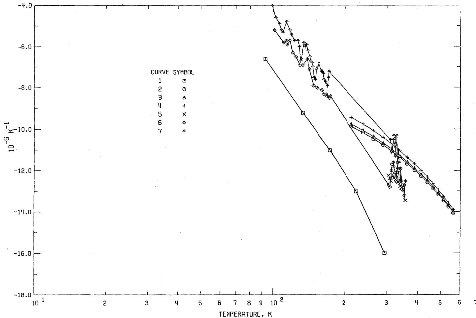
FIGURE 11. TEMPERATURE DERIVATIVE OF REFRACTIVE INDEX OF CALCIUM FLUORIDE (TEMPERATURE DEPENDENCE).
