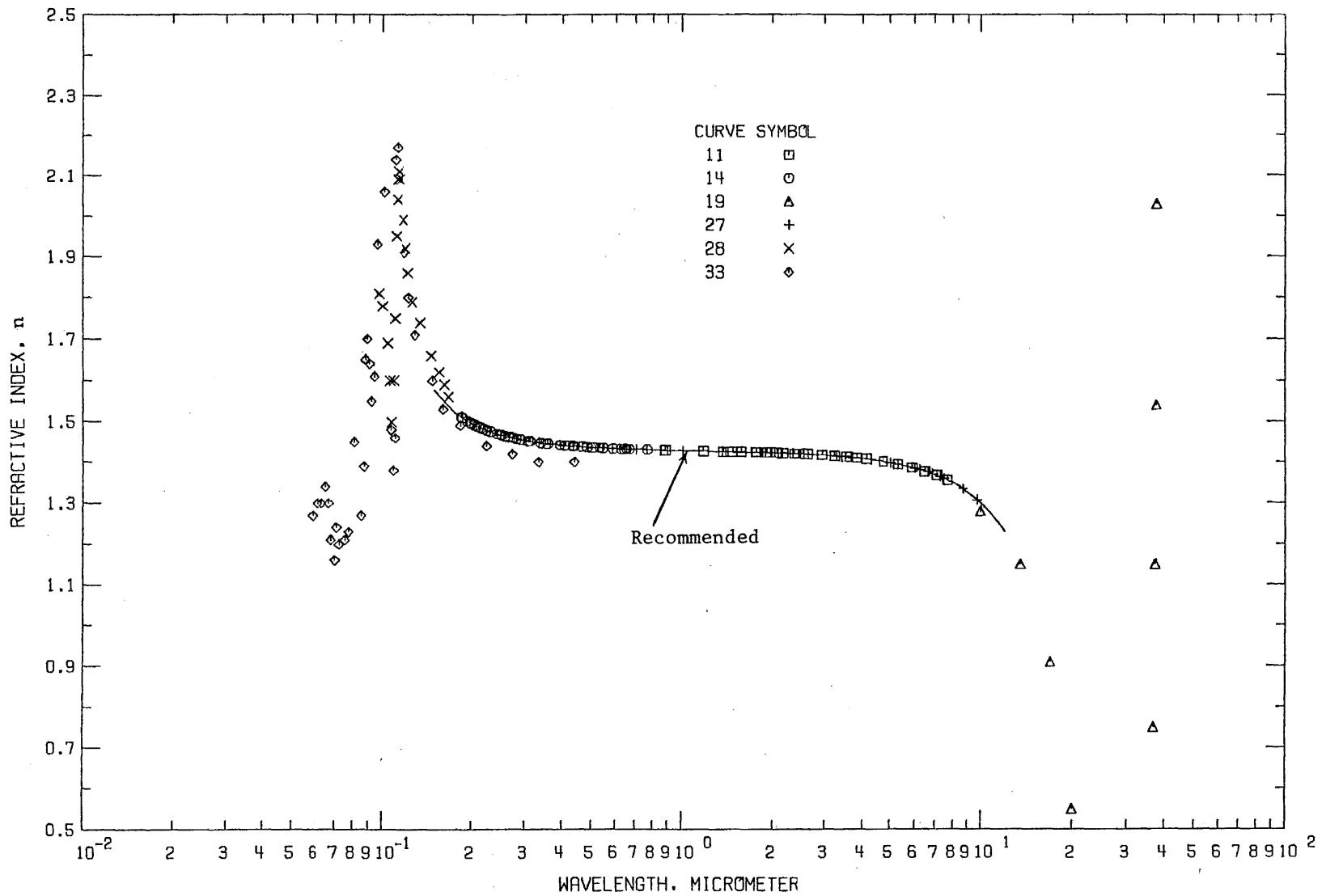
FIGURE 7. REFRACTIVE INDEX OF CALCIUM FLUORIDE (WAVELENGTH DEPENDENCE).
