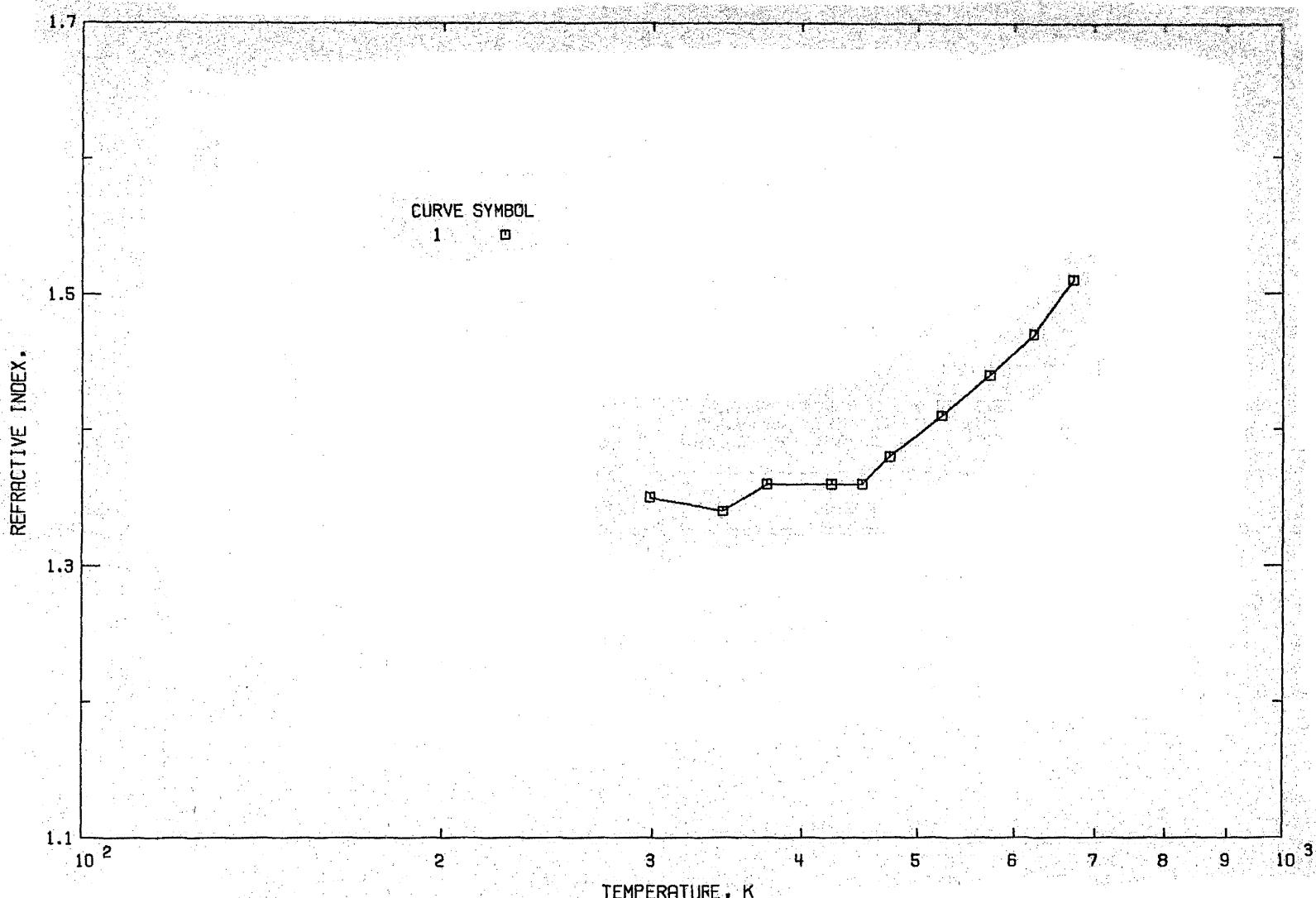
FIGURE 14. REFRACTIVE INDEX OF STRONTIUM FLUORIDE (TEMPERATURE DEPENDENCE).
