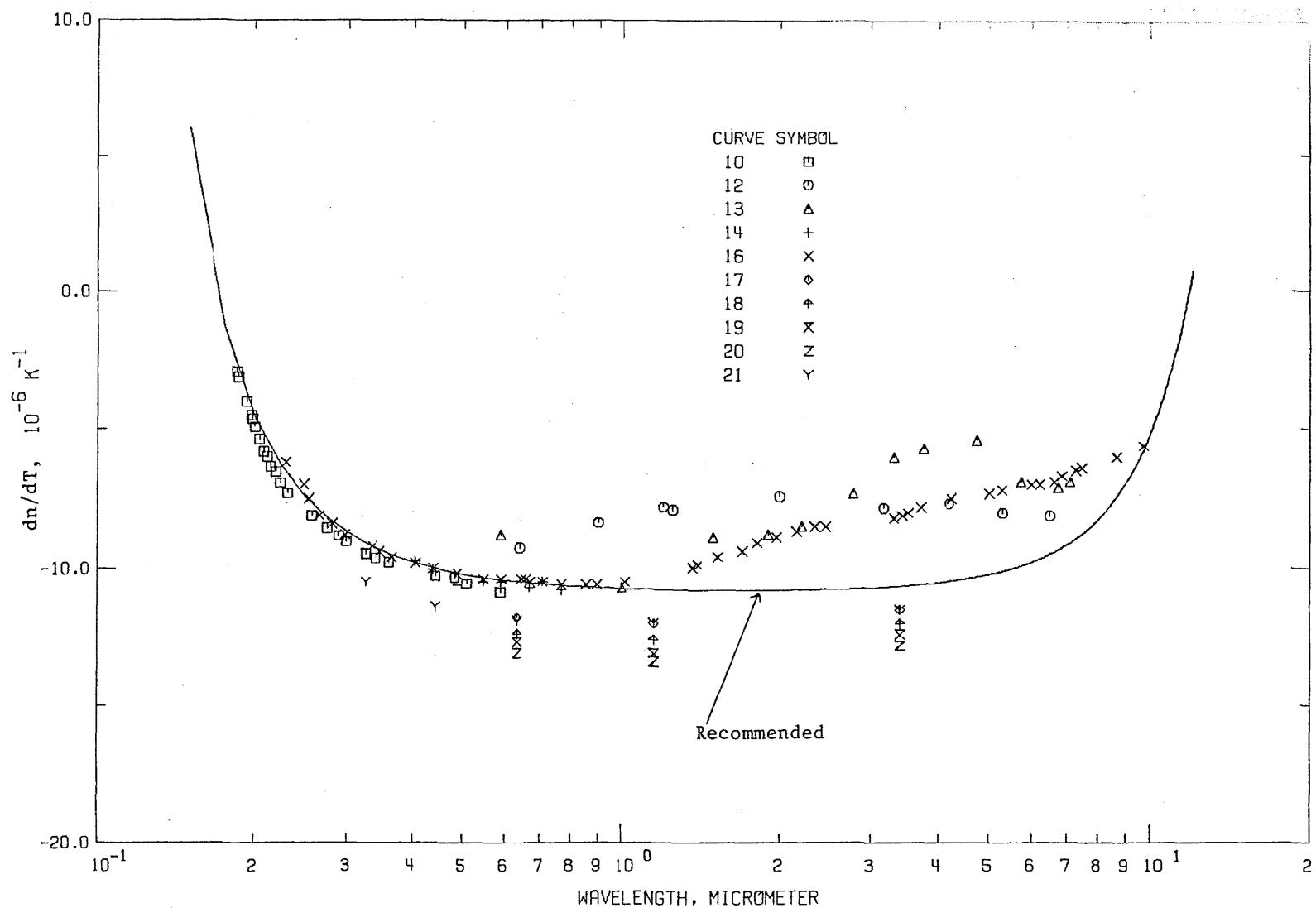
FIGURE 10. TEMPERATURE DERIVATIVE OF REFRACTIVE INDEX OF CALCIUM FLUORIDE (WAVELENGTH DEPENDENCE).
