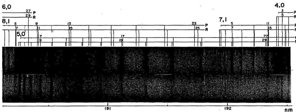
FIG. 6. The (5,0) Schumann-Runge band region of O<sub>2</sub>.
