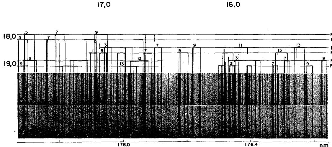
FIG. 17. The (16,0) and (17,0) Schumann-Runge band region of  $O_2$ .
