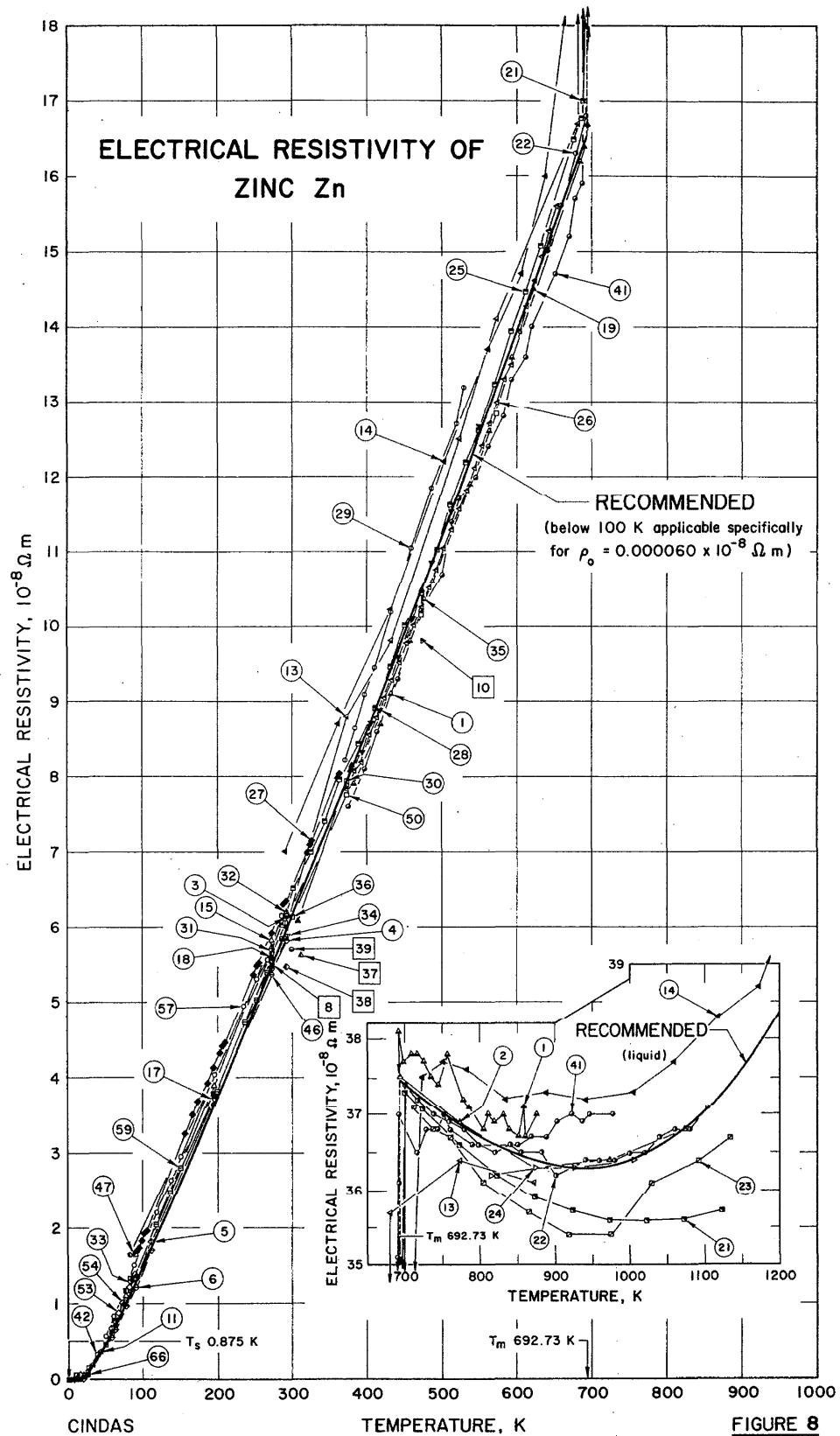
TABLE 4. RECOMMENDED VALUES FOR THE ELECTRICAL RESISTIVITY OF ZINC<sup>a</sup>{Temperature, T, K; Electrical Resistivity,  $\rho$ ,  $10^{-8} \Omega \text{ m}$ }
