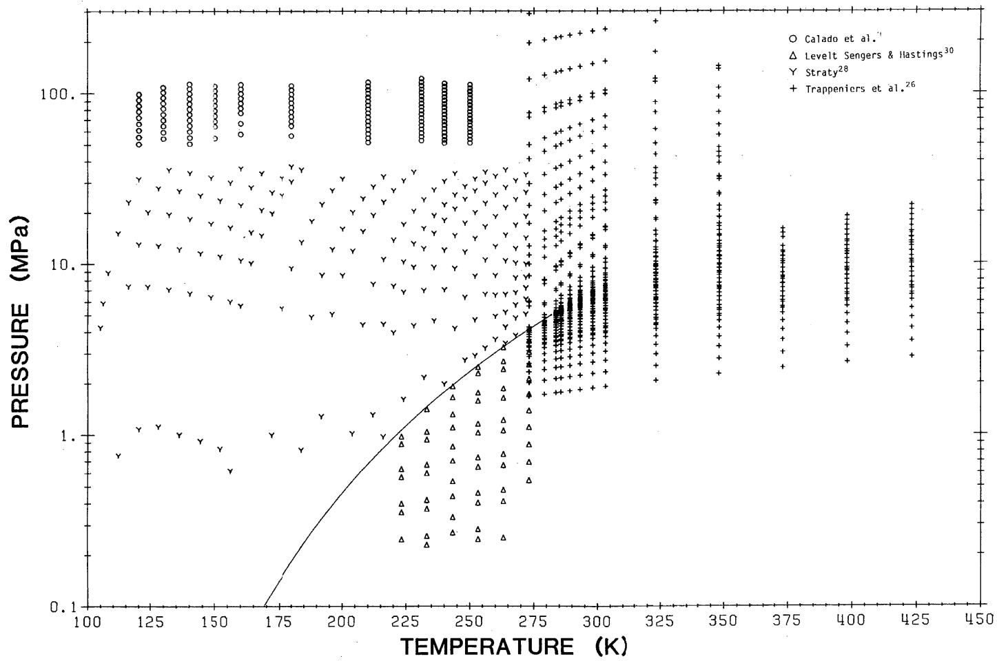
FIG. 12. Ethylene  $P$ - $\rho$ - $T$  data used in the determination of the fundamental equation.
