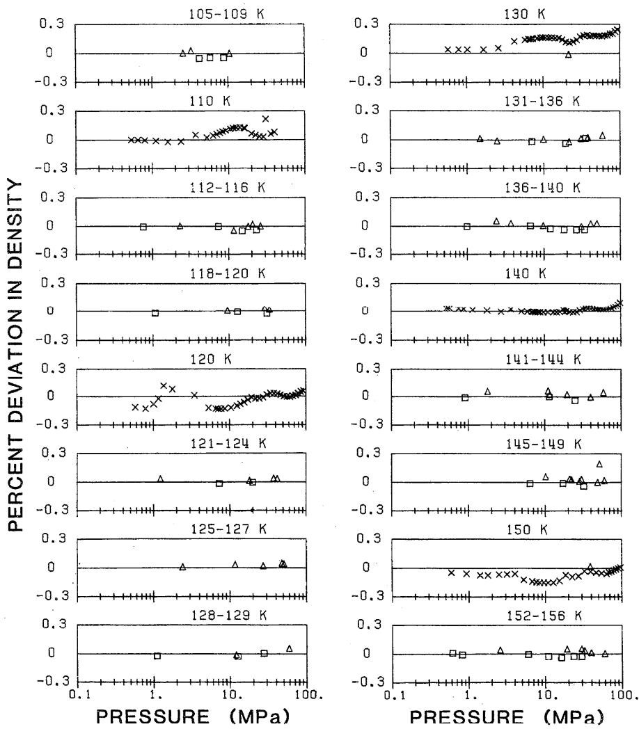
FIG. 15. Comparisons of calculated values of density to data for the liquid below the critical temperature.
