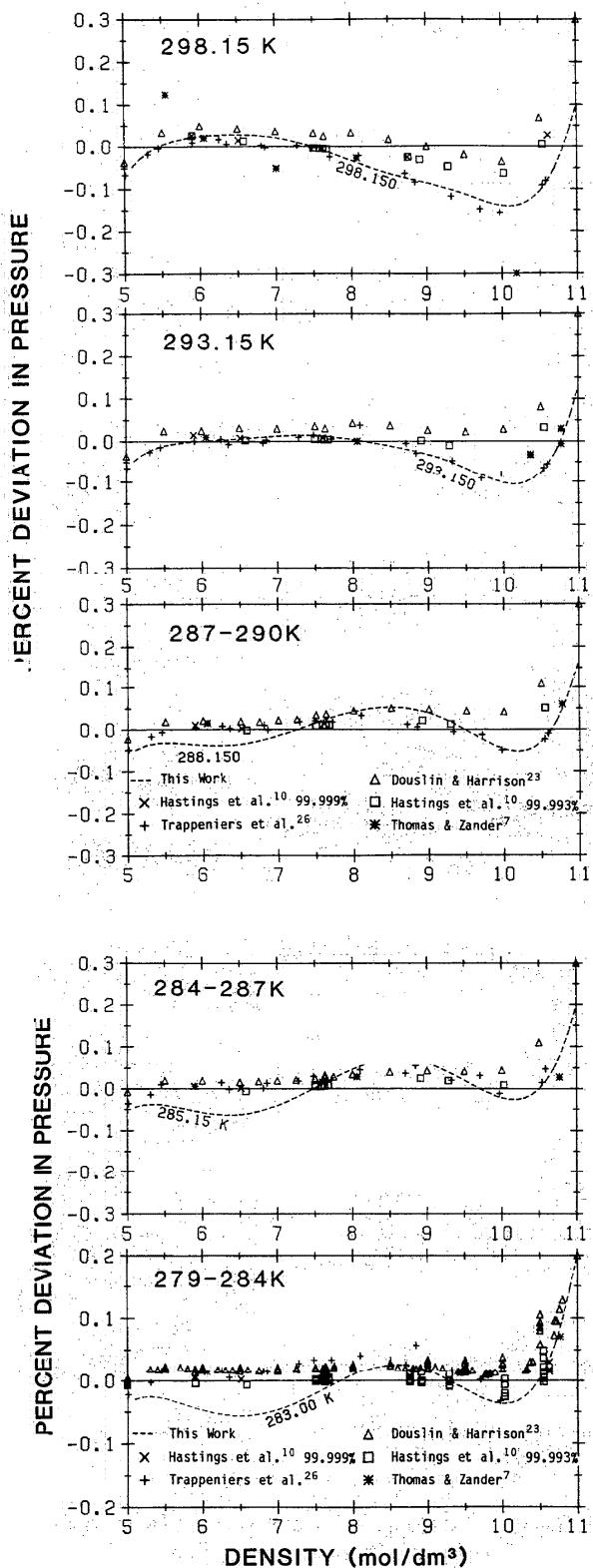
FIG. 31. Pressure deviations of equation of state and  $P\rho-T$  data from the revised and extended scaling equation in the critical region. [The zero deviation line is the formulation of Levent Sengers *et al.* (Ref. 12).]
