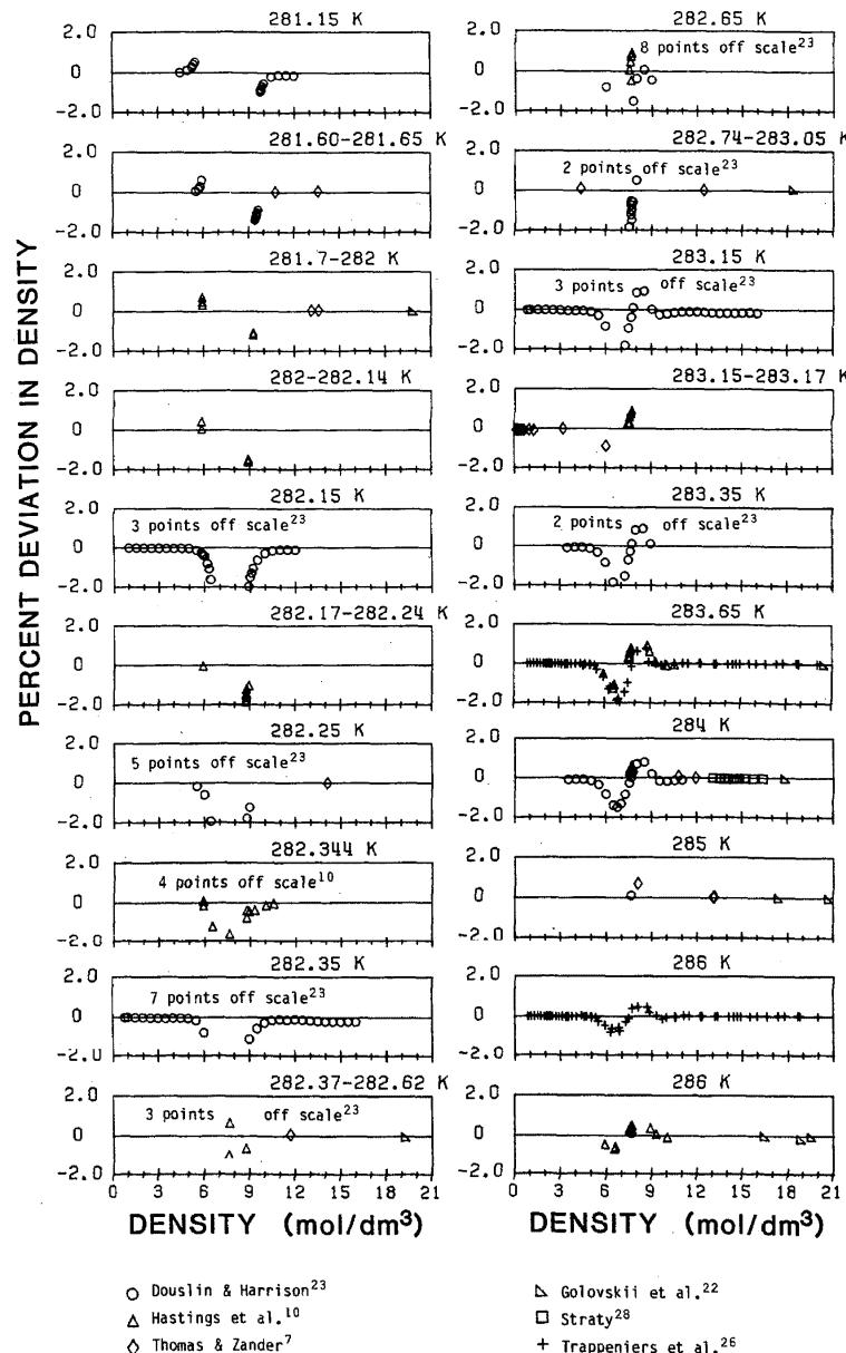
FIG. 18. Comparisons of calculated values of density to data near the critical temperature ( $T_c = 282.3452$  K,  $p_c = 7.6340$  mol/dm<sup>3</sup>).
