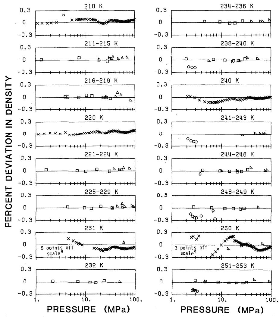
FIG. 15. Comparisons of calculated values of density to data for the liquid below the critical temperature—continued.
