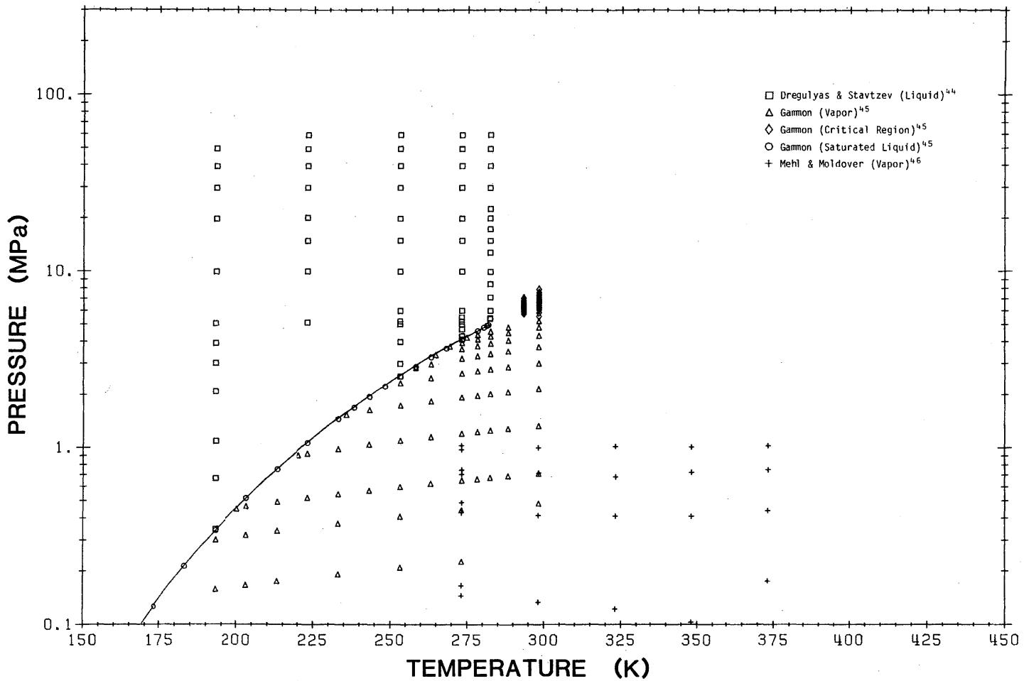
FIG. 14. Ethylene velocity of sound data used in the determination of the fundamental equation.
