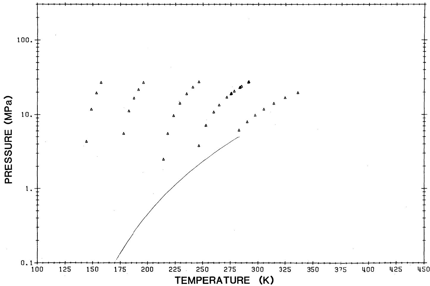
FIG. 13. Ethylene isochoric heat capacity of Weber (Ref. 36) used in the determination of the fundamental equation.
