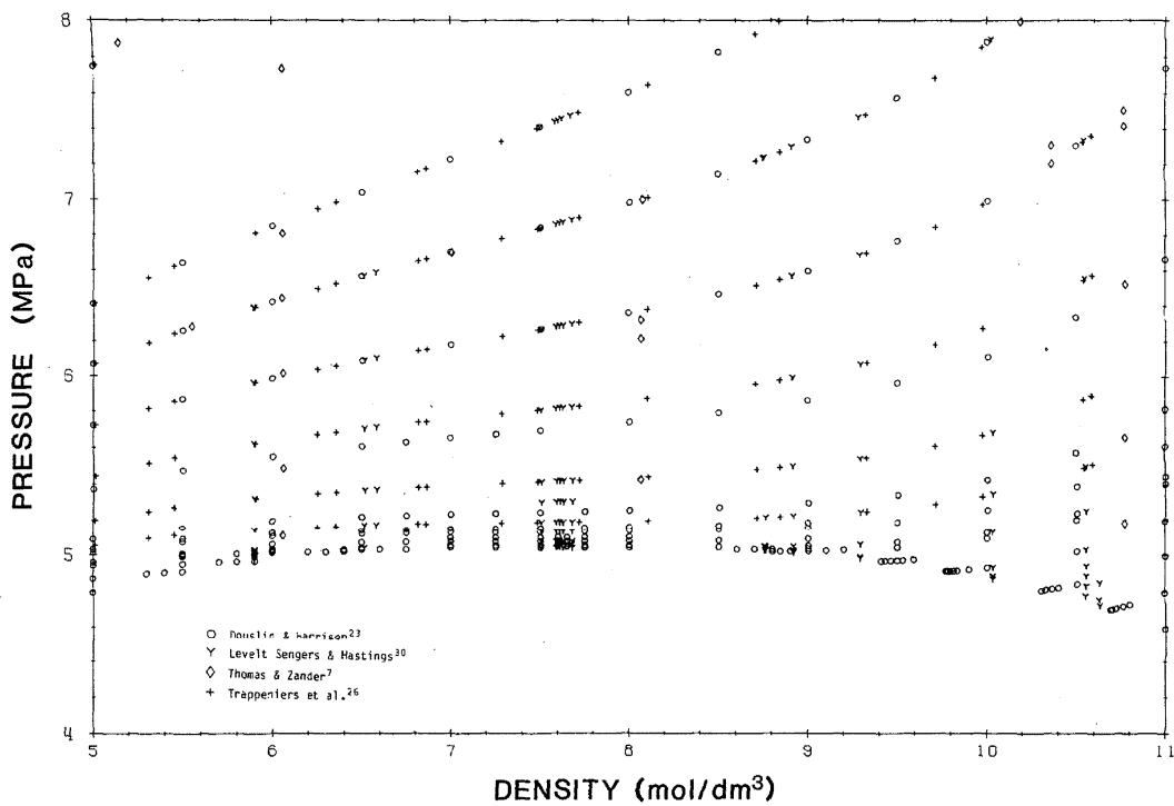
FIG. 2. Ethylene  $P$ - $\rho$ - $T$  data in the critical region.
