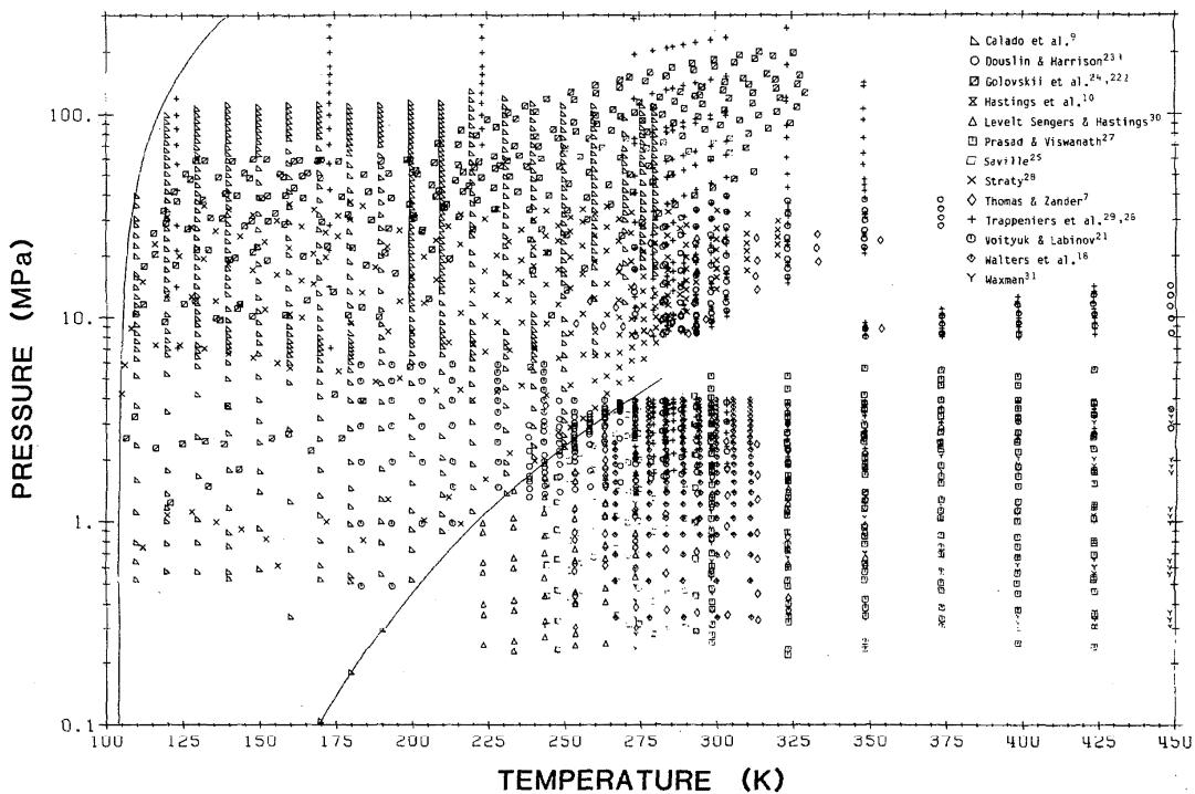
FIG. 1. Ethylene  $P$ - $\rho$ - $T$  data.
