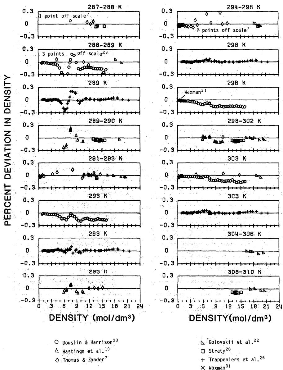
FIG. 17. Comparisons of calculated values of density to data for fluid states above the critical temperature.
