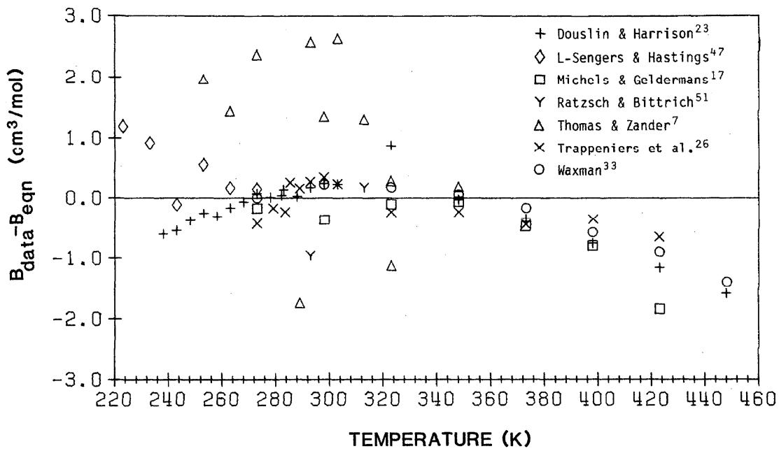
FIG. 25. Comparisons of calculated second virial coefficients with values from other sources [values of Thomas and Trappeniers each were calculated by Levlit Sengers &amp; Hastings (Ref. 47) from data given in Refs. 7 and 26, respectively].
