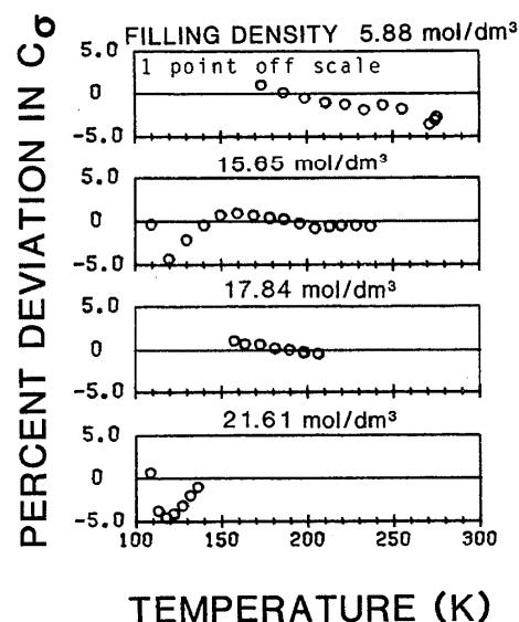
FIG. 20. Comparisons of calculated values of heat capacity,  $C_o$ , to data from Weber (Ref. 36).
