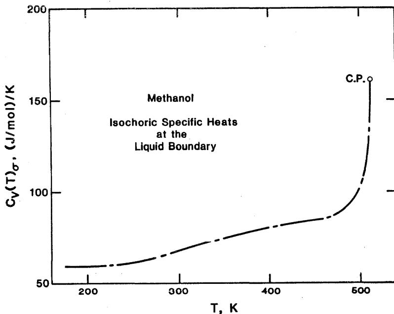
FIG. 3. Derived  $C_v(T)_\sigma$  at the liquid boundary.
