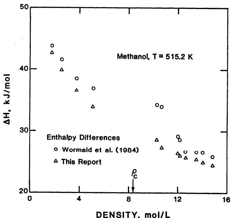
FIG. 4. Comparison of enthalpy differences at 515.2 K.
