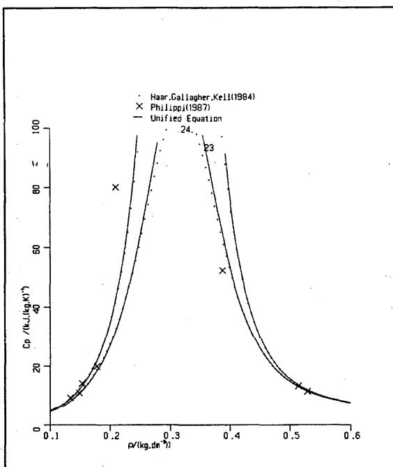
FIG. 111. Isopiestic specific heat  $C_p$ : 23–24 MPa.
