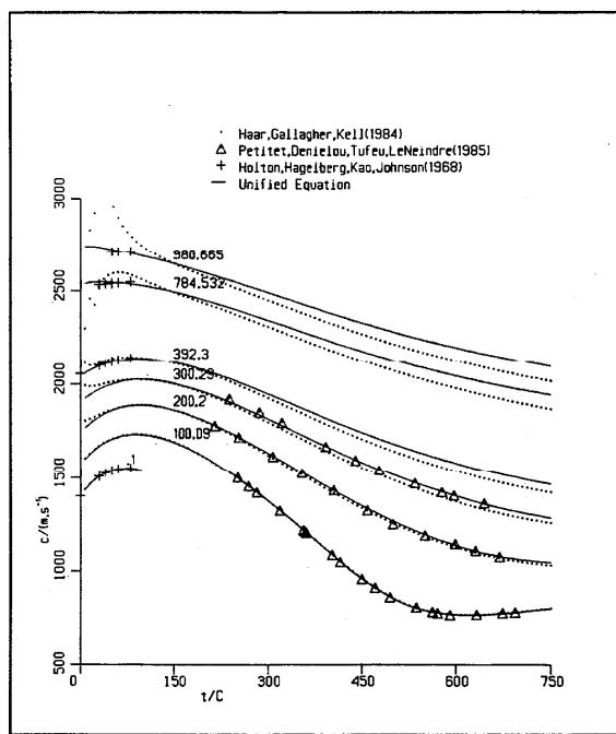
FIG. 98. Speed of sound, liquid: 0.1–1000 (P/MPa).
