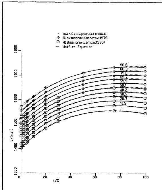
FIG. 95. Speed of sound, liquid: 0.1–100 MPa.
