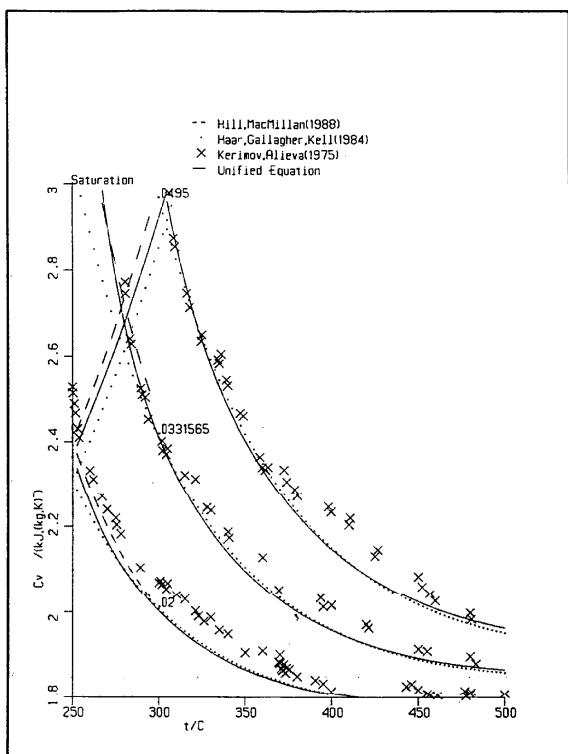
FIG. 114. Isochoric specific heat  $C_v$ : vapor isochores  $\text{kg dm}^{-3}$ .
