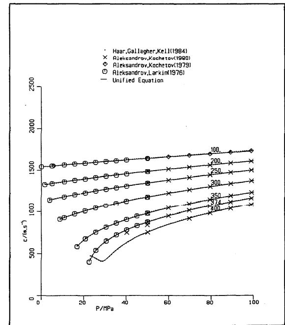
FIG. 97. Speed of sound, liquid: 100–400 °C.
