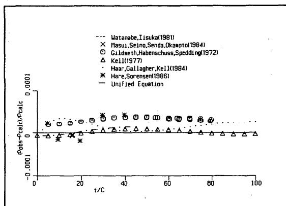
FIG. 73. Liquid density at 0.1 MPa and 0–100 °C.
