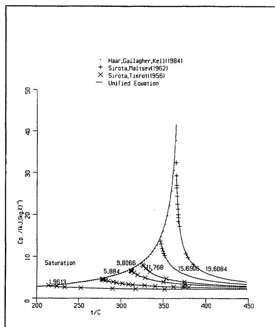
FIG. 108. Isopiestic specific heat  $C_p$ , vapor: 2–20 MPa.
