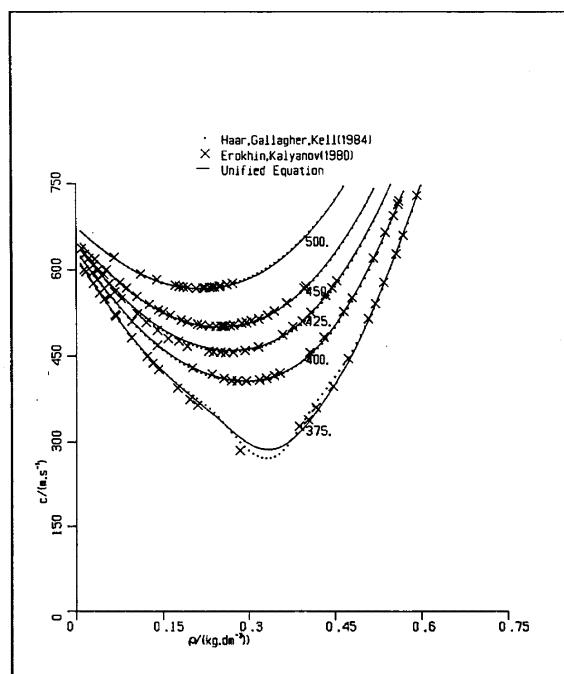
FIG. 99. Speed of sound, supercritical states: 375–500 °C.
