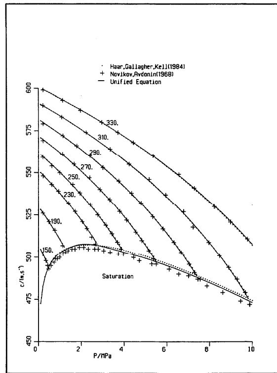
FIG. 100. Speed of sound, vapor: 150–330 °C.
