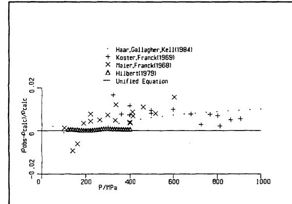
FIG. 70. Density at high pressures: 600 °C.
