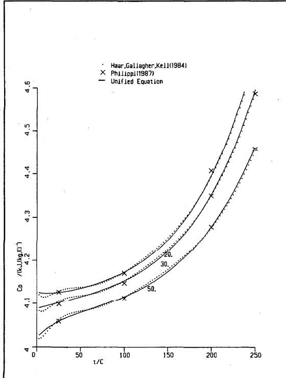
FIG. 105. Liquid Isopiestic specific heat  $C_p$ , liquid: 20–50 MPa.
