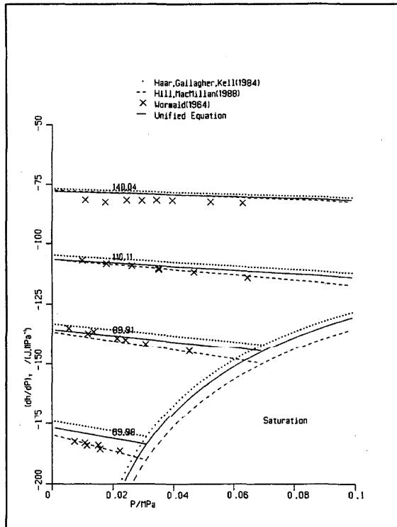
FIG. 118. Isothermal throttling coefficient, vapor: 70–140 °C.
