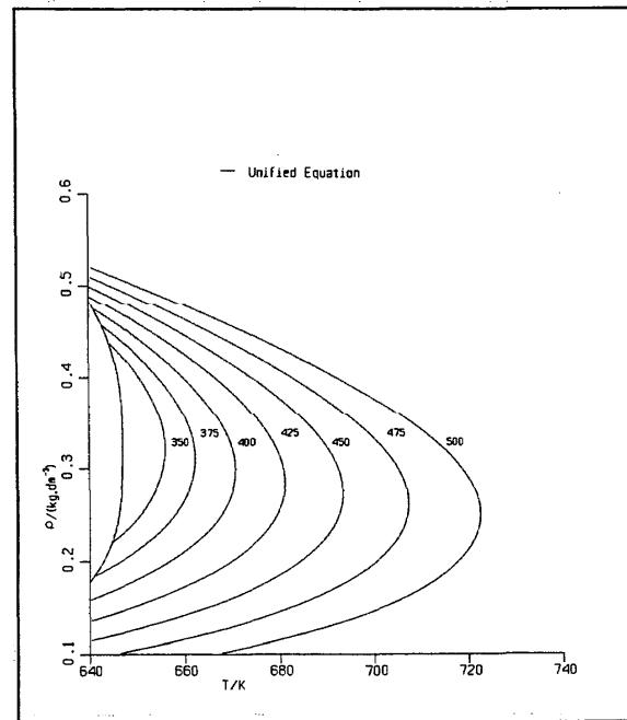
FIG. 131. Speed of sound, critical region.
