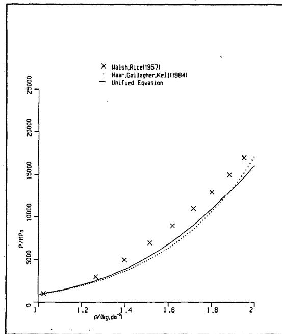
FIG. 87. Ultra high pressure  $500^\circ\text{C}$  ( $773.15\text{ K}$ ).
