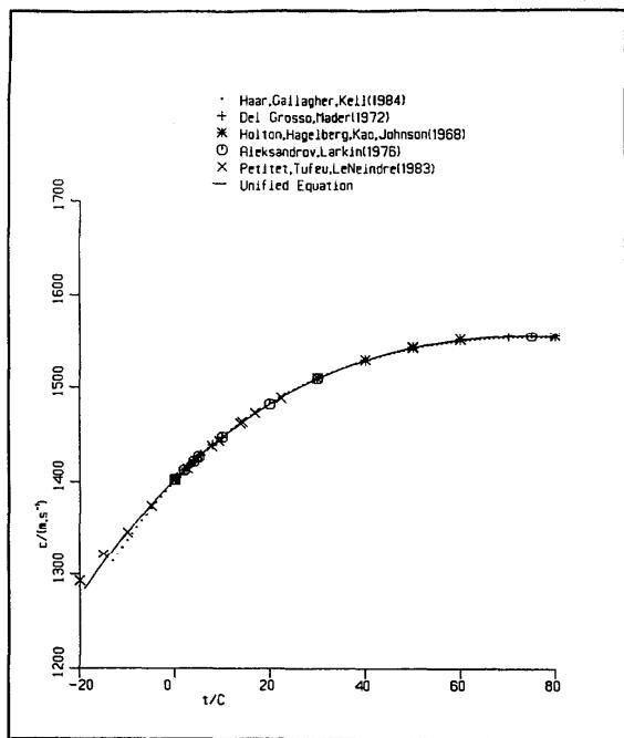
FIG. 94. Speed of sound, supercooled liquid states: 0.1 MPa.
