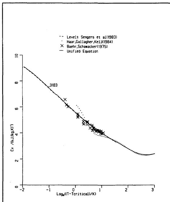
FIG. 113. Isochoric specific heat  $C_v$ : 0.3103  $\text{kg dm}^{-3}$ .
