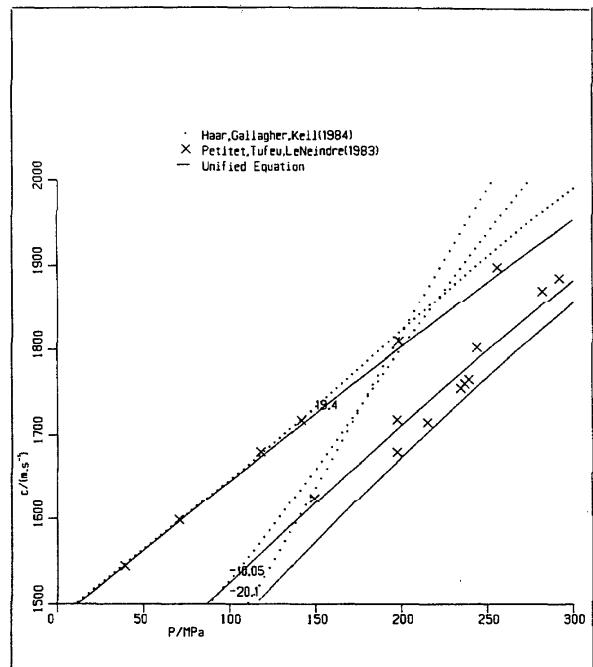
FIG. 96. Speed of sound, supercooled liquid states: -20 to + 20 °C.
