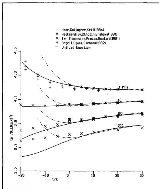
FIG. 106. Isopiestic specific heat  $C_p$ , supercooled liquid: 0.1–400 MPa.
