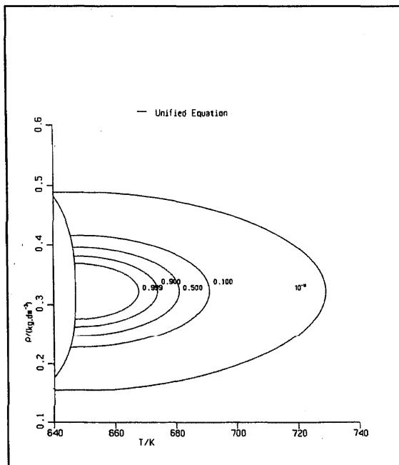
FIG. 126. Blending function  $F$ , critical region.
