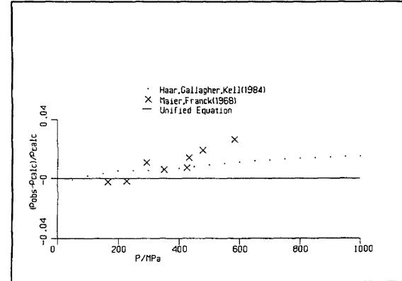
FIG. 71. Density at high pressures: 800 °C.
