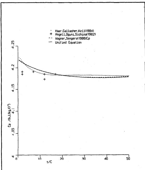
FIG. 103. Isopiestic specific heat  $C_p$ , liquid: 0.1 MPa.
