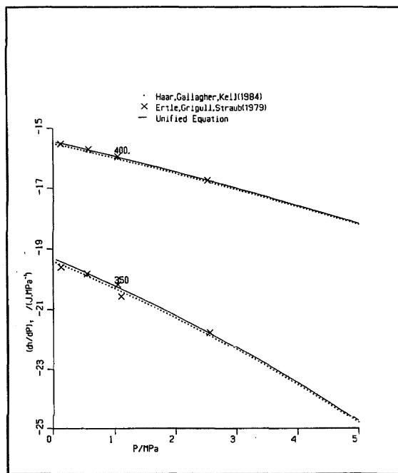
FIG. 119. Isothermal throttling coefficient vapor: 350–400 °C.
