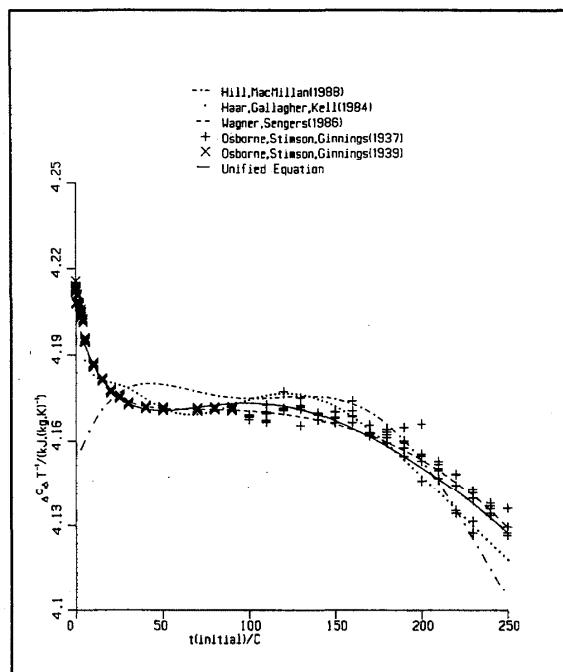
FIG. 22. Saturation function  $\alpha$  0–250 °C.
