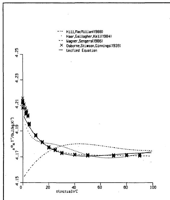
FIG. 21. Saturation function  $\alpha$  0–100 °C.
