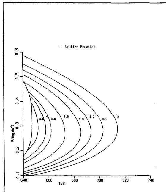
FIG. 127. Isochoric specific heat  $C_v$ , critical region.
