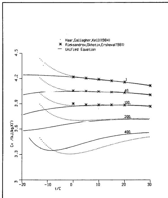
FIG. 115. Isopiestic specific heat  $C_v$ , supercooled 0.1–400 MPa.
