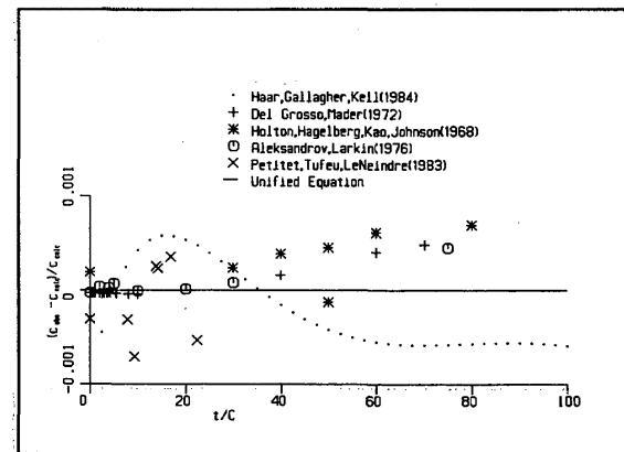
FIG. 92. Speed of sound, liquid: 0.1 MPa.
