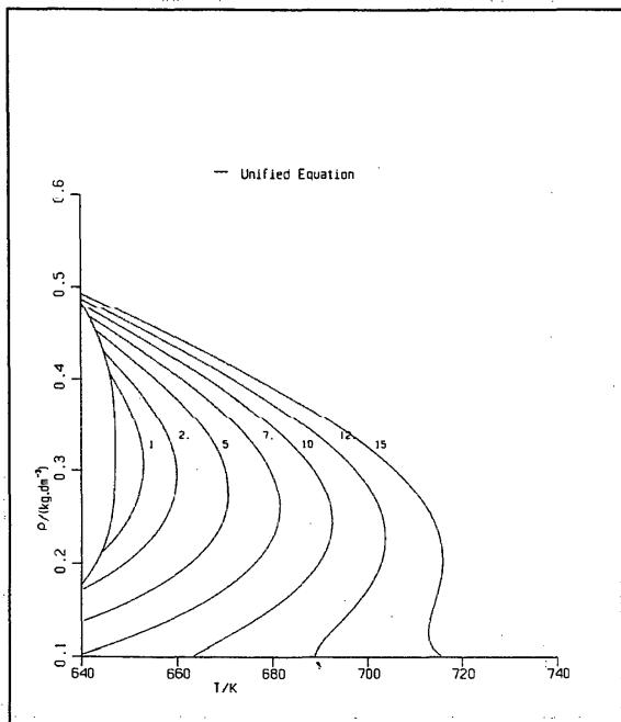
FIG. 129. Inverse isothermal compressibility  $[\rho(\partial P/\partial \rho)]$ , critical region.
