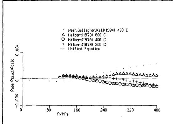
FIG. 68. Density at high pressures: 200–600 °C.
