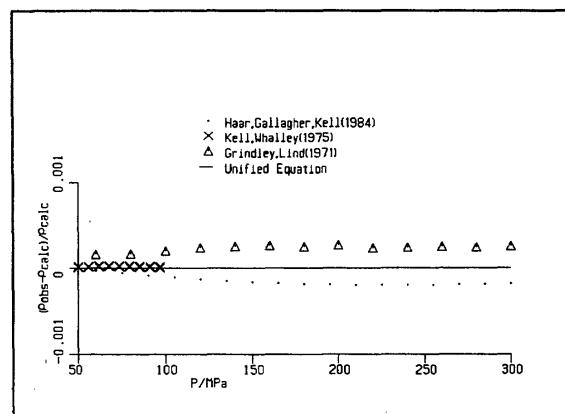
FIG. 64. Liquid density: 150 °C.
