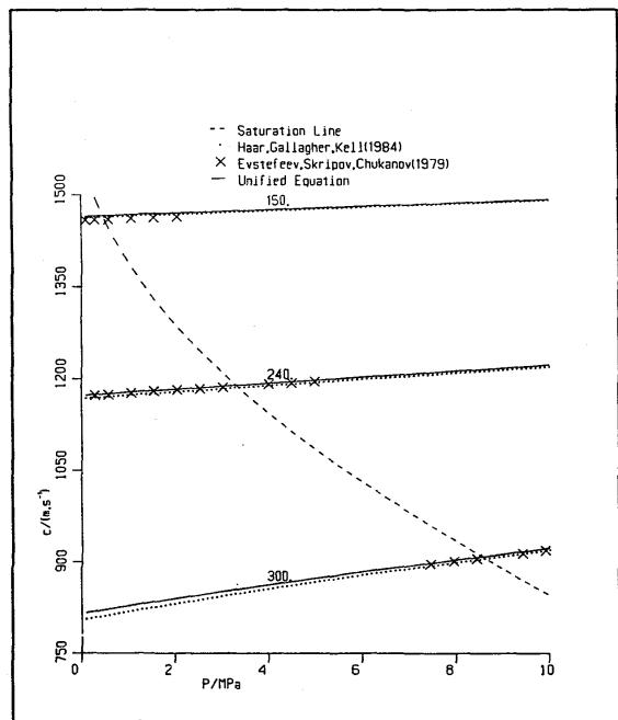
FIG. 101. Speed of sound, metastable liquid states; 150–300 °C.
