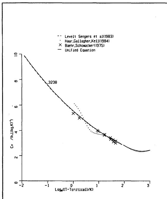
FIG. 112. Isochoric specific heat  $C_v$ : 0.3238  $\text{Kg dm}^{-3}$ .
