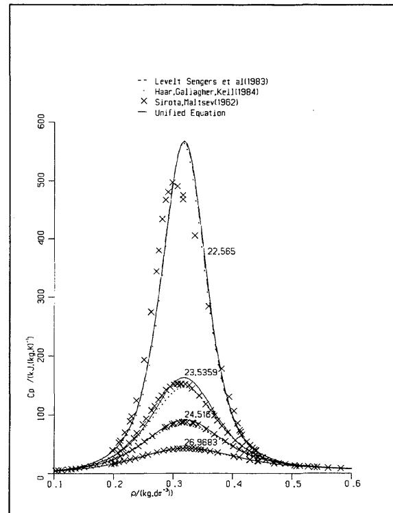
FIG. 110. Isopiestic specific heat  $C_p$ : 22–27 MPa.
