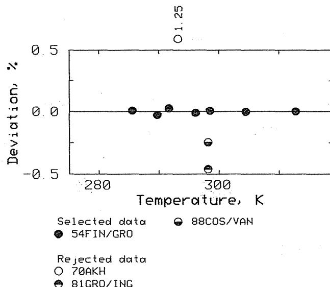
FIG. 15. Deviation plot for pentadecane.
