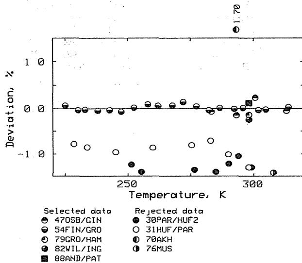
FIG. 9. Deviation plot for nonane.
