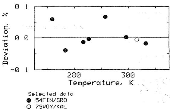
FIG. 13. Deviation plot for tridecane.
