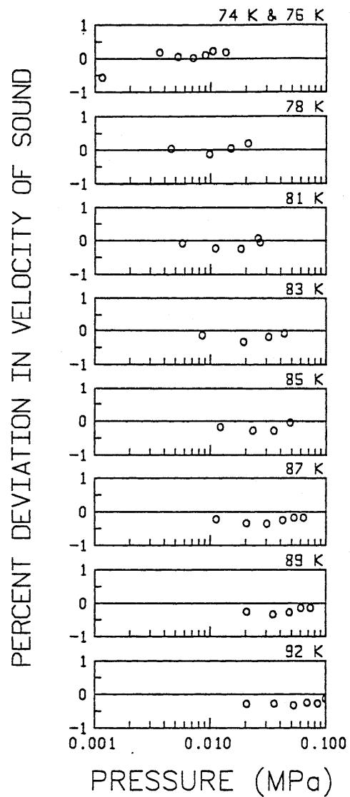
FIG. 13. Comparison of experimental data for the velocity of sound from Van Itterbeek and Van Paeme<sup>47</sup> with calculated values from the fundamental equation
