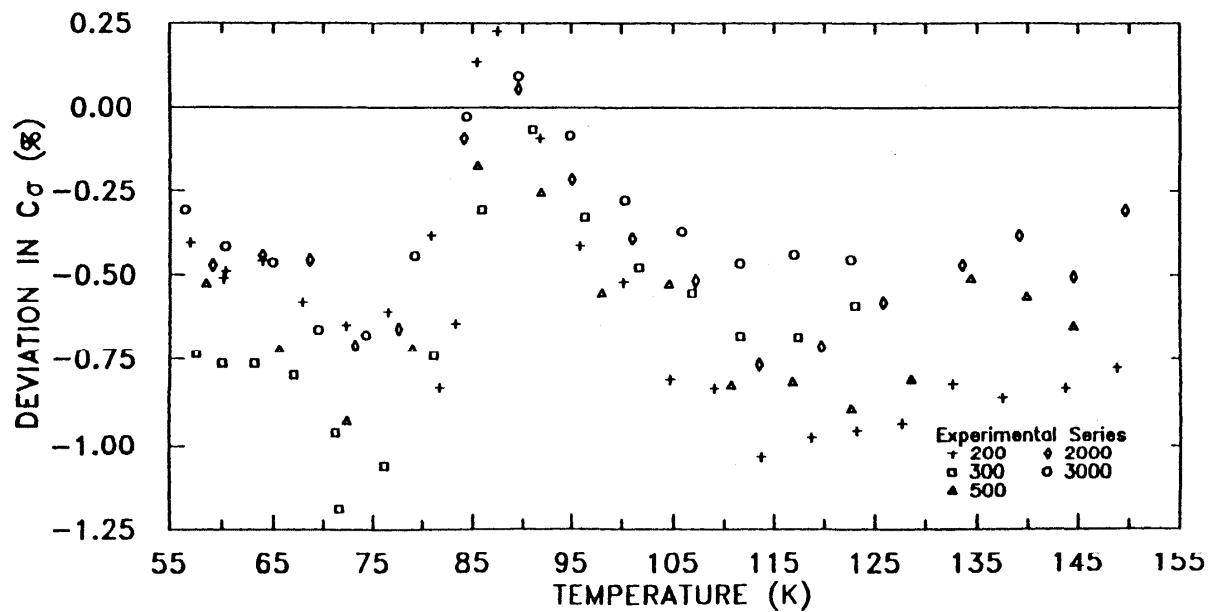
FIG. 11. Comparison of calculated values of the saturated liquid heat capacity ( $C_v$ ) from the fundamental equation to experimental values from Goodwin and Weber<sup>36</sup>.
