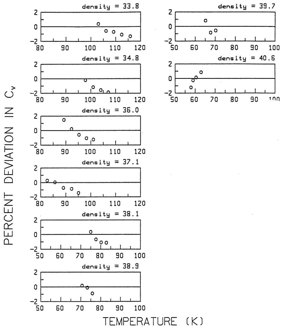
FIG. 10. Comparison of experimental data of the isochoric heat capacity from Goodwin and Weber<sup>37</sup> with values from the fundamental equation. The density given for each graph is in  $\text{mol/dm}^3$  — Continued.
