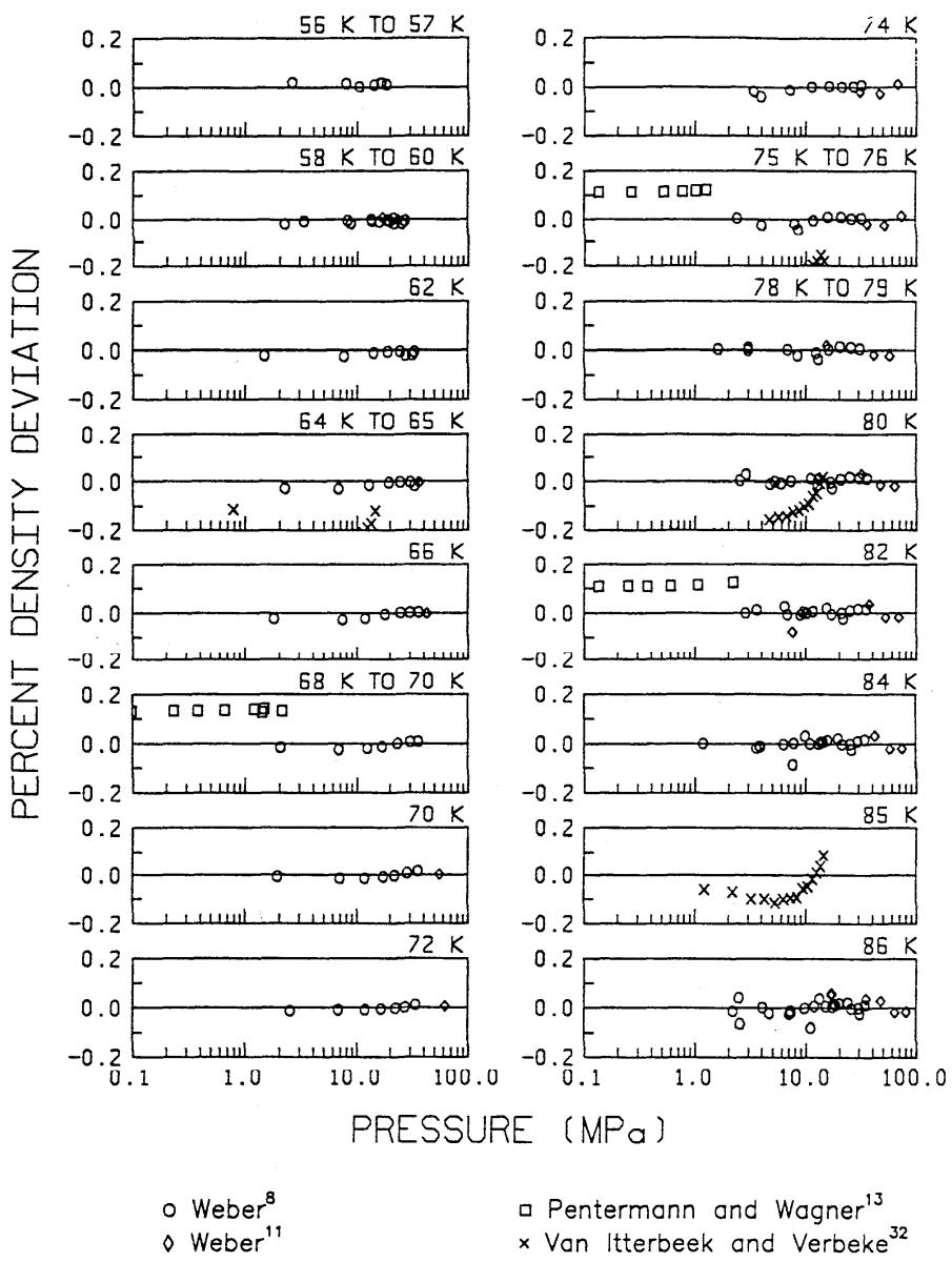
FIG. 6. Comparison of calculated values of density from the fundamental equation to experimental data for liquid states below the critical temperature. The data used in fitting Eq. 15 are  $\circ$  Weber<sup>8</sup>,  $\diamond$  Weber<sup>11</sup>, and  $\square$  Pentermann and Wagner<sup>13</sup>.
