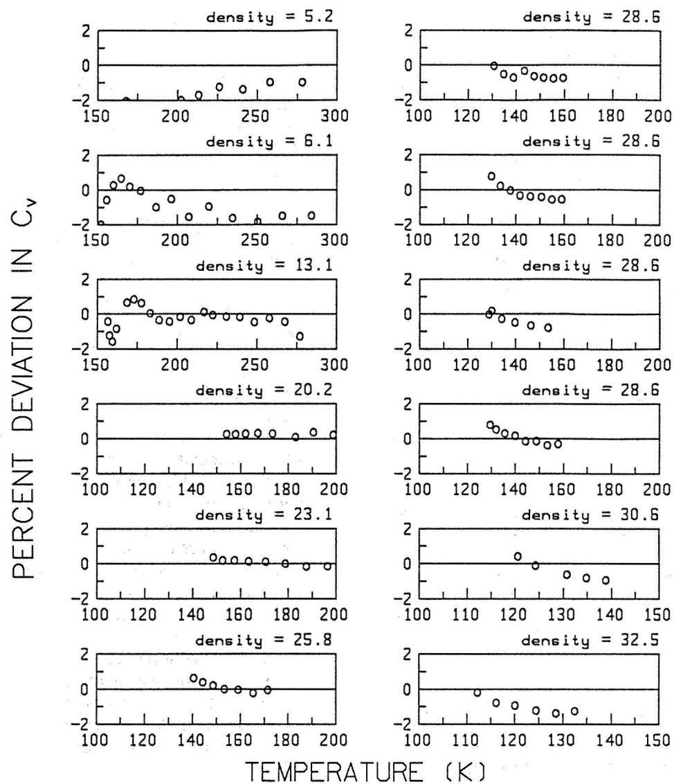
FIG. 10. Comparison of experimental data of the isochoric heat capacity from Goodwin and Weber<sup>37</sup> with values from the fundamental equation. The density given for each graph is in mol/dm<sup>3</sup>.
