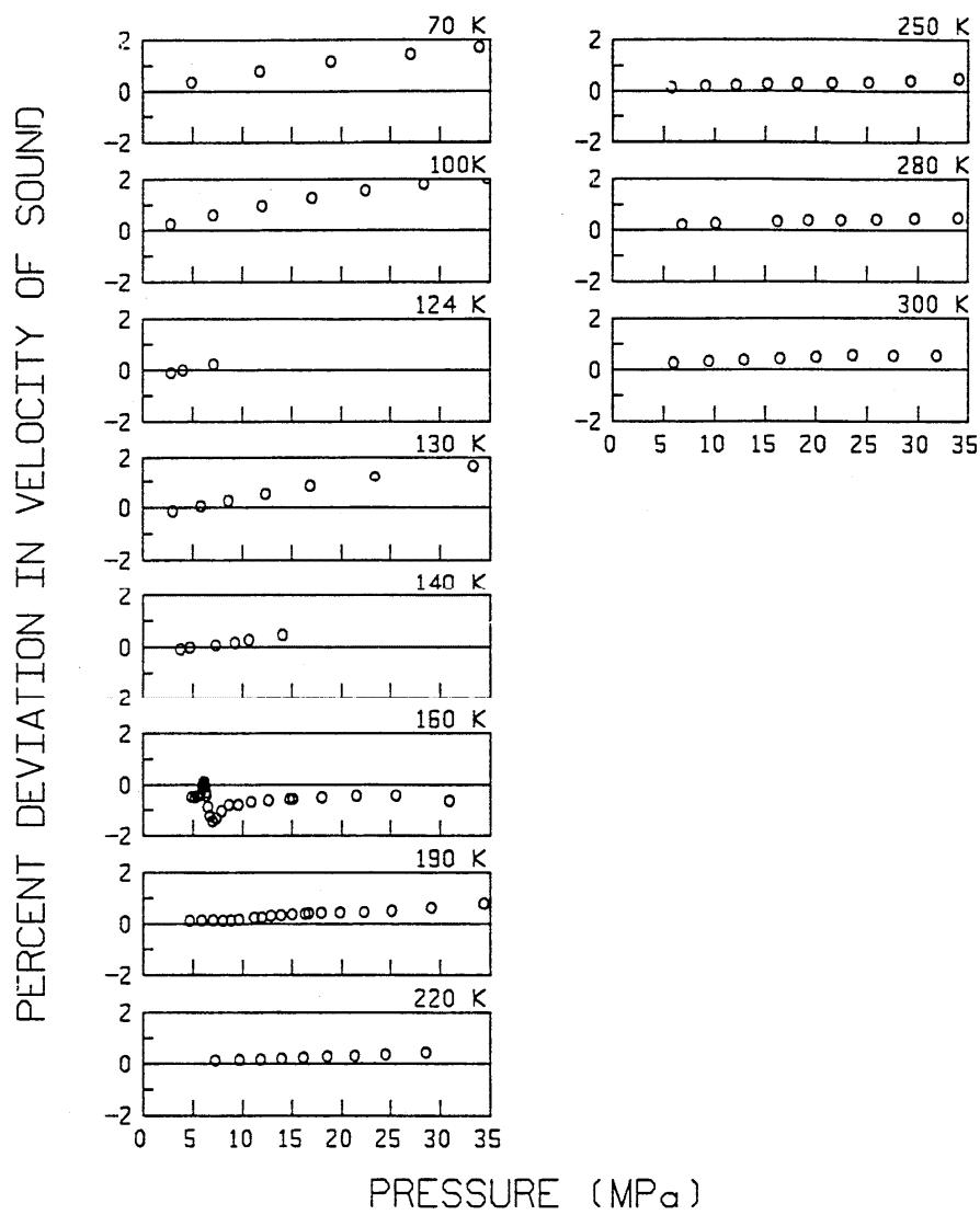
FIG. 12. Comparison of experimental data for the velocity of sound from Straty and Younglove<sup>42</sup> with calculated values from the fundamental equation.
