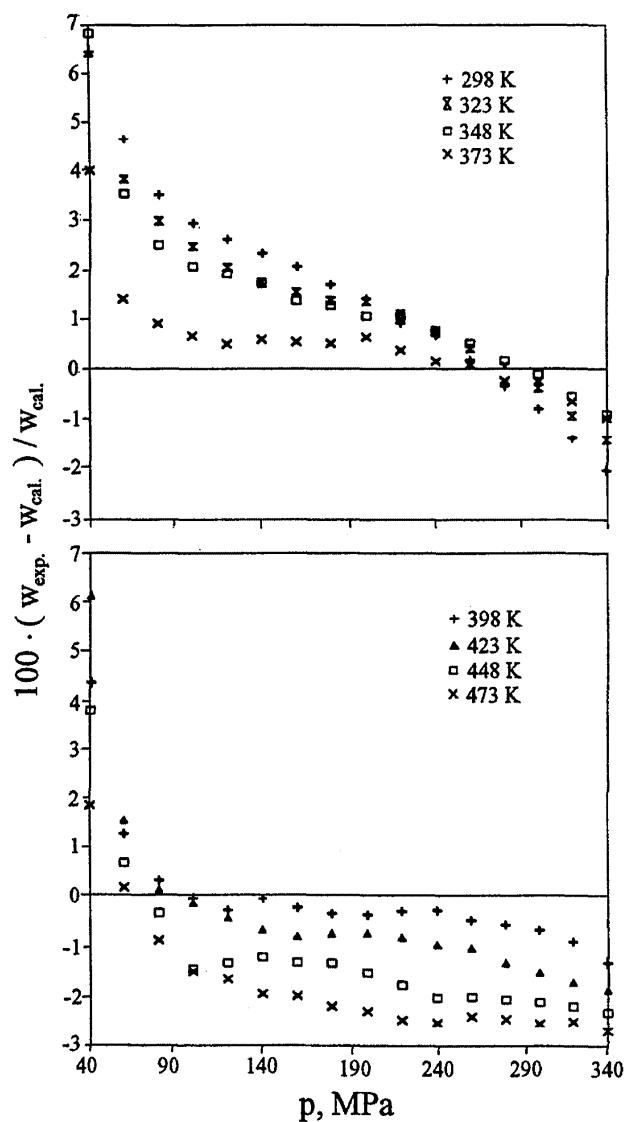
FIG. 11. Comparison of smoothed speed of sound data by Pitajevskaja *et al.*<sup>67</sup> with Eq. (3).
