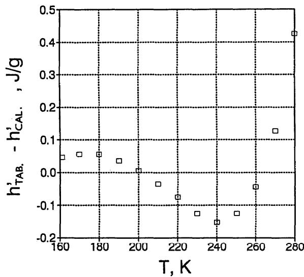
FIG. 14. Comparison of enthalpies along the saturation curve from Tables by Rabinovich<sup>5</sup> with calculated from Eq. (3).
