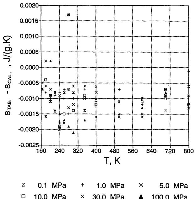
FIG. 18. Comparison of entropies along selected isobars from Tables by Rabinovich<sup>5</sup> with calculated from Eq. (3).
