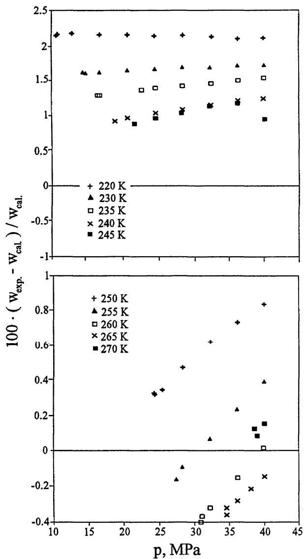
FIG. 12. Comparison of measured speed of sound data by Baidakov *et al.*<sup>68</sup> with Eq. (3).
