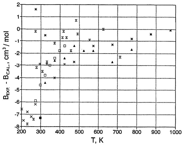
FIG. 4. Deviations of experimental and calculated values of the second virial coefficient.
