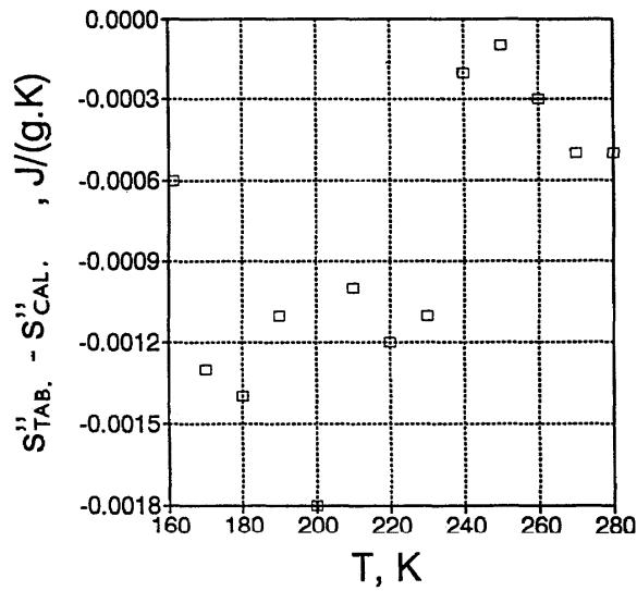
FIG. 15. Comparison of entropies along the saturation curve from Tables by Rabinovich<sup>5</sup> with calculated from Eq. (3).
