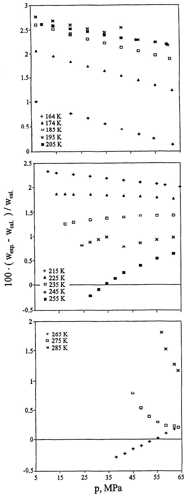
FIG. 10. Comparison of measured speed of sound by Lim *et al.*<sup>66</sup> with Eq. (3).
