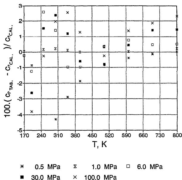
FIG. 17. Comparison of isobaric heat capacities along selected isobars from Tables by Rabinovich<sup>5</sup> with calculated from Eq. (3).
