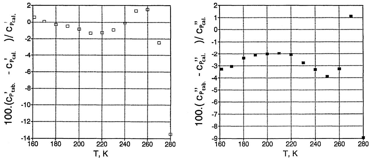
FIG. 13. Comparison of isobaric heat capacities along the saturation curve from Tables by Rabinovich<sup>5</sup> with calculated from Eq. (3).
