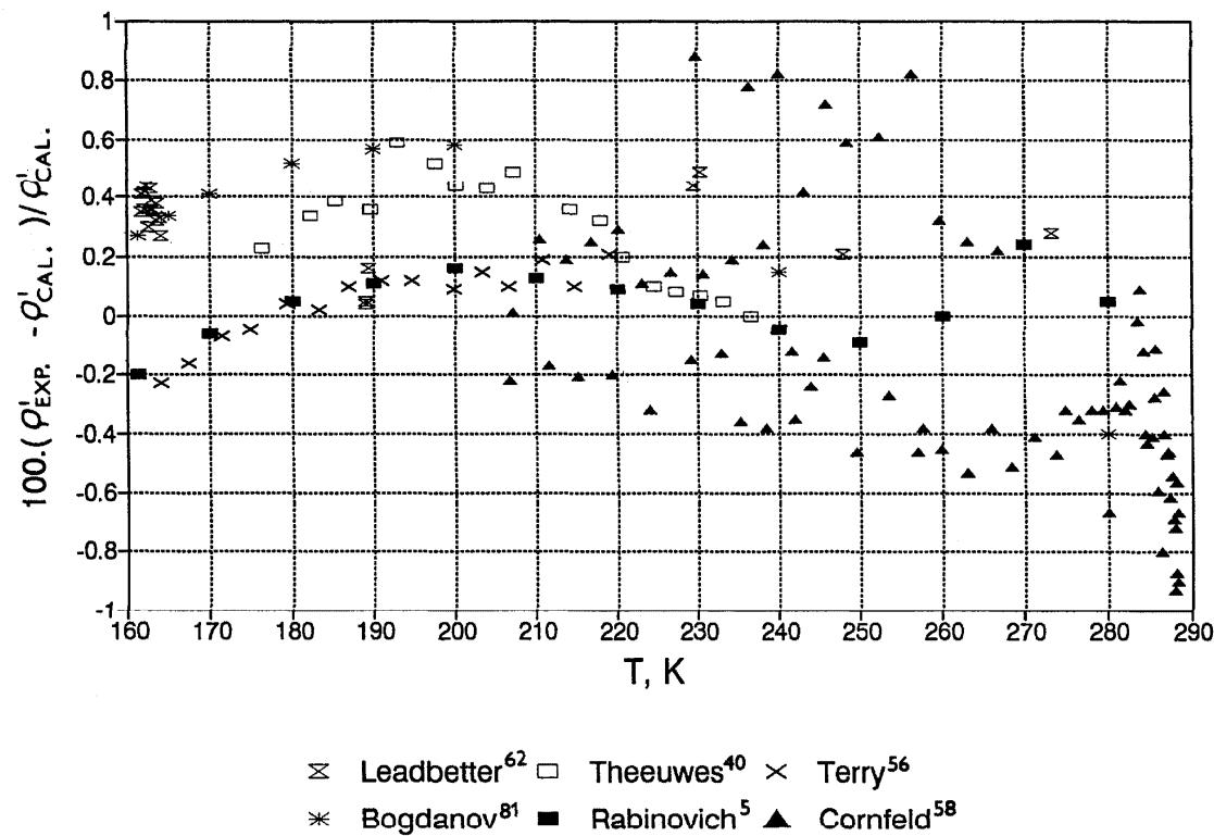
FIG. 7. Comparison of experimental saturated liquid densities with Eq. (3).
