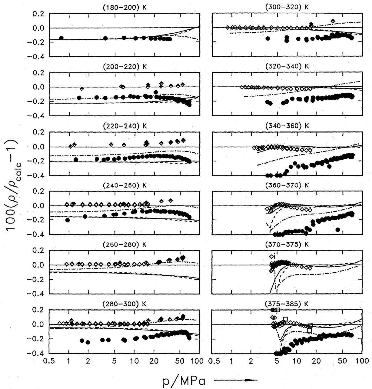
FIG. 6. Density deviations of  $(p,\rho,T)$ -properties in the liquid phase from our own EOS.  $\square$ : Tillner-Roth and Baehr<sup>54</sup>,  $\diamond$ : Tillner-Roth and Baehr<sup>55</sup>,  $\blacklozenge$ : Klomfar et al.<sup>28</sup>,  $\bullet$ : Hou et al.<sup>23</sup>, — HM-EOS, - - HE-EOS, - · - PNSW-EOS.
