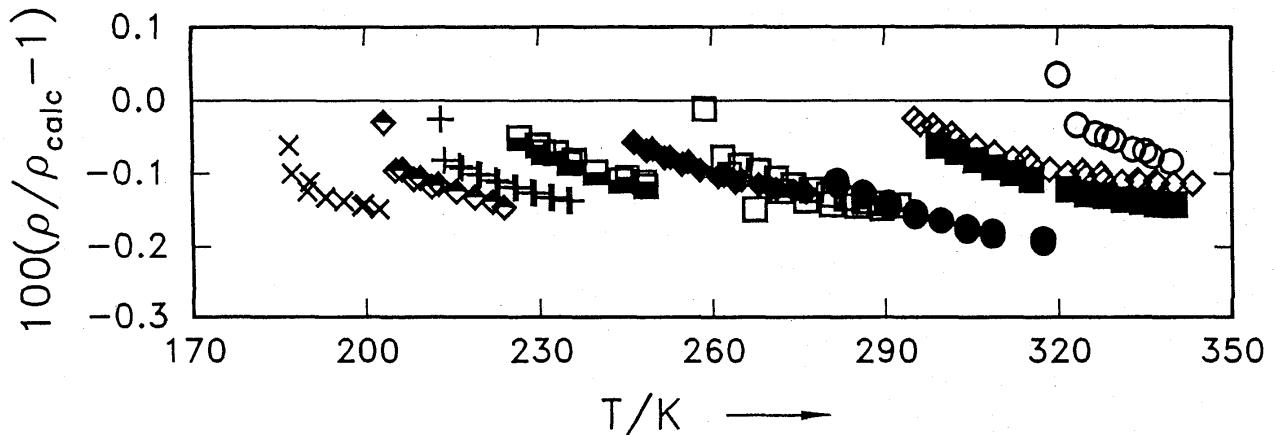
FIG. 14. Density deviations of  $(p, \rho, T)$ -properties reported by Magee<sup>33</sup> from our own EOS. ○: 1130 kg/m<sup>3</sup>, ■: 1215 kg/m<sup>3</sup>, ◇: 1225 kg/m<sup>3</sup>, ●: 1280 kg/m<sup>3</sup>, □: 1345 kg/m<sup>3</sup>, ♦: 1385 kg/m<sup>3</sup>, +: 1475 kg/m<sup>3</sup>, ×: 1500 kg/m<sup>3</sup>.
