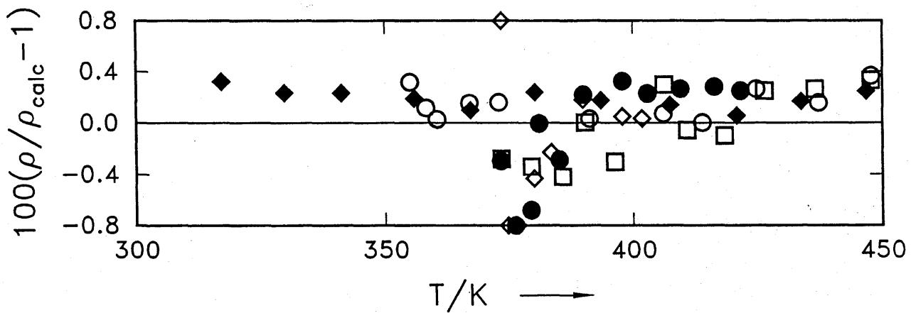
FIG. 9. Density deviations of  $(p, \rho, T)$ -properties reported by Basu and Wilson<sup>5</sup> from our own EOS. ♦: 51 kg/m<sup>3</sup>, ○: 156 kg/m<sup>3</sup>, □: 261 kg/m<sup>3</sup>, ●: 361 kg/m<sup>3</sup>, ◇: 520 kg/m<sup>3</sup>.
