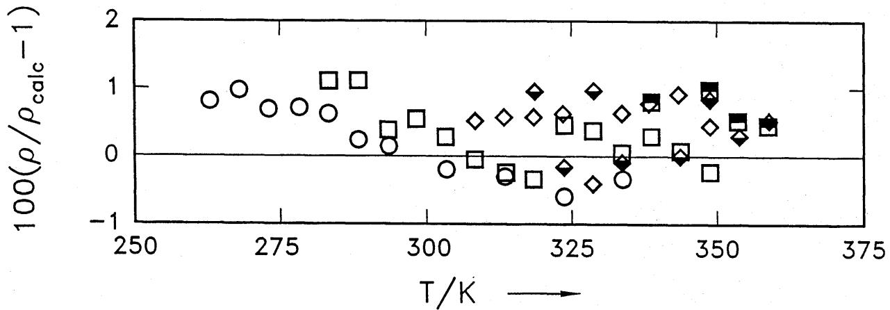
FIG. 8. Density deviations of  $(p, \rho, T)$ -properties reported by Baroncini *et al.*<sup>4</sup> from our own EOS. ○: 9 kg/m<sup>3</sup>, □: 20 kg/m<sup>3</sup>, ◇: 40 kg/m<sup>3</sup>, ♦: 56 kg/m<sup>3</sup>, ■: 88 kg/m<sup>3</sup>.
