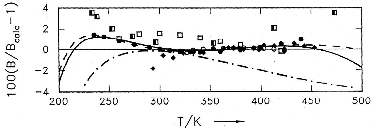
FIG. 20. Deviations of second virial coefficients from the EOS. ♦: Tillner-Roth and Baehr<sup>54</sup>, ○: Dressner and Bier<sup>12</sup>, ●: Goodwin and Moldover<sup>18</sup>, □: Beckermann and Kohler<sup>6</sup>, ■: Schramm *et al.*<sup>50,49</sup>, —: HM-EOS, - - -: HE-EOS, - · - : PNSW-EOS.
