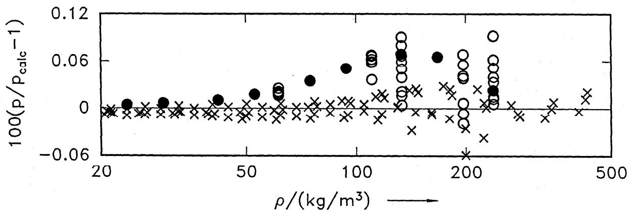
FIG. 18. Pressure deviations of  $(p, \rho, T)$ -properties between 350 K and 400 K from our own EOS. ●: Weber (Burnett-measurements)<sup>58</sup>, ○: Weber (isochoric measurements)<sup>58</sup>, ×: Tillner-Roth and Baehr<sup>54</sup>.
