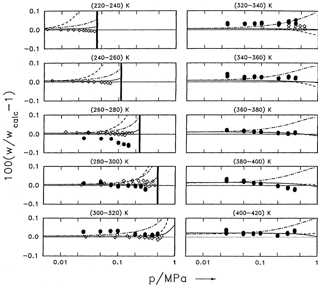
FIG. 23. Deviations of speed of sound values in the gaseous phase from our own EOS.  $\diamond$ : Goodwin and Moldover<sup>18</sup>,  $\bullet$ : Beckermann and Kohler<sup>6</sup>,  $\blacksquare$ : saturation boundary, —: HM-EOS, - - -: HE-EOS, - · - -: PNSW-EOS.
