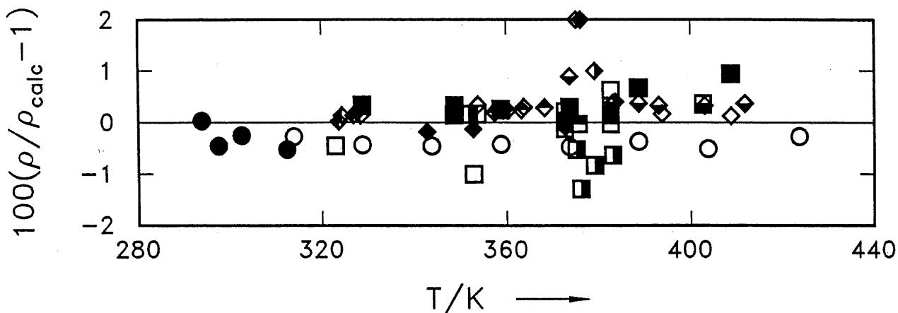
FIG. 11. Density deviations of  $(p,\rho,T)$ -properties reported by Fukushima *et al.*<sup>15</sup> from our own EOS. O:  $23 \text{ kg/m}^3$ , ●:  $28 \text{ kg/m}^3$ , □:  $51 \text{ kg/m}^3$ , ■:  $75 \text{ kg/m}^3$ , ◆:  $109 \text{ kg/m}^3$ , ◇:  $152 \text{ kg/m}^3$ , ◇:  $218 \text{ kg/m}^3$ , ◇:  $313 \text{ kg/m}^3$ , □:  $501 \text{ kg/m}^3$ , ◆:  $548 \text{ kg/m}^3$ , □:  $700 \text{ kg/m}^3$ , ◆:  $897 \text{ kg/m}^3$ , ■:  $968 \text{ kg/m}^3$ , ◆:  $1100 \text{ kg/m}^3$ .
