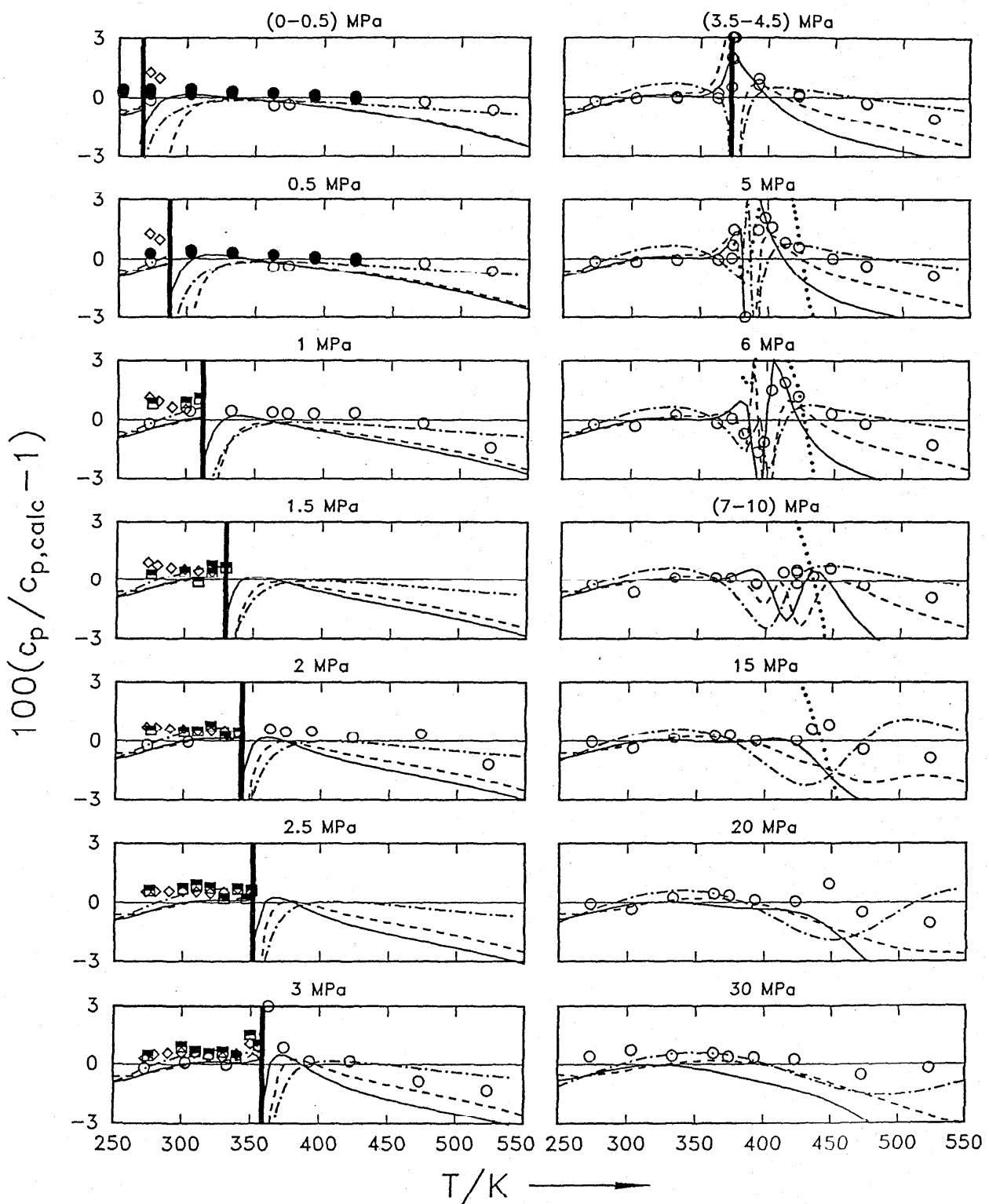
FIG. 22. Deviations of isobaric heat capacities from values calculated from our own EOS.  $\diamond$ : Saitoh *et al.*<sup>46</sup>,  $\square$ : Nakagawa *et al.*<sup>19</sup>,  $\bullet$ : Gürtner and Ernst<sup>20</sup>,  $\circ$ : Wirbser<sup>59</sup>,  $\blacksquare$ : saturation boundary, — HM-EOS, --- HE-EOS, - - - PNSW-EOS, ..... Tang *et al.*<sup>51</sup>.
