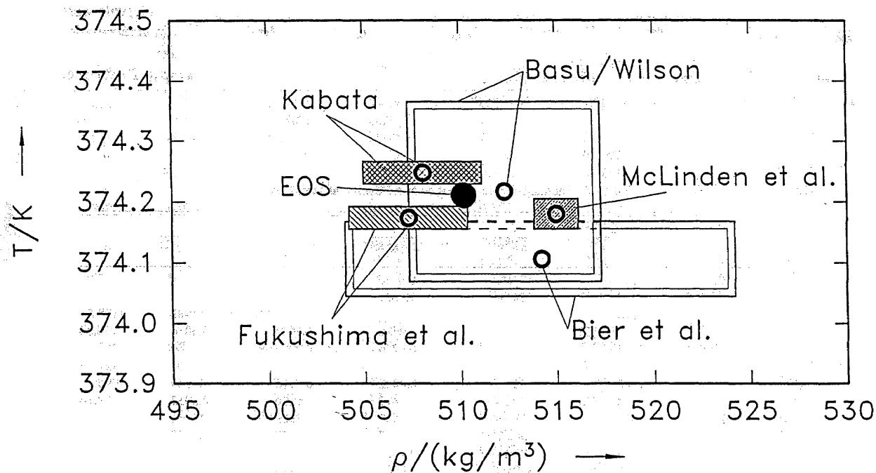
FIG. 32. Comparison of measured critical parameters  $T_c$  and  $p_c$  with values calculated from our own EOS. The rectangles indicate the uncertainty of the respective experimental value.
