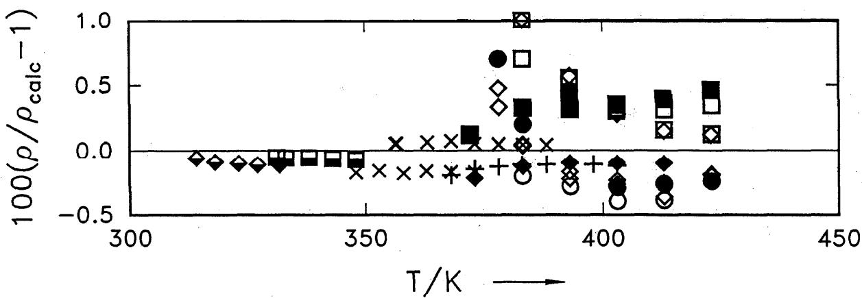
FIG. 16b. Density deviations of  $(p, \rho, T)$ -properties reported by Piao *et al.*<sup>43</sup> from our own EOS. ○: 483 kg/m<sup>3</sup>, □: 495 kg/m<sup>3</sup>, ◇: 508 kg/m<sup>3</sup>, ●: 590 kg/m<sup>3</sup>, ■: 691 kg/m<sup>3</sup>, ◆: 780 kg/m<sup>3</sup>, +: 839 kg/m<sup>3</sup>, ×: 903 kg/m<sup>3</sup>, ■: 1064 kg/m<sup>3</sup>, ♦: 1143 kg/m<sup>3</sup>.
