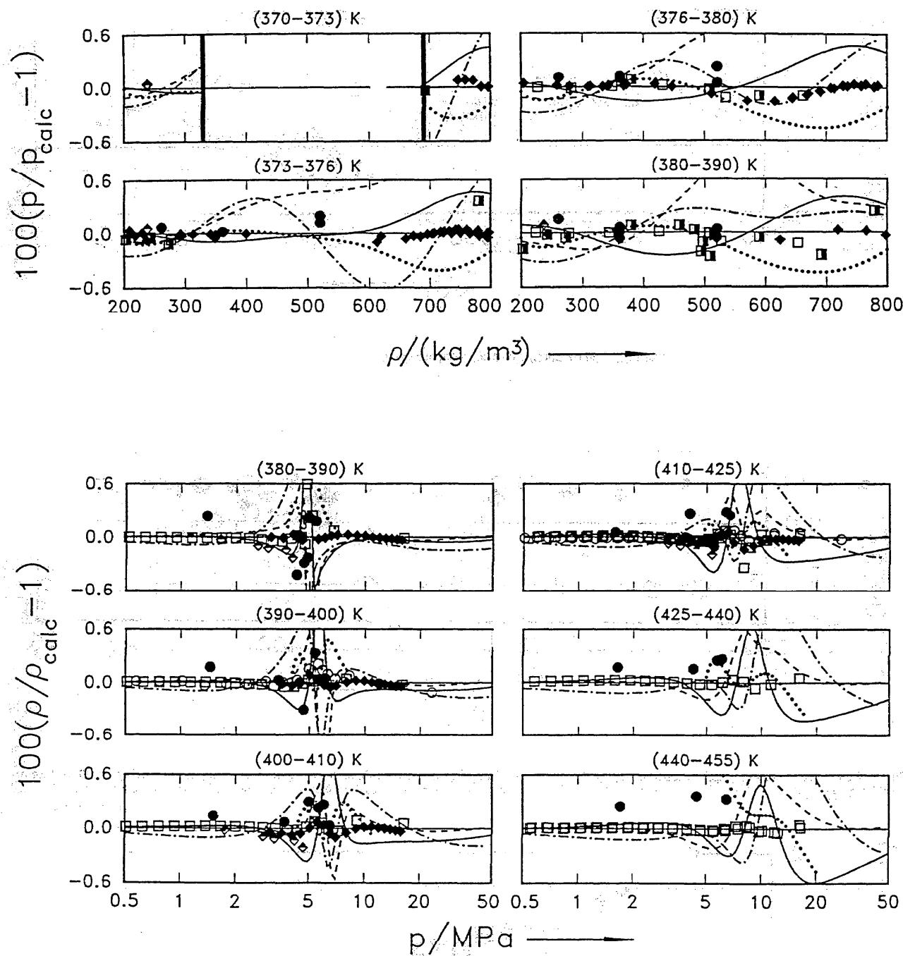
FIG. 7. Pressure and density deviations of  $(p, \rho, T)$ -properties in near-critical and supercritical states from our own EOS. □: Tillner-Roth and Baehr<sup>54</sup>, ▽: Tillner-Roth and Baehr<sup>55</sup>, ●: Basu and Wilson<sup>5</sup>, ○: Dressner and Bier<sup>12</sup>, ■: Piao *et al.*<sup>43</sup>, ◇: Weber<sup>58</sup>, I: Saturation, —: HM-EOS, - - -: HE-EOS, - · - -: PNSW-EOS, · · · · : Tang *et al.*<sup>53</sup>.
