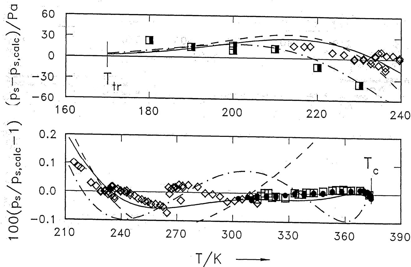
FIG. 26. Deviations of selected vapor pressures from the fundamental equation of state. □: Magee and Howley<sup>34</sup>, ◇: Goodwin *et al.*<sup>17</sup>, ●: Baehr and Tillner-Roth<sup>11</sup>, ▨: Weber<sup>58</sup>, —: HM-EOS, - - -: HE-EOS, - · - -: PNSW-EOS.
