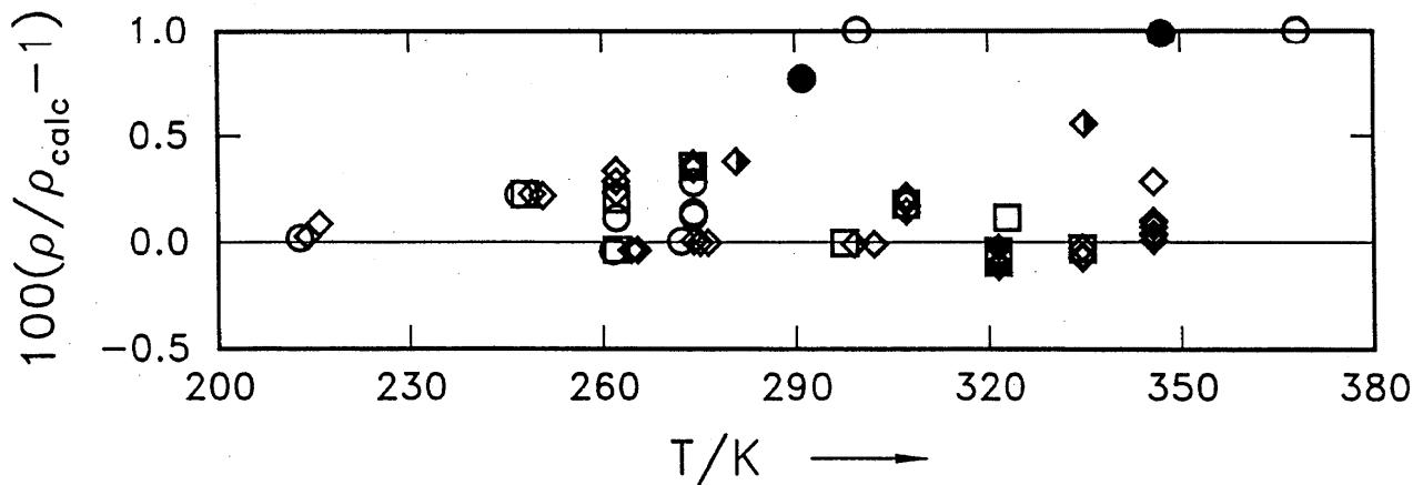
FIG. 12. Density deviations of  $(p,\rho,T)$ -properties reported by Kesselman *et al.*<sup>27</sup> from our own EOS. O: <1 MPa, □: 1-2 MPa, ◇: 2-5 MPa, ◆: 5-10 MPa, ●: 10-20 MPa.
