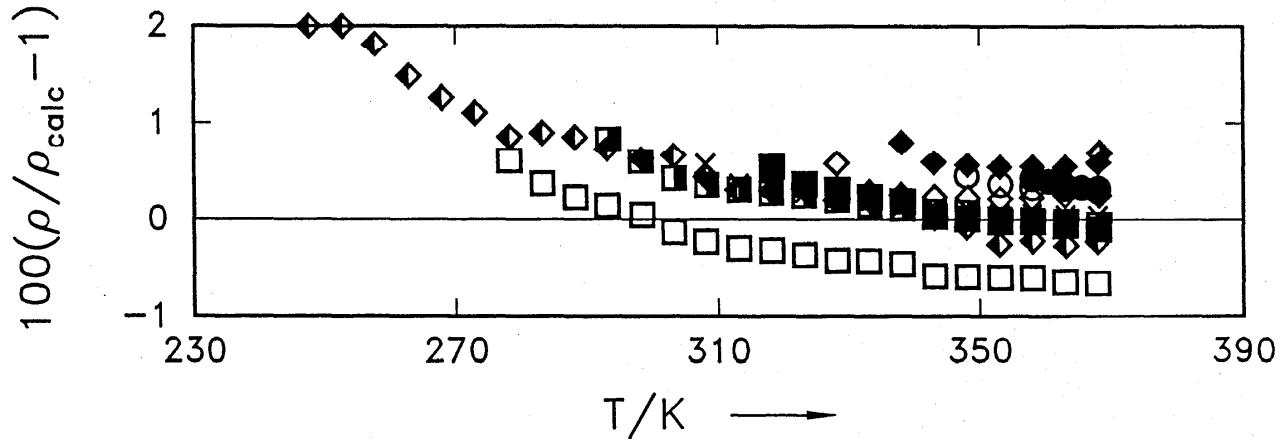
FIG. 10. Density deviations of  $(p, \rho, T)$ -properties reported by Doering<sup>11</sup> from our own EOS. ♦: 3.75 kg/m<sup>3</sup>, □: 12.8 kg/m<sup>3</sup>, ■: 24.5 kg/m<sup>3</sup>, ×: 35 kg/m<sup>3</sup>, ●: 51 kg/m<sup>3</sup>, ◇: 72 kg/m<sup>3</sup>, ♦: 93.5 kg/m<sup>3</sup>, ○: 114 kg/m<sup>3</sup>, ●: 156 kg/m<sup>3</sup>, ♦: 232 kg/m<sup>3</sup>.
