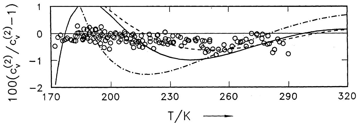
FIG. 31. Deviations of two-phase isochoric heat capacities measured by Magee<sup>33</sup> from our own EOS. The other equations of state were evaluated at  $1100 \text{ kg/m}^3$  which is about in the middle of the density range covered by the experiments. — HM-EOS, - - - HE-EOS, - · - PNSW-EOS.
