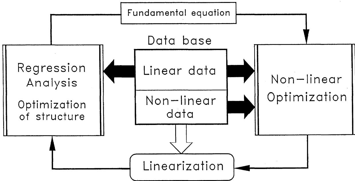
FIG. 4. Optimization cycle during the formulation of the residual part  $\Phi'$  of the fundamental equation.
