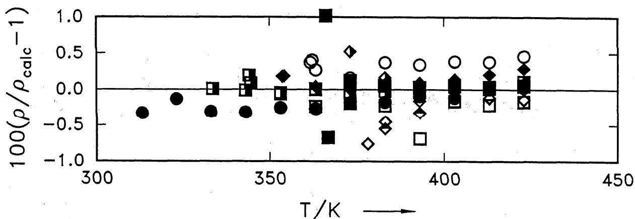
FIG. 16a. Density deviations of  $(p, \rho, T)$ -properties reported by Piao *et al.*<sup>43</sup> from our own EOS. ●: 37 kg/m<sup>3</sup>, ■: 87 kg/m<sup>3</sup>, □: 151 kg/m<sup>3</sup>, ◆: 155 kg/m<sup>3</sup>, ○: 203 kg/m<sup>3</sup>, ■: 242 kg/m<sup>3</sup>, ♦: 273 kg/m<sup>3</sup>, ◇: 380 kg/m<sup>3</sup>, ♦: 459 kg/m<sup>3</sup>.
