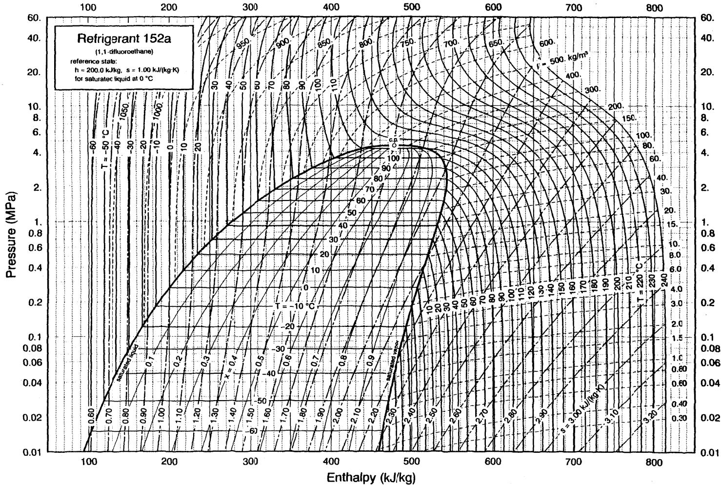
FIG. 13. Pressure-enthalpy diagram for R-152a.
