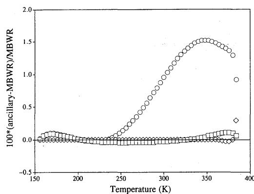
FIG. 4. Deviations of saturation properties calculated with the ancillary equations from saturation properties calculated with the MBWR equation. Saturated vapor densities ( $\circ$ ), vapor pressures ( $\square$ ), and saturated liquid densities ( $\diamond$ ).
