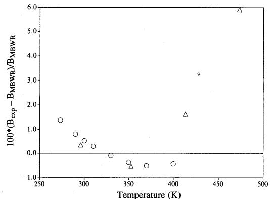
FIG. 6. Deviations of experimental second virial coefficients used in the MBWR correlation from values calculated with the MBWR equation. Data of Gillis<sup>12</sup> (○), and Schramm<sup>36</sup> (△).
