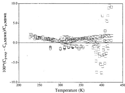
FIG. 8. Deviations of experimental isobaric heat capacities from values calculated with the MBWR equation. Data of Porichanski<sup>22</sup> (□), and Nakagawa<sup>23</sup> (○).
