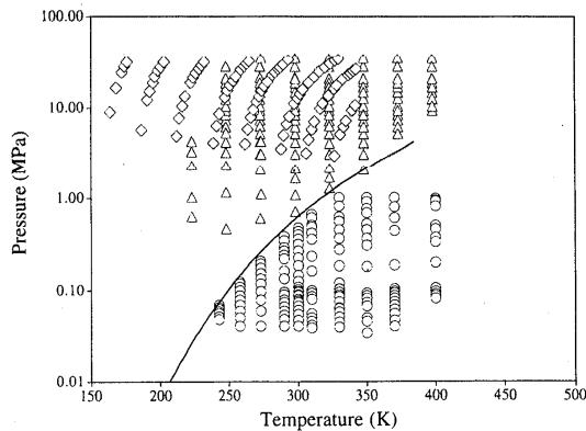
FIG. 2. Experimental isochoric heat capacity and speed of sound data used in MBWR correlation. Speed of sound data of Ahn<sup>24</sup> (Δ), and Gillis<sup>12</sup> (○), and heat capacity data of Magee<sup>7</sup> (◇).
