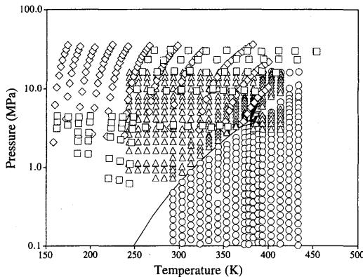
FIG. 1. Experimental PVT data used in the MBWR correlation. Blanke<sup>5</sup> (□), Magee<sup>10</sup> (◊), Tillner-Roth<sup>11</sup> (○), Tillner-Roth<sup>21</sup> (△), and the saturation line (—).
