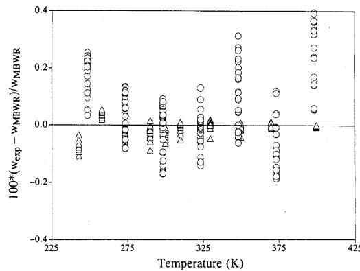
FIG. 9. Deviations of experimental speed of sound used in the MBWR correlation from values calculated with the MBWR equation. Data of Gillis<sup>12</sup> (△), and Ahn<sup>24</sup> (○).
