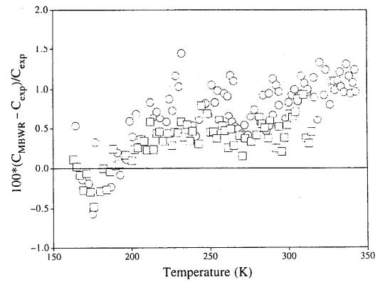
FIG. 7. Deviations of experimental saturated and isochoric heat capacities used in the MBWR correlation from values calculated with the MBWR equation.  $C_s$  data of Magee<sup>7</sup> (□), and  $C_v$  data of Magee<sup>7</sup> (1995) (○).
