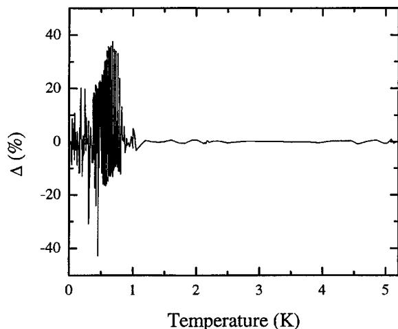
FIG. 10.2. Deviation of the database from the spline fit to  $\log_{10} \mu_+$ . (Note: The large deviations at low temperatures reflect a divergence in magnitudes reported in Refs. 14 and 18.)
