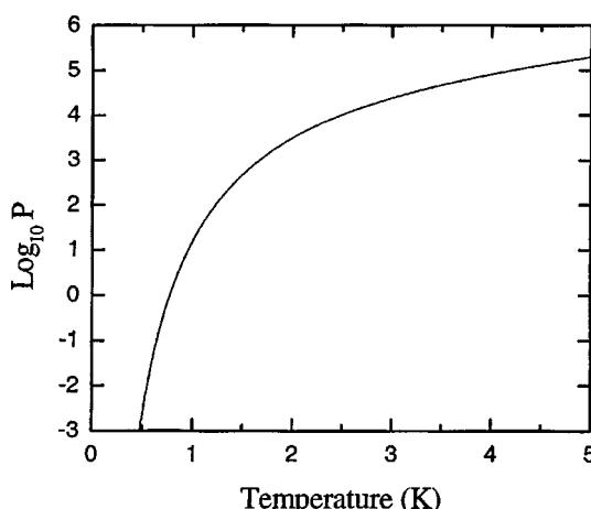
FIG. 17.2.  $\log_{10}$  of the saturated vapor pressure curve (in Pa) of liquid  $^4\text{He}$ .
