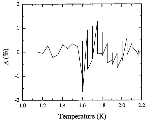
FIG. 8.4. The fractional deviation of values of the adopted database from the recommended values for the entropy integrated from the heat capacity spline.
