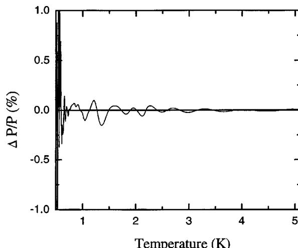
FIG. 17.3. The fractional deviation of values of the saturated vapor pressure of  $^4\text{He}$  calculated with the spline from those calculated with the ITS-90 equations expressed as percent.
