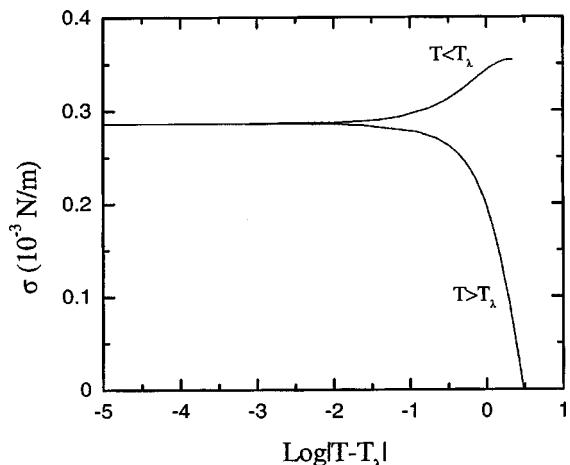
FIG. 9.2. Detail of the surface tension about the lambda transition.
