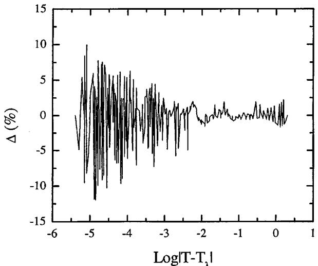
FIG. 15.3. Deviation of the database from the spline fit of thermal conductivity expressed in percent.
