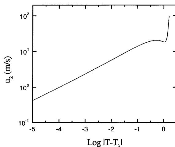
FIG. 4.2. Detail of the recommended values for the second sound velocity in helium II about the lambda transition.
