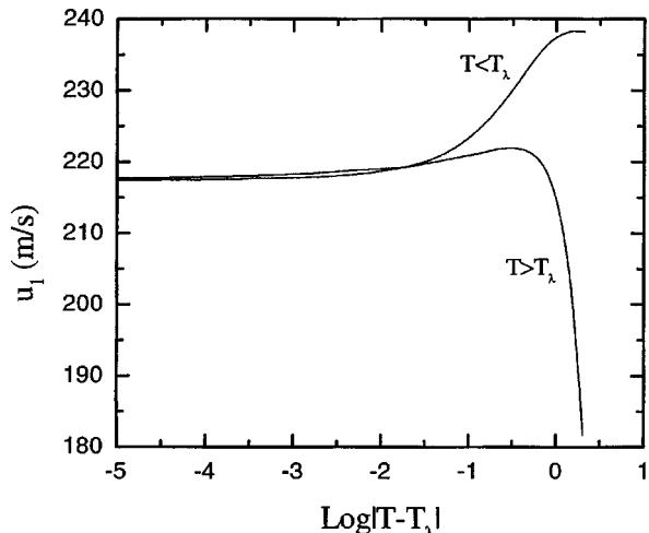
FIG. 3.2. Detail of the recommended values for the first sound velocity of liquid  $^4\text{He}$  about the lambda transition.
