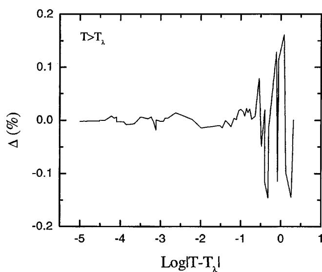
FIG. 3.5. The fractional deviation of the adopted database from the recommended values of the velocity of first sound in liquid  $^4\text{He}$  expressed in percent for  $T > T_\lambda$ .TABLE 3.3. Recommended values of first sound velocity in liquid  $^4\text{He}$
