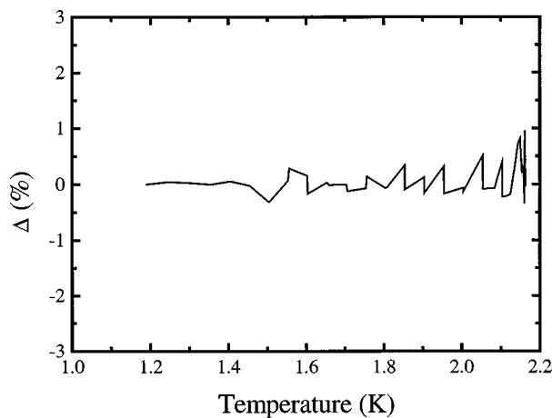
FIG. 6.2. The fractional deviation of values of the adopted database from the recommended values for the velocity of fourth sound in helium II expressed in percent.
