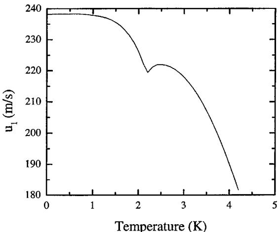
FIG. 3.1. The recommended values for the first sound velocity of liquid  $^4\text{He}$  as a function of temperature at saturated vapor pressure.
