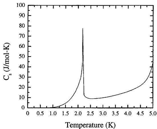
FIG. 7.1. The recommended values for the heat capacity of liquid <sup>4</sup>He as a function of temperature at saturated vapor pressure.
