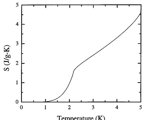
FIG. 8.3. The recommended values of the entropy of liquid  ${}^4\text{He}$  obtained by integration of the heat capacity spline.
