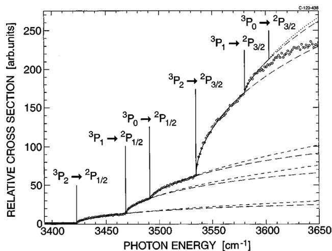
Fig. 1. Photodetachment yield vs photon energy for the  $\text{Al}^-$  ion [SBT98]. The measurements are performed by tunable infrared spectroscopy. The data are analyzed using a Wigner  $s$ -wave fit including the leading correction term (solid line). For the first three thresholds the difference between the dotted lines represents the contribution from the correction term. Thus, the two lines define the upper and lower limits for the  $s$ -wave thresholds.
