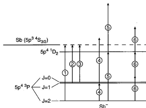
Fig. 4. Schematic energy level diagram of  $\text{Sb}^-$ . Arrows indicate different photodetachment schemes: (1–3) single photon detachment thresholds; (4–5) two-photon detachment via single-photon  $M1$  resonance; (6) three-photon detachment via two-photon E1 resonance [SHB97].
