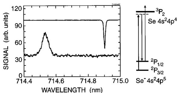
FIG. 5. Raman photodetachment of  $\text{Se}^-(^2P_{3/2})$  ions [TSS96a]. An illustration of the (2+1) Raman detachment scheme is shown on the right side. The neutral Se atom signal vs the wavelength of the "red" laser is shown in the lower trace, while the wavelength of the "blue" laser is fixed at 614.476 nm. The opticalgalvanic calibration signal is shown in the upper trace.
